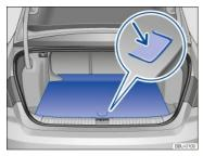
Fig. 127 In the luggage compartment: opening the luggage compartment floor.
