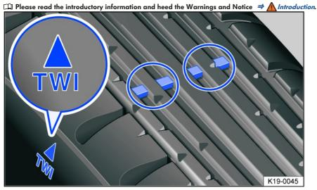
Fig. 163 Tire tread: tread wear indicator.
