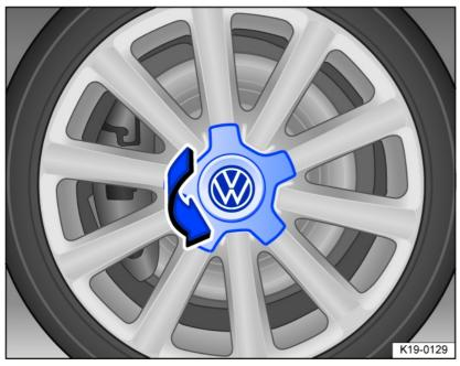
Fig. 166 Twist off the hubcap.
