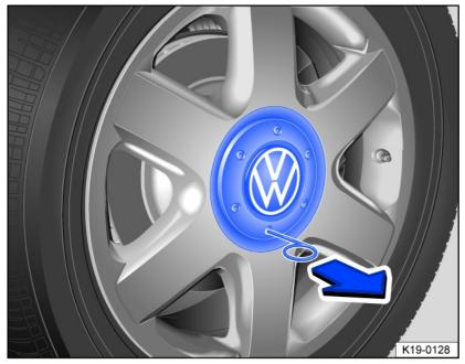
Fig. 165 Remove the wheel center trim.
