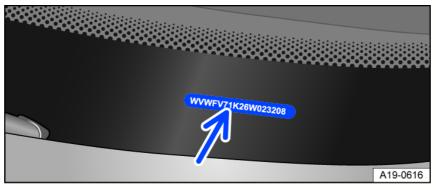
Fig. 183 In the windshield: vehicle identification number (VIN)
