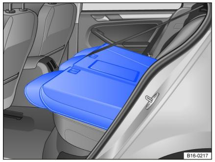
Fig. 71 Rear bench seat: Rear seat backrest folded forwards.
