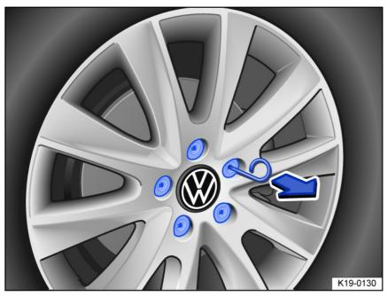
Fig. 168 Remove the caps from the wheel bolts.
