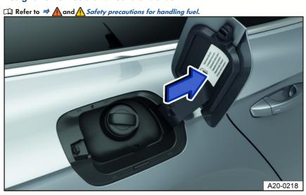
Fig. 129 On the inside of the fuel filler flap: fuel label (general example)
