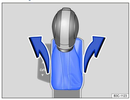
Fig. 104 Remove the cover on the shift gate.
