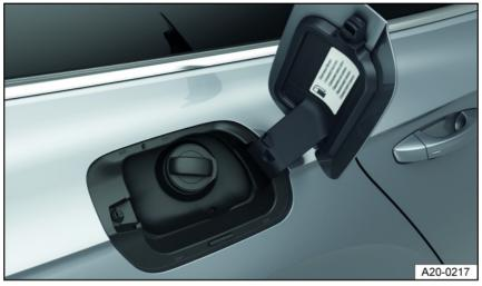
Fig. 130 Behind the fuel filler flap: fuel tank cap (general example)
