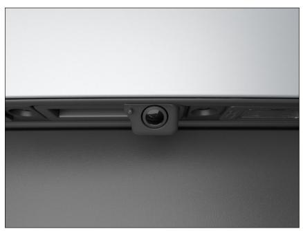
Fig. 182 In the rear of the vehicle: Rear View Camera system on the handle (general example).
