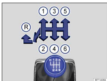
Fig. 110 Gearshift pattern of a 6-speed manual transmission.
