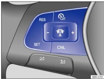
Fig. 121 Left-hand side of the multi-function steering wheel: Buttons for operating the Adaptive Cruise Control (ACC).
