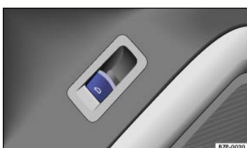
Fig. 67 In the driver door: Switch to open the trunk lid.
