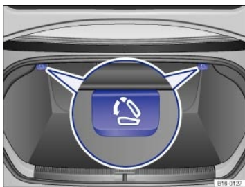
Fig. 77 In the luggage compartment: Release levers for the rear seat backrest.
