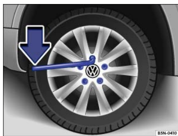
Fig. 177 Changing a wheel: Loosening the wheel bolts.
