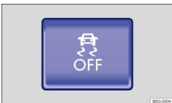
Fig. 129 In the lower center console: Button for switching ASR or ESC Sport mode on and off manually (if equipped).
