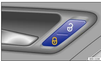
Fig. 58 In the driver and front passenger doors: Power locking switch.
