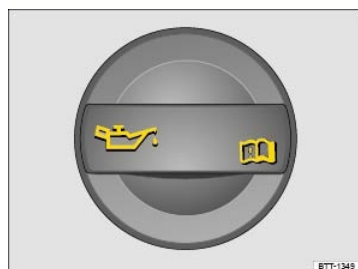
Fig. 162 In the engine compartment: Engine oil filler cap (cap design may vary depending on vehicle equipment).
