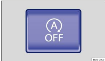
Fig. 109 In the lower center console: Button for the Start-stop system.
