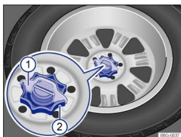
Fig. 170 In the luggage compartment: Handwheel holding the spare wheel in place (if equipped).
