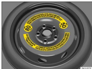
Fig. 171 In the luggage compartment: Compact spare wheel (if equipped, label design may vary).
