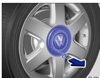
Fig. 173 Pulling the hubcap off.
