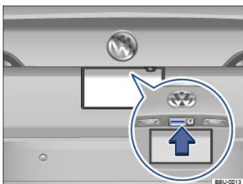
Fig. 66 Opening the trunk lid from the outside.
