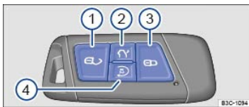
Fig. 107 Remote control vehicle key with remote start button.
