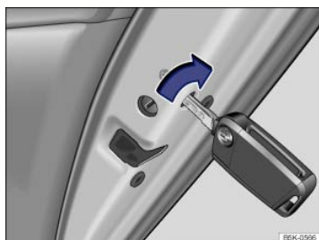
Fig. 63 On the front side of the rear passenger door: Locking the vehicle with the key bit in the vehicle key.
