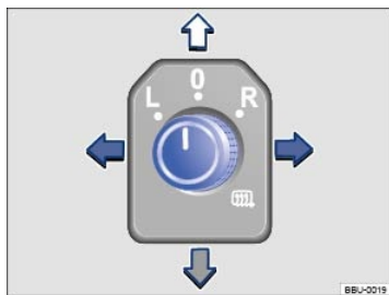
Fig. 94 In the driver door: Adjusting knob for the outside mirrors.
