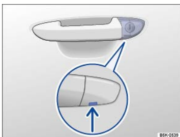
Fig. 60 Driver door: Concealed lock cylinder.
