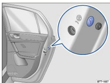
Fig. 62 On the front side of the rear passenger door: Manual lock, covered by a rubber seal (if equipped).
