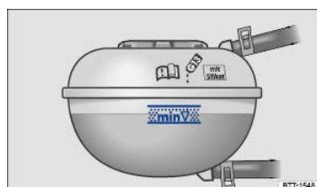
Fig. 163 Coolant expansion tank in the engine compartment.
