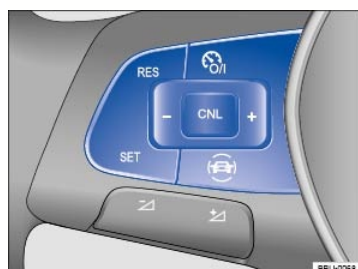
Fig. 118 Left-hand side of the multi-function steering wheel: Buttons for operating the cruise control.
