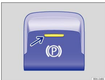
Fig. 126 In the lower center console: Electronic parking brake switch.
