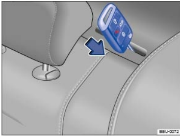
Fig. 69 Behind the rear seat backrest: Release of the rear seat backrest.
