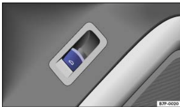
Fig. 59 In the driver door: Switch to open the trunk lid.
