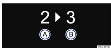
Fig. 101 In the instrument cluster display: Gear recommendation.
