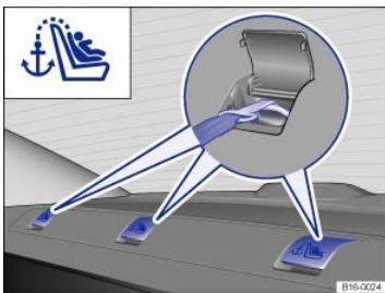
Fig. 46 Behind the rear seat backrest: Top tether anchorages.
