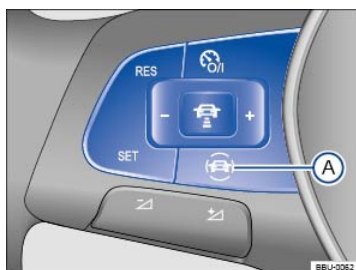
Fig. 18 On the multi-function steering wheel: Driver assistance systems button.
