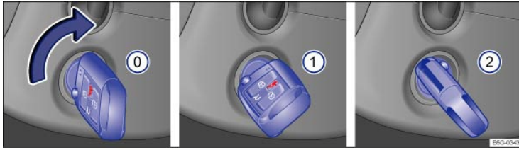
Fig. 105 In the ignition switch: Vehicle key positions for vehicles without Keyless Access.
