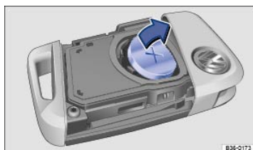
Fig. 54 Remote control vehicle key: Changing the battery.
