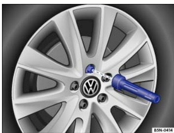
Fig. 180 Changing a wheel: Remove previously loosened wheel bolts using the screwdriver handle.
