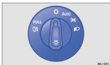
Fig. 87 Headlight switch next to the steering wheel (with fog lights and automatic headlights, if equipped).
