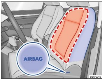
Fig. 38 Location and deployment zone of the side airbags in the padding on the outboard side of the front seat backrests.
