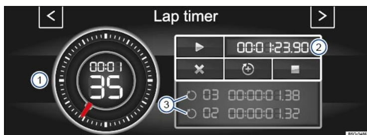
Fig. 20 In the Infotainment system: Performance Monitor lap timer/stopwatch.
