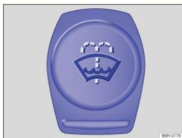
Fig. 160 In the engine compartment: Cap of the windshield washer fluid reservoir.
