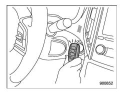
5. Hold the access key fob with the buttons facing you, and touch the pushbutton ignition switch with it.
