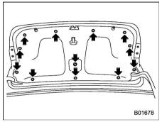
1. Open the trunk and remove the clips from the trunk lid trim with a flat-head screwdriver.
