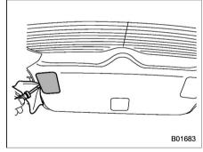
1. Apply a flat-head screwdriver to the light cover as shown in the illustration, and pry the light cover off from the rear gate trim.
