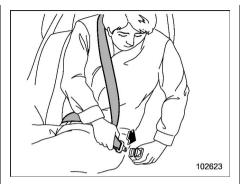
5. Insert the center seatbelt tongue plate into the center seatbelt buckle until it clicks.
