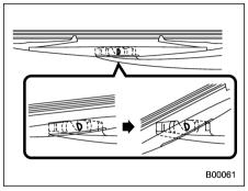
2. Turn the wiper blade assembly counterclockwise.
