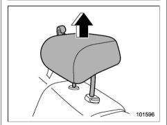
1. Raise the head restraint to the extended position. Do not remove the head restraint.
