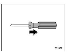
3. Remove the grip portion of the screwdriver.
