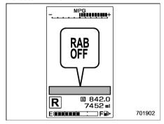
RAB OFF indicator: illuminates when the Reverse Automatic Braking (RAB) system is turned OFF.
