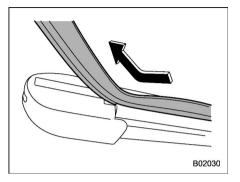
2. Pull the end of the wiper blade rubber through the slit to remove it.
