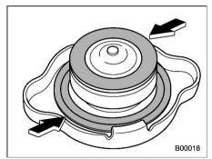
3. After refilling the reserve tank and the radiator, reinstall the cap and check that the rubber gaskets inside the radiator cap are in the proper position.
