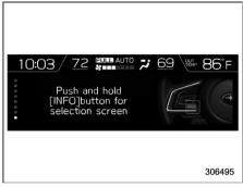
When the INFO button on the steering wheel is pressed and held on this screen, the setting screen can be displayed. For details, refer to "Setting screen" @ 3-55.
