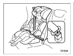
5. To remove the booster seat/cushion. press the release button on the seatbelt buckle and allow the belt to retract.
