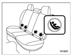
2. You will find marks "Q" at the bottoms of the rear seatback. These marks indicate the positions of the lower anchorages (bars).
