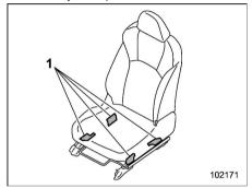
Occupant detection system sensors
