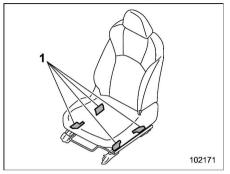
1) Occupant detection system sensors
