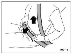
6. To tighten the lap part, pull up on the shoulder belt.
