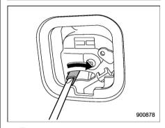
3. To open the rear gate, turn the lever to the right position using a flat-head screwdriver or a similar tool.
