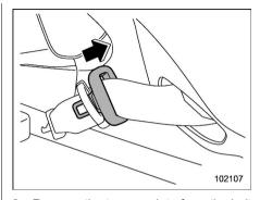
2. Remove the tongue plate from the belt holder on the right side of the cargo area and pull out the seatbelt slowly.
