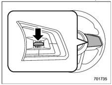
2. Press the "RES/SET" switch to the "SET" side once. Now the desired speed is set and the vehicle will keep running at that speed without depressing the accelerator pedal.
