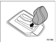
"L" is for using engine braking when going down a hill, etc. To select this mode, move the select lever from the "D" position to the "L" position.
