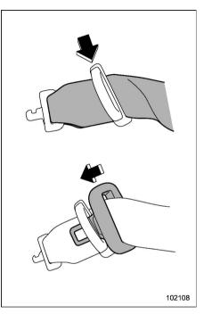
3. Allow the retractor to roll up the belt. You should hold the webbing end and guide it back into the retractor while it is rolling up. Insert the tongue plate into the belt holder.
