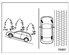
When parking on a hill, always turn the steering wheel. When the vehicle is headed up the hill, the front wheels should be turned away from the curb.
