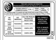
The vehicle placard shows original tire size, recommended cold tire inflation pressure on each tire at maximum loaded vehicle weight. seating capacity and loading information
