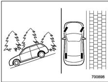
When facing downhill, the front wheels should be turned into the curb.
