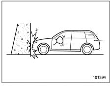
A head-on collision against a thick concrete wall at a vehicle speed of 12 to 19 mph (20 to 30 km/h) or higher activates only the driver's SRS frontal airbag or both driver's and front passenger's SRS frontal airbags. The airbag(s) will also be activated when the vehicle is exposed to a frontal impact similar in fashion and magnitude to the collision described above.
