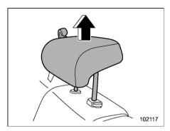
(For 5-door model center seat) Raise the head restraint to the extended position. Do not remove the head restraint.
