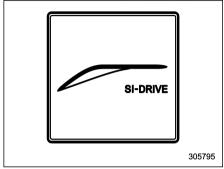
This screen indicates the current SI-DRIVE mode with its throttle angle.
