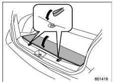
3. Put the cargo floor board back while hanging two retaining straps on the hooks that are located on the rear wall of cargo area.
