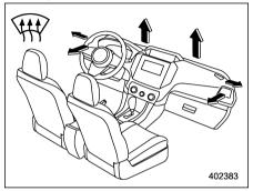
**Defrost for type A:** Windshield defroster outlets and both side outlets of the instrument panel (Refer to "Defrosting" \$\sigma -4-10.)
