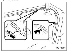
1. Remove the clips from the trunk trim with a flat-head screwdriver.
