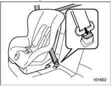
11. To remove the child restraint system, press the release button on the seatbelt buckle and allow the belt to retract completely. The belt will return to the ELR mode.
