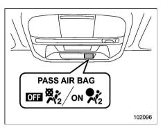
on ♣2: Front passenger's frontal airbag ON indicator
