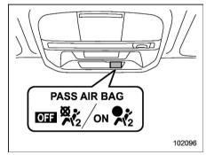
oN ♣2: Front passenger's frontal airbag ON indicator
