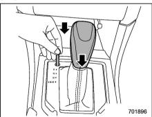
4. While depressing the brake pedal, insert a screwdriver into the hole, move it right and left while pushing the shift lock release button using a screwdriver, and then move the select lever
