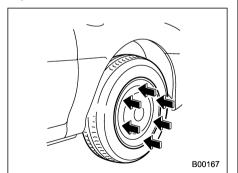
Align the valve with the valve hole in the cover, then fit the cover on the wheel by tapping your hand evenly around the circumference of the cover.
