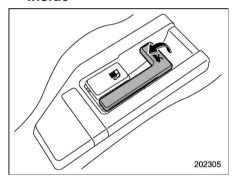
Pull the trunk lid release lever upward. The lever is on the floor at the left of the driver's seat.
