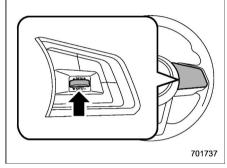
Press the "RES/SET" switch to the "RES" side and hold it until the vehicle reaches the desired speed. Then, release the switch. The vehicle speed at that moment will be memorized and treated as the new set speed.
