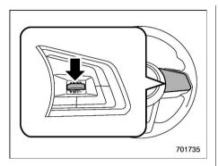
3. Press the "RES/SET" switch to the "SET" side and release it. Then release the accelerator pedal.
