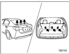
The tether anchorages (upper anchorages) are provided at the locations shown in the above illustration. For details. refer to "Top tether anchorages" \$\tilde{\Pi}\$1-41.
