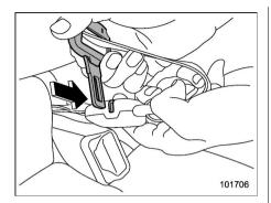
2. Insert a tongue plate or another hard pointed object into the slot in the anchor buckle on the right-hand side and push it in. The anchor tongue plate will then disconnect from the buckle.
