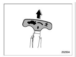
To open the trunk lid from inside the trunk, pull the trunk lid release handle upward as indicated by the arrow on the handle.
