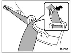
3. After drawing out the seatbelt, pass it through the belt guide as follows: First insert one edge of the belt into the open
