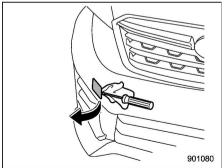
2. Cover the tip of a flat-head screwdriver with vinvl tape or cloth so that it will not scratch the bumper. Insert the flat-head screwdriver into the cutout of the cover and pry open the cover.
