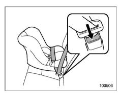
9. To remove the child restraint system, press the release button on the seatbelt buckle and allow the belt to retract completely. The belt will return to the ELR mode.
