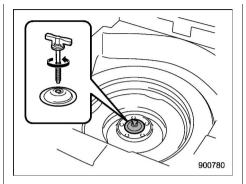
6. Take out the tool bucket and turn the attaching bolt counterclockwise, then take the spare tire out.
