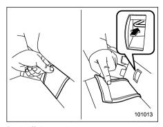
Peel off the anchorage cover completely from the selected side of the rear seat cushion to expose the anchorages (bars) to be used for installation of the child restraint system.
