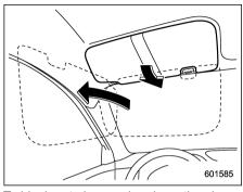
To block out glare, swing down the visors. To use the sun visor at a side window, swing it down and move it sideways.
