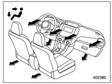
**Bi-level:** Instrument panel outlets and foot outlets
