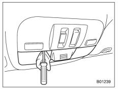
1. Remove the lens by prying the edge of the lens with a flat-head screwdriver.
