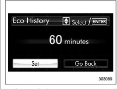
6. Select "Set" by operating the "\( \tilde{\texts}\)" switch and confirm the setting by pushing the (INTER) button.
