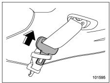
2. Remove the tongue plate from the belt holder on the right side of the cargo area and pull out the seatbelt slowly.
