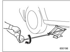
7. Insert the jack handle into the jackscrew, and turn the handle until the tire clears the ground. Do not raise the vehicle higher than necessary.
