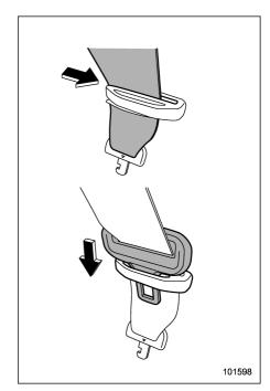
2. Allow the retractor to roll up the belt. You should hold the webbing end and guide it back into the retractor while it is rolling up. Insert the connector (tongue) into the belt holder.
