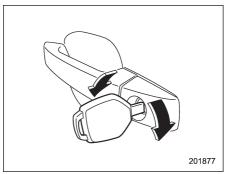
To lock the driver's door from the outside with the key, turn the key toward the front.
