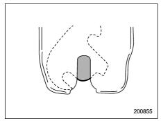
3. Pull the trunk lid release handle from outside the vehicle, as indicated by the arrow on the handle to check if the latch is released.
