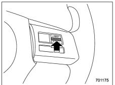
To resume the cruise control after it has been temporarily canceled and with vehicle speed of approximately 20 mph (32 km/h) or more, press the "RES/SET" switch to the "RES" side to return to the original cruising speed automatically.
