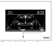
When the Vehicle Dynamics Control system is being activated: the tires illuminate in yellow.
