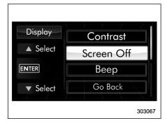
2. Operate the " $\blacktriangle$ " or " $\blacktriangledown$ " switch to select the "Screen Off" item. Then push the INTER button.
