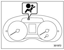
SRS airbag system warning light (type A)
