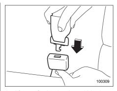
4. After confirming that the webbing is not twisted, insert the connector (tongue) attached at the webbing end into the buckle on the right-hand side until a click is heard.
