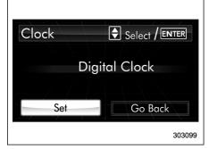
5. Select "Set" by operating the "\sumsets" switch, and confirm the setting by pushing the ENTER button.
