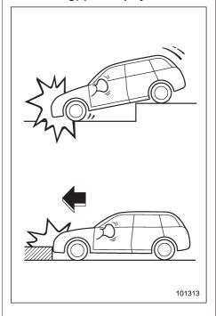
Only the driver's SRS frontal airbag or both driver's and front passenger's SRS frontal airbags may be activated when the vehicle sustains a hard impact in the undercarriage area from the road surface (such as when the vehicle plunges into a deep ditch, is severely impacted or knocked hard against an obstacle on the road such as a curb).
