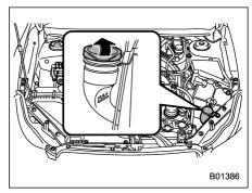
Remove the washer tank filler cap, then add windshield washer fluid until it reaches the "FULL" mark on the tank.
