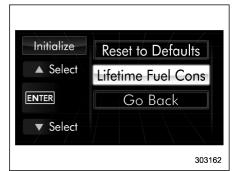
2. Operate the "▲" or "▼" switch to select the "Lifetime Fuel Consumption Resetting" item. Then push the ENTER button.
