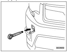
3. Screw the towing hook into the thread
