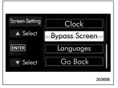
2. Operate the "▲" or "▼" switch to select the "Bypass Screen" item. Then push the me button.
