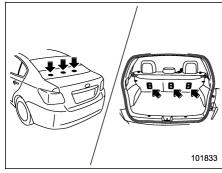
The tether anchorages (upper anchorages) are provided at the locations shown in the above illustration. For details, refer to "Top tether anchorages" \$\tilde{\text{\$\sigma}}\$1-35.
