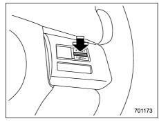
Press the "RES/SET" switch to the "SET" side and hold it until the vehicle reaches the desired speed. Then, release the switch. The vehicle speed at that moment will be memorized and treated as the new set speed.
