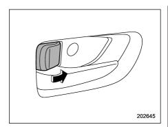
2. Rotate the lock lever forward.
