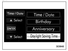
2. Operate the "▲" or "▼" switch to select the "Daylight Saving Time" item. Then push the ENTER button.
