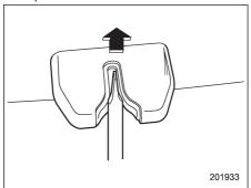
2. Use a flat-head screwdriver with a thin blade. Slide the screwdriver blade from the slit aperture of the lock assembly to the end until you hear a click.
