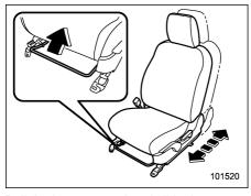
Pull the lever upward and slide the seat to the desired position. Then release the lever and try to move the seat back and forth to make sure that it is securely locked into place.
