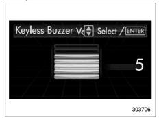
3. Select a volume level by operating the "▲" or "▼" switch, and confirm the setting by pushing the reset button.
