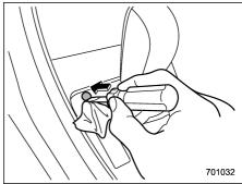
2. Wrap the tip of a flat-head screwdriver with vinyl tape or a cloth and use it to remove the shift lock cover. The shift lock release button is located under the shift lock cover.
