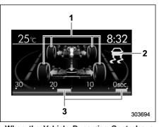
When the Vehicle Dynamics Control system has been activated: the tires remain illuminated in yellow while the Vehicle Dynamics Control System is activated.
