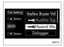
2. Operate the "▲" or "▼" switch to select the "Hazard Warning Flasher" item. Then push the ENTER button.
