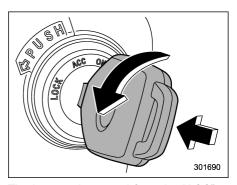
The key can be turned from the "ACC" to "LOCK" (off) position only when the select lever is in the "P" position (CVT models) and the key is pushed in while turning it (all models).
