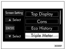
2. Operate the "▲" or "▼" switch to select the "Triple Meter" item. Then push the EMTER button.
