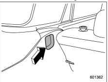
2. Insert both ends of the cover housing into the recesses of the retainers.
