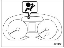
SRS airbag system warning light (type A)
