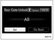
5. Select "Set" by operating the "▼" switch, and confirm the setting by pushing the region button.
