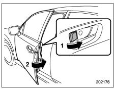
Locking using lock lever
