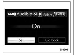
5. Select "Set" by operating the "V" switch, and confirm the setting by pushing the ENTER button.
