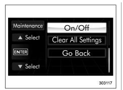
2. Operate the "▲" or "▼" switch to select the "On/Off" item. Then push the enter button.
