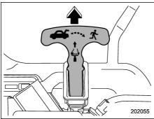
To open the trunk lid from inside the trunk, pull the yellow handle upward as indicated by the arrow on the handle.
