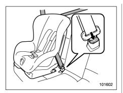
11. To remove the child restraint system, press the release button on the seatbelt buckle and allow the belt to retract completely. The belt will return to the ELR mode.
