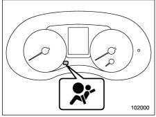
SRS airbag system warning light (type B)
