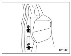
7. Tighten the upper and lower screws.
