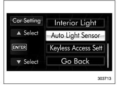
2. Operate the "▲" or "▼" switch to select the "Auto Light Sensor" item. Then push the ™ button.
