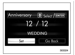
8. After entering the name by repeating step 7, select "Set" by operating the "\(\nbeggreent\)" switch and confirm the setting by pushing the ENTER button.
