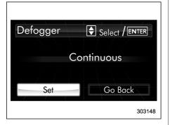
5. Select "Set" by operating the "\state" switch, and confirm the setting by pushing the ENTER button.
