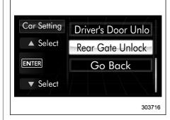
2. Operate the "▲" or "▼" switch to select the "Rear Gate Unlock" item. Then push the ENTER button.
