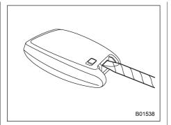
2. Wrap a flat-head screwdriver with vinyl tape or a cloth, and insert it in the gap to remove the cover.
