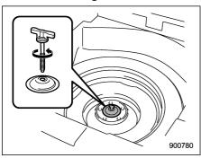
6. Take out the tool bucket and turn the attaching bolt counterclockwise, then take the spare tire out.
