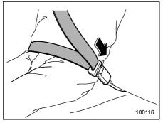
Push the release button of the center seatbelt buckle (on the left-hand side) to unfasten the seatbelt.
