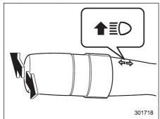
To change from low beam to high beam, push the turn signal lever forward. When the headlights are on high beam, the high beam indicator light "E " on the combination meter is also on.
