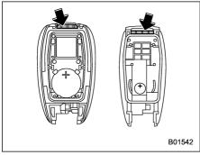
5. Attach the cover to the access key by fitting the projections and recesses together.
