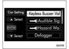
2. Operate the "\( \bigsim \)" or "\( \bigsim \)" switch to select the "Keyless Buzzer Volume" item. Then push the (RTER) button.
