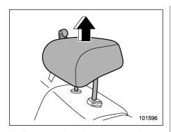
1. Raise the head restraint to the extended position. Do not remove the head restraint.
