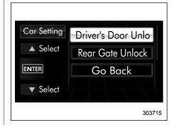
2. Operate the "\( \bigcap \)" or "\( \bigcup \)" switch to select the "Driver's Door Unlock" item. Then push the (NTER) button.
