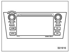
"POWER/VOLUME" knob: Press to turn the audio/visual system on and off. When the system turns on, the last mode is displayed. Press and hold the knob approx. 1.5 seconds or more, turn the display to off.
