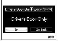
5. Select "Set" by operating the "V" switch, and confirm the setting by pushing the ENTER button.
