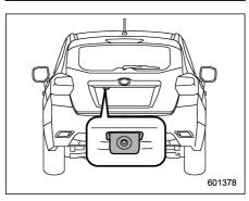
A rear view camera is attached to the trunk lid or rear gate. When the ignition switch is "ON" and the shift lever (MT models) or select lever (CVT models) is set to "R". the rear view camera automatically displays the rear view image behind the vehicle on one of the following displays.
