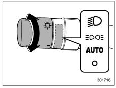
To turn on the headlights, turn the knob on the end of the turn signal lever.
