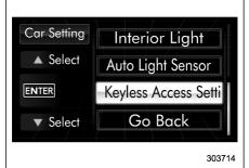
2. Operate the "▲" or "▼" switch to select the "Keyless Access Setting" item. Then push the ™™ button.
