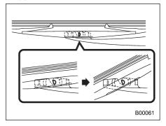
2. Turn the wiper blade assembly counterclockwise.
