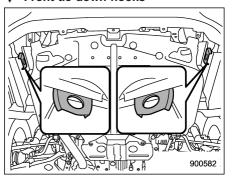
The front tie-down hooks are located between each of the front tires and the
