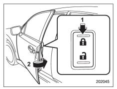
Locking using power door locking switch
