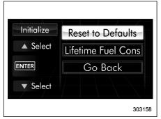
2. Operate the "▲" or "▼" switch to select the "Reset to Defaults" item. Then push the ENTER button.
