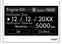
3. Select the setting location (month, day, year or distance) by operating the "\(\nbegin{vmatrix} \text{"} \text{"} \text{ or "A" switch. Then push the ENTER button.
