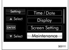
3. After the selection screen is displayed, operate the "A" or "V" switch to show the "Maintenance" item. Then, push the ENTER button.
