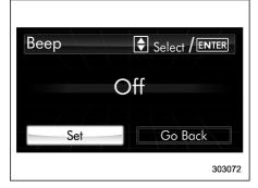
5. Select "Set" by operating the "V" switch, and confirm the setting by pushing the INTER button.
