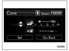
4. Select the displayed configuration by operating the "▲" or "▼" switch. Then push the extent button.
