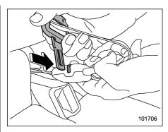
1. Insert a tongue plate or other hard pointed object into the slot in the connector (buckle) on the right-hand side and push it in. The connector (tongue) plate will then disconnect from the buckle.
