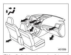
(Bi-level): Instrument panel outlets and foot outlets
