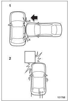
A severe side impact near the front seat or the rear seat.  An offset frontal collision that is severe enough to deploy the front airbag.
