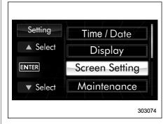
3. After the selection screen is displayed, operate the "▲" or "▼" switch to show the "Screen Setting" item. Then, push the ENTER button.
