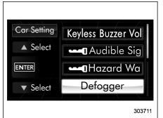
2. Operate the "▲" or "▼" switch to select the "Defogger" item. Then push the ENTER button.
