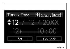
4. Select a number by operating the "▲" or "▼" switch. Then push the MTE button. When "12 h" is selected, the clock will be set to a 12-hour display. When "24 h" is selected, the clock will be set to a 24-hour display.
