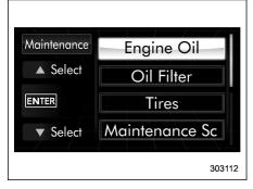
2. Operate the "▲" or "▼" switch to select the "Engine Oil" item. Then push the ENTER button.
