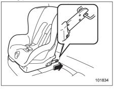
4. While following the instructions supplied by the child restraint system manufacturer, connect the lower hooks onto the lower anchorages located at "" marks on the bottom of the rear seatback. When the hooks are connected, make sure the adjacent seatbelts are not caught.
