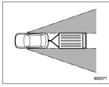
After hitching a trailer to your vehicle, check that the standard side mirrors provide a good rearward field of view without significant blind spots. If significant blind spots occur with the vehicle's standard side mirrors, use towing mirrors that conform with Federal, state/province and/or other applicable regulations.
