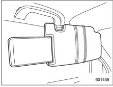
With the sun visor positioned over the side window, you can use the sun visor extension plate to prevent glare through the gap between the sun visor and center pillar. To use the extension plate, pull it toward the rear of the vehicle. When you have finished using it, stow it by pushing it toward the front of the vehicle.
