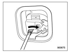
3. To open the rear gate, turn the lever to the right position using a flat-head screwdriver or a similar tool
