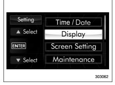
3. After the selection screen is displayed, operate the "\( \bigcup \)" or "\( \bigcup \)" switch to show the "Display" item. Then, push the \( \bigcup \) mes button.
