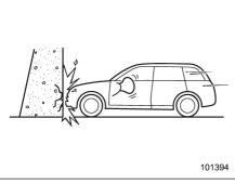
A head-on collision against a thick concrete wall at a vehicle speed of 12 to 19 mph (20 to 30 km/h) or higher activates only the driver's SRS frontal airbag or both driver's and front passenger's SRS frontal airbags. The airbag(s) will also be activated when the vehicle is exposed to a frontal impact similar in fashion and
