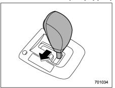
"L" is for using engine braking when going down a hill, etc. To select this mode, move the selector lever from the "D" position to the "L" position.
