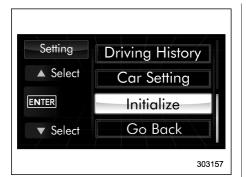
3. After the selection screen is displayed, operate the "A" or "V" switch to show the "Initialize" item. Then, push the ENTER button.
