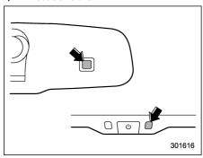
The mirror has a photosensor attached on the front and back sides. During nighttime driving, these sensors detect distracting glare from vehicle headlights behind you and automatically dim the mirror to eliminate glare and preserve your vision. For this reason, use care not to cover the sensors with stickers, or other similar items. Periodically wipe the sensors clean using a piece of dry soft cotton cloth or an applicator.
