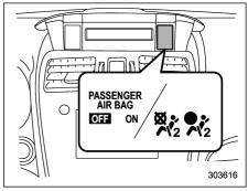
ON / 1: Front passenger's frontal airbag ON indicator
