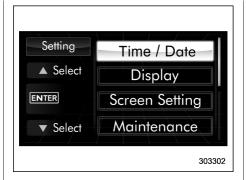
3. After the selection screen is displayed, operate the "\( \\_\)" switch to show the "Time/Date" item. Then, push the ENTER button.
