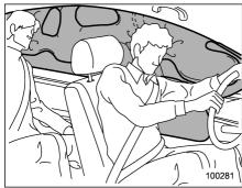
In a moderate to severe side impact collision, the SRS side airbag on the impacted side of the vehicle deploys between the occupant and the door panel and supplements the seatbelt by reducing the impact on the occupant's chest and waist. The SRS side airbag operates only for front seat occupants.
