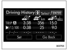
6. Select one of the registration lines by operating the "\( \bigcap \)" or "\( \bigcup '' \) switch. Then push the [ENTER] button.
