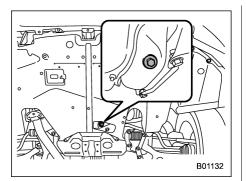
4. Drain out the engine oil by removing the drain plug while the engine is still warm. The used oil should be drained into an appropriate container and disposed of properly.
