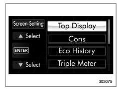
2. Operate the "▲" or "▼" switch to select the "Top Display" item. Then push the ENTER button.
