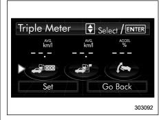
3. Select the setting location (left, center or right) by operating the " $\blacktriangledown$ " or " $\blacktriangle$ " switch. Then push the  $\blacksquare$ NTE button.
