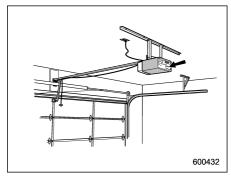
1. Locate the training button on the garage door opener motor head unit. The exact location and color of the button may vary by brand of garage door opener. If it is difficult to locate the training button,
