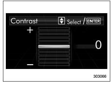
3. Select a contrast level by operating the "▲" or "▼" switch, and confirm the setting by pushing the ▶ button.
