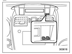
To adjust the time shown by the clock, press the "+" button or "-" button. If you press the "+" button, the indicated time will change in one-minute increments. If you press the "-" button, the indicated time will change in one-minute decrements. If you keep the button pressed, the rate at which the indicated time changes will speed up.
