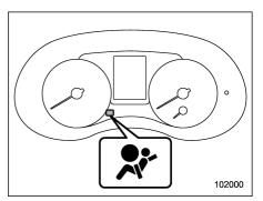
SRS airbag system warning light (type B)
