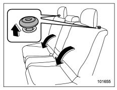
Unlock the seatback by pulling the lock release knob and then fold the seatback down.
