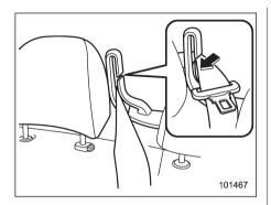
2. After drawing out the seatbelt, pass it through the belt guide as follows: First insert one edge of the belt into the open gap in the belt guide; then slide the rest of the belt in, so that the whole belt fits inside.
