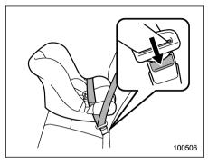
8. To remove the child restraint system. press the release button on the seatbelt buckle and allow the belt to retract completely. The belt will return to the FIR mode.
