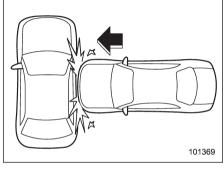
A severe side impact near the front seat activates the SRS side airbag and SRS curtain airbag.
