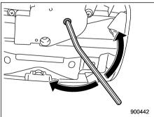
4. Insert the wrench in the end of the motor shaft.
