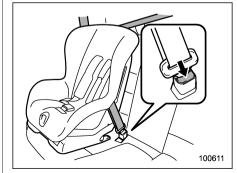
9. To remove the child restraint system, press the release button on the seatbelt buckle and allow the belt to retract completely. The belt will return to the FIR mode.
