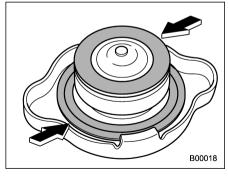
7. Put the radiator cap back on and tighten firmly. At this time, make sure that the rubber gasket in the radiator cap is
