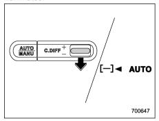
Pull the control switch rearward to select the "AUTO [-]" mode. After setting the mode, "t-]-▲AUTO" on the combination meter illuminates.
