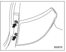
1. Using a Phillips screwdriver, remove the upper and lower screws that secure the rear combination light assembly.
