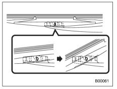
2. Turn the wiper blade assembly counterclockwise.
