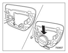
3. Set the fuel filler cap on the cap holder inside the fuel filler lid (turbo models).
