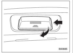
1. Insert a finger into the right side of the license plate light cover, then press once to the left and pull out to remove the cover.
