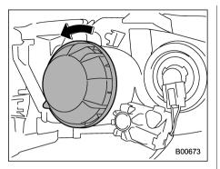
3. Remove the bulb cover, by turning it counterclockwise.
