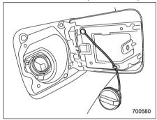
4. Hook the cord that is attached to the fuel filler cap onto the hook inside the fuel filler lid (non-turbo models).
