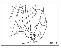
4. Insert the center seatbelt tongue plate into the center seatbelt buckle marked "CENTER" on the left-hand side until it clicks.
