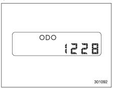
The odometer shows the total distance that the vehicle has been driven.
