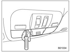
2. Remove the spotlight lens by prying the edge of the lens using flat-head screwdriver.
