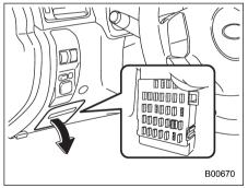
One is located under the instrument panel behind the fuse box cover on the driver's seat side. To remove the cover, pull it out.
