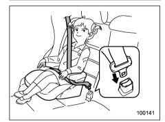
Place the booster seat in the rear seating position and sit the child on it. The child should sit well back on the booster seat.
