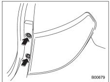
7. Tighten the upper and lower screws.
