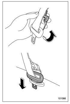
2. Allow the retractor to roll up the belt. You should hold the webbing end and guide it back into the retractor while it is rolling up. Insert the connector (tongue) into the belt holder.
