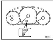
When you select the manual mode of the driver's control center differential, the initial limited slip differential (LSD) torque that is currently selected for the center differential is indicated by the illumination of these indicator lights.
