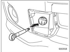
3. Screw the towing hook into the
