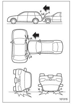
The driver's and front passenger's SRS frontal airbags are designed basically not to deploy if the vehicle is struck from the side or from behind, or if it rolls onto its side or roof, or if it is involved in a lowspeed frontal collision.
