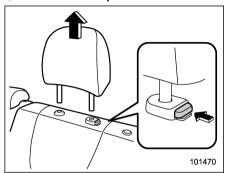
1. Remove the head restraint at the window-side seating position where the child restraint system has been installed with the lower anchorages or seatbelt: lift up the head restraint while pressing the release button. Store the head restraint in the trunk (4-door) or cargo area (5-door). Avoid placing the head restraint in the passenger compartment to prevent it from being thrown around in the passenger compartment in a sudden stop or a sharp turn.
