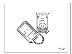
1. Carefully pry the remote engine start transmitter halves apart using a small flathead screwdriver.
