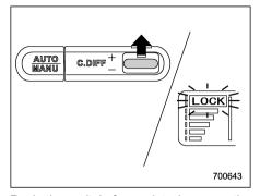
Push the switch forward to increase the initial LSD torque; when the "LOCK" indicator light illuminates, the initial LSD torque setting is maximum. The center differential will then be almost completely locked.
