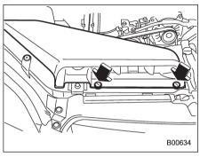
1. Use a screwdriver to undo the clips on the air intake duct, then remove the air intake duct.
