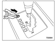
2. Remove the shift lock cover using a flat-head screwdriver. The shift lock release button is located under the shift lock cover
