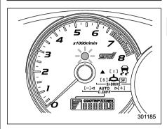
The REV alarm system issues a warning using the REV indicator light (and a buzzer if additionally selected) when the engine speed reaches a level previously set using the trip knob.
