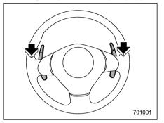
Pull the "+" of the paddle shift to upshift one level. Pull the "-" of the paddle shift to downshift one level.
