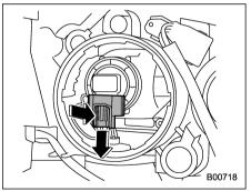
4. Disconnect the electrical connector from the bulb.
