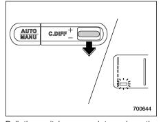
Pull the switch rearward to reduce the initial LSD torque. When the lowest position of the driver's control center differential indicator light illuminates, the initial LSD torque will be minimum. Under this condition, only the Mechanical LSD torque will limit the differential action
