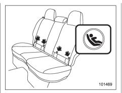
You will find marks "©" at the bottom of the rear seat seatbacks. These marks indicate the positions of the lower anchorages (bars).
