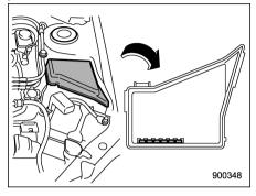
2. Pull any one spare fuse out of the spare fuse holder in the engine compartment. Spare fuses are attached on the back side of the fuse holder cover. You may pick up any one fuse in the spare fuse holder
