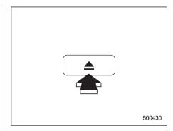
2. Briefly press the "\_\_\_" button. The selected disc will be ejected. The disc number indicator will flash at this time. When you remove the ejected disc, the disc number indicator will turn off.
