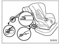
Some types of child restraint systems can be installed on the rear seat of your vehicle without use of the seatbelts. Such child restraint systems are secured to the designated anchorages provided on the vehicle body. The lower and tether anchorages are sometimes referred to as the LATCH system (Lower Anchors and Tethers for CHildren).
