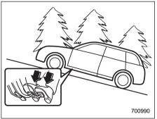
On an uphill grade, when the clutch pedal is depressed while the brake pedal is also depressed, braking power is maintained temporarily by the Hill start assist system when the brake pedal is released. The driver is therefore able to start the vehicle the same way as on a level grade, just using the clutch and accelerator pedal.
