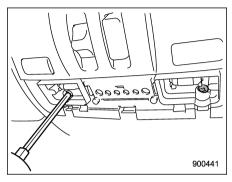
3. Remove the two screws that retain the moonroof switch body. Then, remove the moonroof switch.
