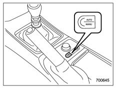
Press the "AUTO-MANU" switch on the center console to switch from auto mode to manual mode or vice versa. When you select the auto mode, the "AUTO" indicator light illuminates. When you select the manual mode, the "AUTO" indicator light turns off.
