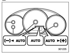
In the auto mode, the system estimates the driving and road conditions using signals from the wheel speed sensor. throttle position sensor, steering angle sensor and brake switch, etc. According to the result, it electronically and automatically controls the degree of limitation of the differential action (LSD torque) to optimize the differential action of the center differential. When the ignition switch is turned ON, the "AUTO" indicator light on the combination meter illuminates.
