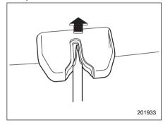
2. Use a flat-head screwdriver with a thin blade. Slide the screwdriver blade from the slit aperture of the lock assembly to the end until you hear a click.
