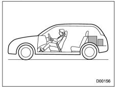
Vehicle capacity weight of the vehicle is 900 lbs (408 kg), which is indicated on the vehicle placard with the statement "The combined weight of occupants and cargo should never exceed 900 lbs or 408 ka".
