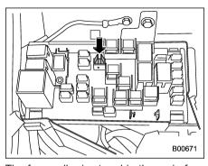
The fuse puller is stored in the main fuse box in the engine compartment.
