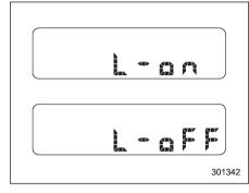
2. Press the trip knob to show "L-oo" or "L-off" on the odometer and trip meter display. The display can be switched as shown in the following illustration by pressing the trip knob.
