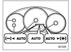
This light functions while the ignition switch is "ON". When illuminated it indicates that the driver's control center differential is set to the auto mode. It turns off when the driver's control center differential is set to the manual mode. For details. refer to "Driver's Control Center Differential (DCCD) (STI)" @7-18.
