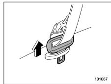
The rear center seatbelt is stowed in the seatbelt holder on the right side of the cargo area.
