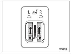
Each seat heater has four levels of adjustment. To use the heater in the right-hand seat, turn the "R" adjustment dial forward until the "\omega" mark reaches the
