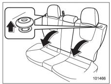
2. Unlock the seatback by pulling the release knob and then fold the seatback down.
