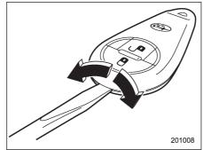
1. Open the transmitter case using a flathead screwdriver.
