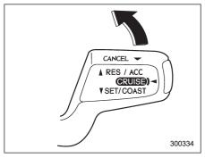
Push the control lever upward in the "RES/ACC" direction and hold it until the vehicle reaches the desired speed. Then, release the control lever. The vehicle speed at that moment will be memorized and treated as the new set speed.
