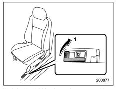
Pull the trunk lid release lever upward.
