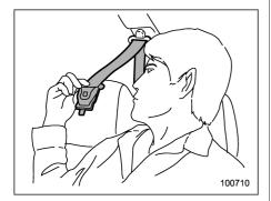
1. Remove the tongue plate from the belt holder located under the right rear quarter glass and pull out the seatbelt slowly.
