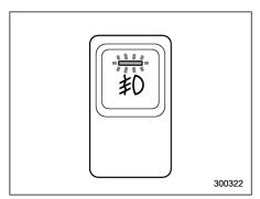
The front fog lights operate only when the headlights are on low beam. Push the front fog light button to turn the front fog lights on.
