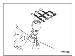
The manual transmission is a fully synchromeshed, 6-forward-speed and 1-reverse-speed transmission.
