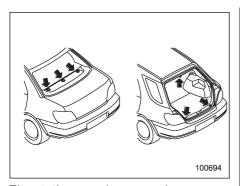
The tether anchorages (upper anchorages) are provided for all the seating positions (center and both window-side ones) of the rear seat.
