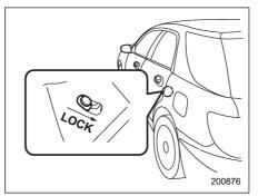
Each rear door has a child safety lock that prevents the doors from being opened even if the inside door handle is pulled.
