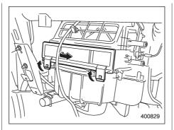
2. Unhook the hooks of the air filter cover and remove the cover.
