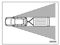
After hitching a trailer to your vehicle, check that the standard side mirrors provide a good rearward field of view without significant blind spots. If significant blind spots occur with the vehicle's standard side mirrors, use towing mirrors that
