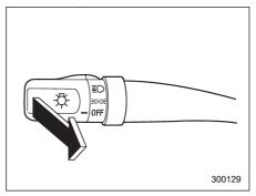
To flash the headlights, pull the lever toward you and then release it. The high beam will stay on for as long as you hold the lever. The headlight flasher works even though the light switch is in the "OFF" position.
