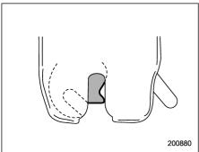
3. Move the release handle, from outside the vehicle, in the direction of the arrow to check if the latch is released.
