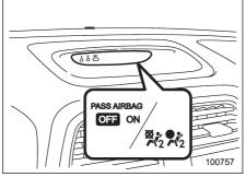
ON or :: Front passenger's frontal airbag ON
