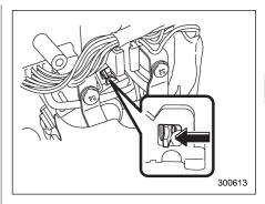
3. Turn the ignition key while pressing the key interlock release lever.
