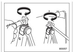
After placing the jack in its storage location, turn the jackscrew clockwise by hand until it becomes too hard to turn. Then, tighten it by an additional 1/4-1/3 of a turn using a screwdriver or the jack handle. Unless the jack is properly secured, it may rattle while the vehicle is moving.
