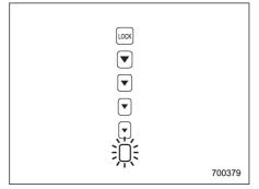
The bottom indicator light "()" flashes in the event of failure of the driver's control center differential. Have the vehicle inspected by your SUBARU dealer. For details, refer to Chapter 7, "Driver's Control Center Differential (DCCD) (WRX-STI)".
