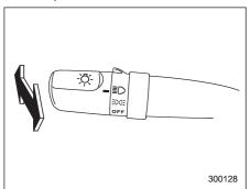
To change from low beam to high beam. push the turn signal lever forward. When the headlights are on high beam, the high beam indicator light "\( \bar{\su} \bar{\su} \)" on the instrument panel is also on.
