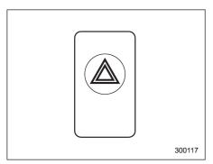
The hazard warning flasher is used to warn other drivers when you have to park your vehicle under emergency conditions. The hazard warning flasher works with the ignition switch in any position.
