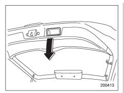
To close the rear gate, lower it slowly and push down firmly until the latch engages. The rear gate can be lowered easily if you pull it down holding the recessed grip.
