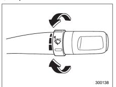
When the wiper switch is in the "\$\sqrt{p}\sigma\$" position, turn the dial to adjust the operating interval of the wiper.
