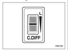
The control dial is located beside the parking brake lever. By turning the control dial forward and rearward, it is possible to change the initial LSD torque.
