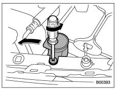
Before replacing the left-hand (batteryside) high-beam light bulb, remove the screw that retains the windshield washer nozzle and tip the windshield washer nozzle sideways.
