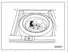
Sedan: Remove the floor cover from the trunk. Turn the attaching bolt counterclockwise, then take the spare tire out.
