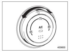
This dial is used to set the desired interior temperature. With the dial set to your desired temperature, the system automatically adjusts the temperature of air supplied from the outlets such that the desired temperature is achieved and maintained.
