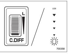
Turn the dial rearward to reduce the initial LSD torque; when the white line reaches the rearmost position, the initial LSD torque will be minimum and the "O" indicator light will come on. Under this condition, only the Mechanical LSD torque will limit the differential action.
