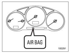
A diagnostic system continually monitors the readiness of the seatbelt pretensioner while the vehicle is being driven. The seatbelt pretensioners share the control module with the SRS airbag system. Therefore, if any malfunction occurs in a seatbelt pretensioner, the SRS airbag system warning light will illuminate. The SRS airbag system warning light will show normal system operation by lighting for approximately 6 seconds when the igni-
