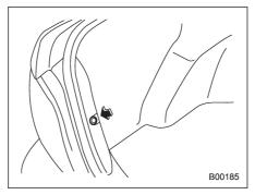
1. Remove the clip from the rear trunk trim with a screwdriver.
