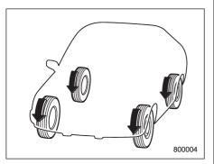
All-Wheel Drive distributes the engine power to all four wheels. AWD vehicles provide better traction when driving on slippery, wet or snow-covered roads and when moving out of mud, dirt and sand. By shifting power between the front and rear wheels, SUBARU AWD can also provide added traction during acceleration and added engine braking force during deceleration
