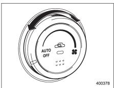
The fan operates only with the ignition switch in the ON position. The fan speed control dial is used to select the AUTO (automatic control) mode or to select the desired fan speed. The dial's positions and their functions are as follows:
