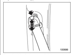
The shoulder belt anchor height should be adjusted to the best position for the passenger. To adjust the anchor height, push the release button and slide the anchor up or down. Pull down on the anchor to make sure that it is locked in place.
