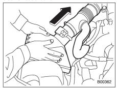
2. Push the air cleaner case cover in the direction of the arrow shown in the drawing.
