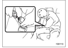
3. After confirming that the webbing is not twisted, insert the connector (tongue) attached at the webbing end into the buckle on the right-hand side until a click is heard.
