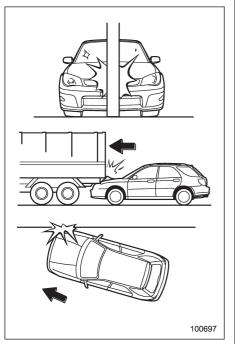
There are many types of collisions which might not necessarily require deployment of driver's/driver's and front passenger's SRS frontal airbag(s). If the vehicle strikes an object, such as a telephone pole or sign pole, or if it slides under a truck's load bed, or if it sustains an oblique offset frontal impact, the driver's/driver's and front passenger's SRS frontal airbag(s) may not deploy depending on the level of accident forces involved.
