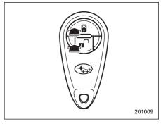
**?** LOCK/ARM button Press to Lock all doors. Press and Hold to activate panic alarm. Press 3 times in a 5-second period to use vehicle finder function.
