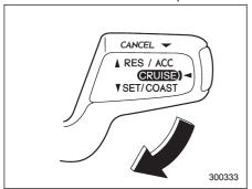
3. Push the control lever downward in the "SET/COAST" direction and release it. Then release the accelerator pedal.
