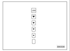
When illuminated, one of these indicator lights indicates the initial limited slip differential (LSD) torque currently selected for the center differential.
