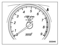
The REV alarm system issues a warning using the REV indicator light (and a buzzer if additionally selected) when the engine speed reaches a level previously set using the REV setting knob.
