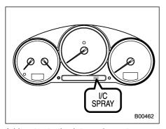
Add water to the intercooler water spray tank when the intercooler water spray warning light in the combination meter comes on. The warning light comes on when the water in the tank has decreased to approximately 0.4 liters (0.4 US qt, 0.4 Imp qt).
