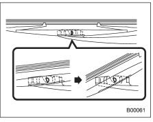
2. Turn the wiper blade assembly counterclockwise.
