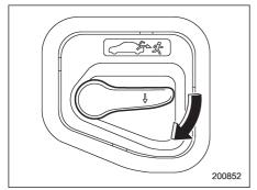
To open the trunk lid from inside the trunk, press the yellow handle downward as indicated by the arrow on the handle.
