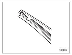
Securely retain both ends of the rubber with the stoppers on the plastic support ends. If the rubber is not retained properly, the wiper may scratch the rear window glass.
