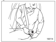
Insert the center seatbelt tongue plate into the center seatbelt buckle marked "CENTER" on the left-hand side until it clicks.
