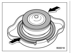
3. After refilling the reserve tank and the radiator, reinstall the caps and check that the rubber gaskets inside the radiator cap are in the proper position.
