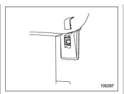
2. (For both window-side seating positions) Remove the cap from the anchor fitting cover.
