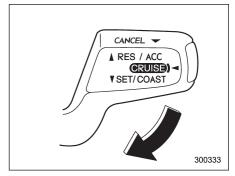
Push the control lever downward in the "SET/COAST" direction and hold it until the vehicle reaches the desired speed. Then, release the control lever. The vehicle speed at that moment will be memorized and treated as the new set speed.
