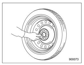
10.Before putting the spare tire on, clean the mounting surface of the wheel and hub with a cloth.
