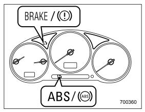
If a malfunction occurs in the EBD system, the system stops working and the brake system warning light and ABS warning light come on simultaneously.
