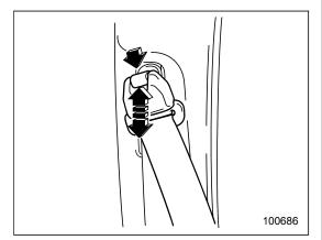
The shoulder belt anchor height should be adjusted to the position best suited for you. To adjust the anchor height, push the release button and slide the anchor up or down. Pull down on the anchor to make sure that it is locked in place.
