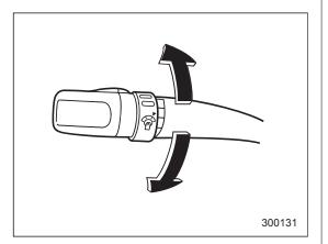
When the headlight switch is in the " <code>\subseteq DOS = " or " \subseteq D " position, you can adjust brightness of the instrument panel illumination for better visibility.</code>
