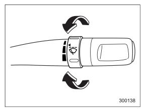
When the wiper switch is in the "  $\nabla$ " position, turn the dial to adjust the operating interval of the wiper.
