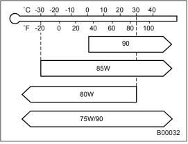
SAE viscosity No. and applicable temperature
