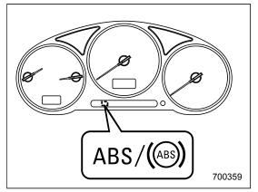
The ABS warning light comes on when the ignition switch is turned to the "ON" position and goes out after approximately two seconds.
