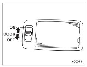
The dome light switch has three positions:
