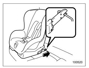
2. While following the instructions supplied by the child restraint system manufacturer, connect the lower hooks onto the lower anchorages located at " " marks on the bottom of the rear seatback. When the hooks are connected, make sure the adjacent seatbelts are not caught.
