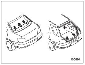
The tether anchorages (upper anchorages) are provided for all the seating positions (middle and both window-side ones) of the rear seat.
