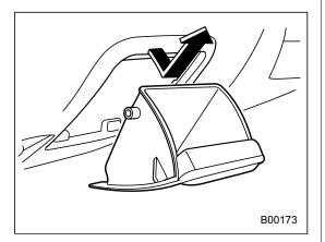
To remove the coin tray, open the cover and pull the coin tray out.
