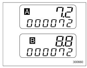
The trip meter shows the distance that the vehicle has been driven since you last set it to zero.
