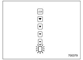
The bottom indicator light " ① " flashes in the event of failure of the driver's control center differential. Have the vehicle inspected by your SUBARU dealer. For details, refer to Chapter 7, "Driver's Control Center Differential (DCCD) (WRX-STI)".
