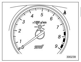
The REV alarm system issues a warning using the REV indicator light (and a buzzer if additionally selected) when the engine speed reaches a level previously set using the REV setting knob.
