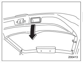
To close the rear gate, lower it slowly and push down firmly until the latch engages. The rear gate can be lowered easily if you pull down on the recessed grip.
