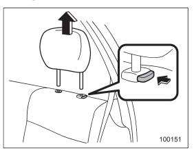
1. Remove the headrest at the windowside seating position where the child restraint system has been installed with the lower anchorages or seatbelt; lift up the headrest while pressing the release button. Store the headrest in the cargo area. Avoid placing the headrest in the passenger compartment to prevent it from being thrown around in the passenger compartment in a sudden stop or a sharp turn.
