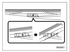
2. Turn the wiper blade assembly counterclockwise.
