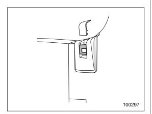
2. (For both window-side seating positions) Remove the cap from the anchor fitting cover by prying it with a screwdriver.
