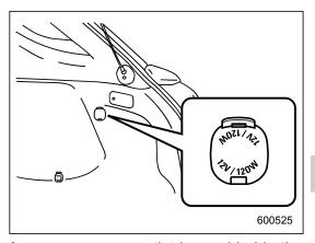
Accessory power outlet is provided in the cargo area (if equipped).
