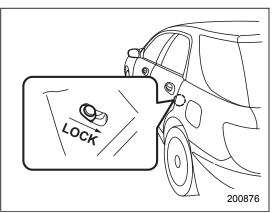
Each rear door has a child safety lock that prevents the doors from being opened even if the inside door handle is pulled. When the child safety lock lever is in the lock position, the door cannot be opened from inside regardless of the position of the inner door handle lock lever. The door can only be opened from the outside.
