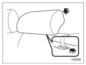
To raise the head restraint, pull it up. To lower it, push the head restraint down while pressing the release button on the top of the seatback.
