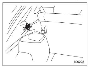
2. Insert the projections located on the both ends of the sleeve into the recesses of the retainers.
