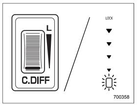
Turn the dial rearward to reduce the initial LSD torque; when the white line reaches the rearmost position, the initial LSD torque will be minimum and the "  $\bigcirc$  " indicator light will come on. Under this condition, only the Mechanical LSD torque will limit the differential action.
