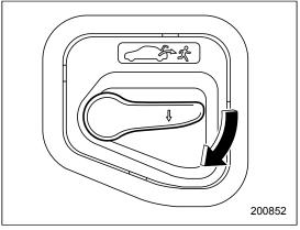
To open the trunk lid from inside the trunk, press the yellow handle downward as indicated by the arrow on the handle.
