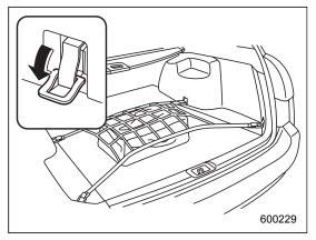
The cargo area is equipped with four tiedown hooks so that cargo can be secured with a cargo net or ropes.
