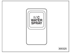
Water is sprayed for approximately two seconds every time the switch is pressed and then released.
