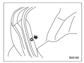
1. Remove the clip from the rear trunk trim with a screwdriver.
