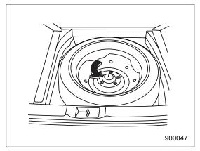
**Sedan:** Remove the floor cover from the trunk. Remove the storage compartment (if so equipped). Turn the attaching bolt counterclockwise, then take the spare tire out.
