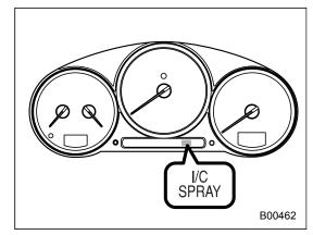
Add water to the intercooler water spray tank when the intercooler water spray warning light in the combination meter comes on. The warning light comes on when the water in the tank has decreased to approximately 0.4 liters (0.4 US qt, 0.4 lmp qt).
