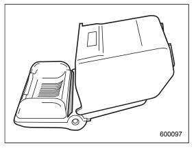
Particles of ash and tobacco will accumulate around the hinges of the ashtray's inner lid. Clean them off using a toothbrush or other narrow-ended implement.
