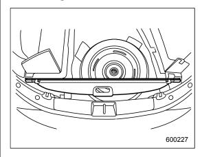
The cargo area cover can be stowed under the cargo floor.
