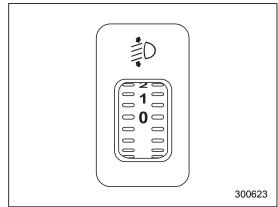
The WRX-STI version has High-Intensity Discharge (HID) headlights on the low beam setting. The HID headlights generate more light than conventional halogen headlights. Therefore a driver of an oncoming vehicle may experience too much glare when your headlight beam height adjustment is high due to the vehicle carrying heavy load.
