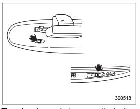
The mirror has a photosensor attached on both the front and back sides. If the glare from the headlights of vehicles behind you strikes the mirror, these sensors detect it and make the reflection surface of the mirror dimmer to help prevent you from being blinded. For this reason, use care not to cover the sensors with stickers, or other similar items. Periodically wipe the sensors clean using a piece of dry soft cotton cloth or an applicator.
