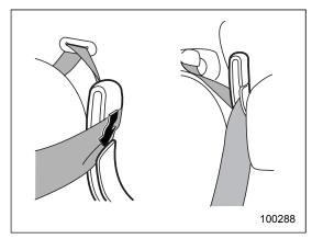
2. After drawing out the seatbelt, pass it through the belt guide as follows: First insert one edge of the belt into the open gap in the comfort guide; then slide the rest of the belt in, so that the whole belt fits inside.
