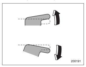
To open the passengers' windows, push the appropriate switch down and hold it until the window reaches the desired position.
