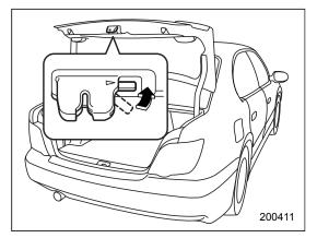
The inside trunk lid release can be cancelled to prevent unauthorized entry into the trunk. To cancel the trunk lid release, set the lid release cancel lever (located on the inside of the trunk lid, mounted to the trunk lid latch) to the "CANCEL" position. When this lock is in the "CANCEL" position, the trunk can be opened only with the key.
