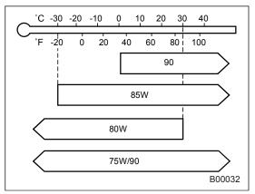
SAE viscosity No. and applicable temperature
