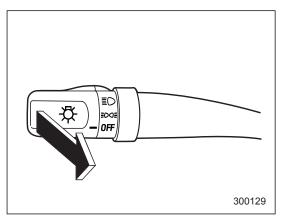
To flash the headlights, pull the lever toward you and then release it. The high beam will stay on for as long as you hold the lever. The headlight flasher works even though the lighting switch is in the "OFF" position.
