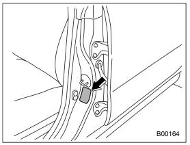
The load capacity of your vehicle is determined by weight, not by available cargo space. The maximum load you can carry in your vehicle is shown on the vehicle
