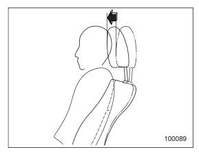
The front seats of your vehicle are equipped with active head restraints. They automatically tilt forward slightly in the event the vehicle is struck from the rear, decreasing the amount of rearward head movement and thus reducing the risk of whiplash. For maximum effectiveness the head restraint should be adjusted so that the center of the head restraint is closest to the top of the occupant's ears.
