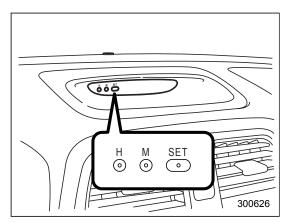
To set the hour, press the "H" button. To set the minutes, press the "M" button. To reset the minutes the "00" with a radio time signal, push the "SET" button.
