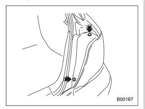
1. Using a Phillips screwdriver, remove the upper and lower clips that secure the side cover of the rear combination light assembly.
