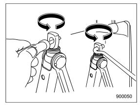
If the jackscrew is too tight to be loosened by hand, loosen it using a screwdriver or the jack handle.
