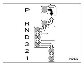
: With the brake pedal depressed, move the lever along the gate.
