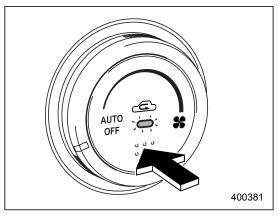
**ON position (Recirculation):** Interior air is recirculated inside the vehicle. Push the air inlet selection button to the ON position for fast cooling with the air conditioner or
