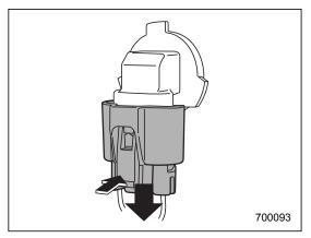
1. Disconnect the electrical connector from the bulb.
