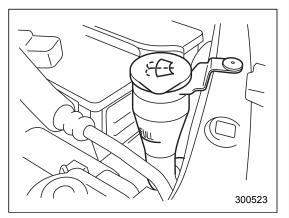
If you spray washer fluid on the windshield but the supply of washer fluid appears to diminish, check the level of washer fluid in the tank.
