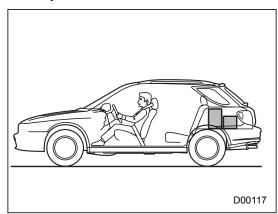
Vehicle capacity weight of the vehicle is 900 lbs (408 kg), which is indicated on the vehicle placard with the statement "The combined weight of occupants and cargo should never exceed 900 lbs or 408 kg".
