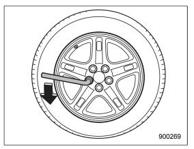
6. Loosen the wheel nuts using the wheel nut wrench but do not remove the nuts.
