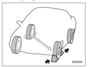
4. Put wheel blocks at the front and rear of the tire diagonally opposite the flat tire.
