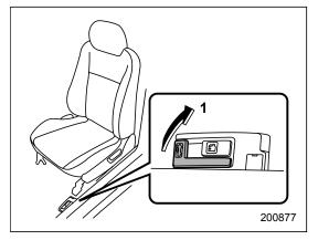
Pull the trunk lid release lever upward.
