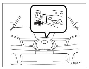
3. Release the secondary hood release located under the front grille by moving the lever toward the left.
