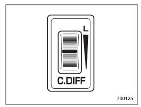
The control dial is located beside the parking-brake lever. By turning the control dial forward and rearward, it is possible to change the initial LSD torque.
