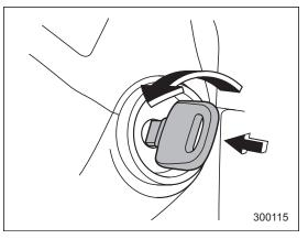
The key can be turned from "ACC" to "LOCK" only when the key is pushed in while turning it.
