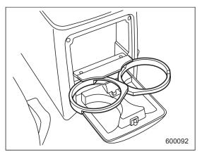
A dual cup holder is located at the back of the center console. To use the cup holder, open the lid by pulling its upper edge.
