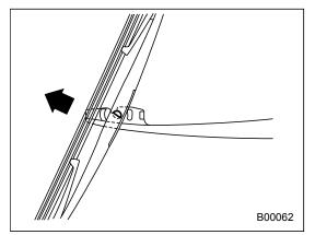
3. Pull the wiper blade assembly toward you to remove it from the wiper arm.
