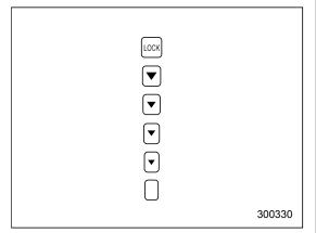
When illuminated, one of these indiator lights indicates the initial limited slip differential (LSD) torque currently selected for the center differential.
