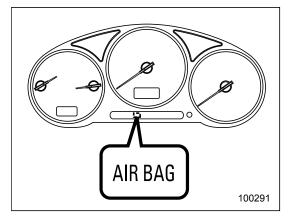
A diagnostic system continually monitors the readiness of the seatbelt pretensioner while the vehicle is being driven. The seatbelt pretensioners share the control module with the SRS airbag system. Therefore, if any malfunction occurs in a seatbelt pretensioner, the SRS airbag system warning light will illuminate. The SRS airbag system warning light will show normal system operation by lighting for approximately 6 seconds when the ignition switch
