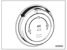
This dial is used to set the desired interior temperature. With the dial set to your desired temperature, the system automatically adjusts the temperature of air supplied from the outlets such that the desired temperature is achieved and maintained. If the dial is turned fully counterclockwise, the system gives maximum cooling performance. If the dial is turned fully clockwise, the system gives maximum heating per-
