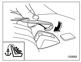
1. Attach the child restraint top tether hook to the appropriate upper anchorage.
