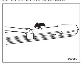
3. Align the claws of the metal support with the grooves in the rubber and slide the blade rubber assembly into the metal support until it locks.
