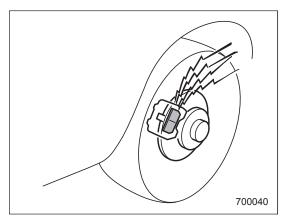
The right front disc brake and the right rear disc brake have audible wear indicators on the brake pads. If the brake pads wear close to their service limit, the wear indicator makes a very audible scraping noise when the brake pedal is applied.
