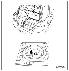
**Wagon:** Open the lid and hang the hook provided on the under side of the lid on the rear edge of the roof to keep the lid open.
