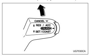
Push the control lever upward in the "RES/ACC" direction and hold it until the vehicle reaches the desired speed. Then, release the control lever. The vehicle speed at that moment will be memorized and treated as the new set speed.
