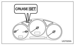
At this time, the " SET " indicator light is illuminated in the combination meter.
