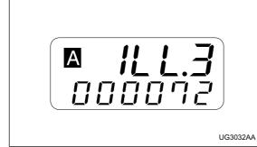
The brightness of the combination meter can be adjusted in five steps with the headlight switch either the OFF position or the " FOSE " or " FOSE " position.
