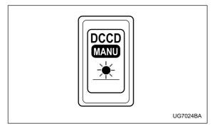
Press the "DCCD-MANU" switch on the center con-
