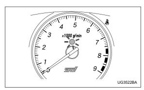
The REV alarm system issues a warning using the REV indicator light (and a buzzer if additionally selected) when the engine speed reaches a level previously set using the REV setting knob.
