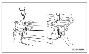
2. Remove the front grille. Use a screwdriver to detach the four clips at the top and the two hooks on each side.
