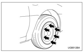
Align the valve with the valve hole in the cover, then fit the cover on the wheel by tapping your hand evenly around the circumference of the cover.
