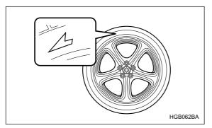
Unidirectional tires: Some tires have a specified direction of rotation. A tire of this type has an arrow or other mark on its side wall to indicate the direction of rotation. Install it so that the direction of rotation is correct when the vehicle is driven forward.
