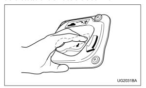
To open the trunk lid from inside the trunk, press the yellow handle downward as indicated by the arrow on the handle.
