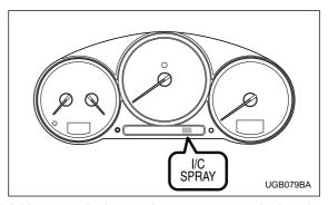
Add water to the intercooler water spray tank when the intercooler water spray warning light in the combination meter comes on. The warning light comes on when the water in the tank has decreased to approximately 0.4 liters (0.4 US qt, 0.4 Imp qt).
