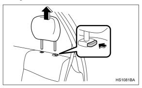
1. Remove the headrest at the seating position where the child restraint system has been installed with the lower anchorages or seatbelt; lift up the headrest while pressing the release button. Store the headrest in the cargo area. Avoid placing the headrest in the passenger compartment to prevent it from being thrown around in the passenger compartment in a sudden stop or a sharp turn.
