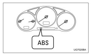
The ABS warning light comes on when the ignition switch is turned to the "ON" position and goes out after about two seconds.
