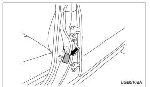
The load capacity of your vehicle is determined by weight, not by available cargo space. The maximum load you can carry in your vehicle is shown as the Vehicle Capacity Weight on the tire information label attached to the driver's side door jamb. It includes the total weight of driver and all passengers and their belongings, any optional equipment such as a trailer hitch, roof rack or bike carrier, etc., and the tongue load of a trailer.
