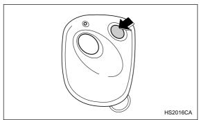
1. Press "UNLOCK/DISARM" button to disarm the security system. (If your vehicle is equipped with the optional security system.)
