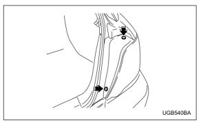
1. Using a Phillips screwdriver, remove the upper and lower screws that secure the side cover of the rear combination light assembly.
