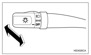
To change from low beam to high beam, push the turn signal lever forward. When the headlights are on high beam, the high beam indicator light "  $\equiv \bigcirc$ " on the instrument panel is also on.
