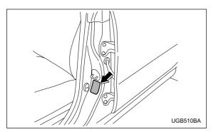
Check the tire pressures when the tires are cold. Use a pressure gauge to adjust the tire pressures to the values shown on the tire placard. The tire placard is located on the door pillar on the driver's side.
