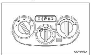
It is possible to obtain air of different temperatures from the instrument panel outlets and foot outlets. Air from the foot outlets is slightly warmer than air from the instrument panel outlets. Make the following settings:
