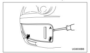
2. Insert a flat-head screwdriver into the slot at point A on the front passenger side fog light cover, then use it to pry the cover upward. The tabs at point A on the fog
