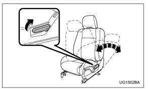
Pull the reclining lever up and adjust the seatback to the desired position. Then release the lever and make sure the seatback is securely locked into place. The seatback placed in a reclined position can spring
