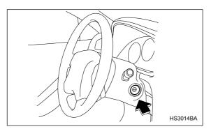
The ignition switch has four positions: LOCK, ACC, ON and START.
