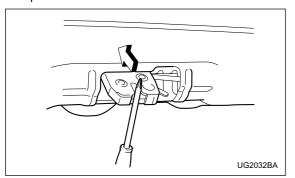
2. Use a screwdriver with a thin blade. Slide the screwdriver blade from the slit aperture of the lock assembly fully to the end until you hear a click.
