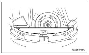
The cargo area cover can be stowed under the cargo floor.
