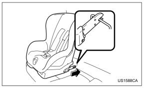
2. While following the instructions supplied by the child restraint system manufacturer, connect the lower hooks onto the lower anchorages located at " marks on the bottom of the rear seatback. When the hooks are connected, make sure the adjacent seatbelts are not caught.
