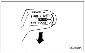
Push the control lever downward in the "SET/COAST" direction and hold it until the vehicle reaches the desired speed. Then, release the control lever. The vehicle speed at that moment will be memorized and treated as the new set speed.
