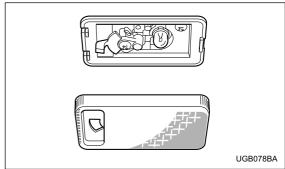
1. Remove the lens by prying the edge of the lens with – *continued* –
