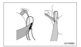
2. After drawing out the seatbelt, pass it through the belt guide as follows: First insert one edge of the belt into the open gap in the comfort guide; then slide the rest of the belt in, so that the whole belt fits inside.
