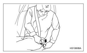
4. Insert the center seatbelt tongue plate in the center seatbelt buckle marked "CENTER" on the left-hand side until it clicks.
