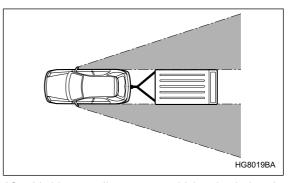
After hitching a trailer to your vehicle, check that the standard side mirrors provide a good rearward field of view without significant blind spots. If significant blind spots occur with the vehicle's standard side mirrors,
