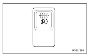
Pressing the fog lights operate only when the headlights are on low beam. Push the fog light switch to turn the fog lights on.
