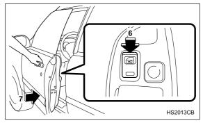
6. Push the front side ("LOCK" side) of the power door locking switch to set the door locks.
