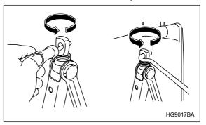
If the jackscrew is too tight to be loosened by hand, loosen it using a screwdriver or the jack handle.
