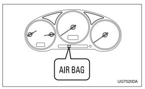
A diagnostic system continually monitors the readiness of the seatbelt pretensioner while the vehicle is being driven. The seatbelt pretensioners share the control module with the SRS airbag system. Therefore, if any malfunction occurs in a seatbelt pretensioner, the SRS airbag system warning light will illuminate. The SRS airbag system warning light will show normal system operation by lighting for about 6 seconds when the ignition key is turned to the "ON" posi-
