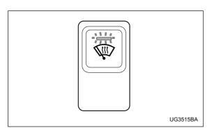
The windshield wiper deicer operates only when the ignition switch is in the "ON" position.
