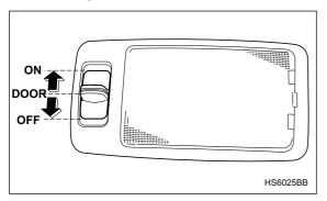
The dome light switch has three positions:
