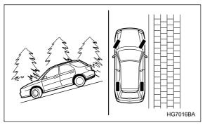
When facing downhill, the front wheels should be turned into the curb.
