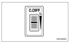
The control dial is located beside the parking-brake lever. By turning the control dial forward and rearward, it is possible to change the differential-action limiting factor of the center differential.
