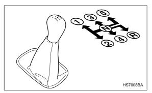
The manual transmission is a fully synchromeshed 5forward and 1-reverse speed transmission.
