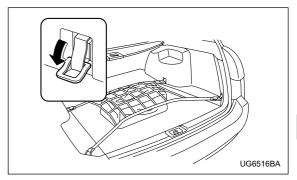
The cargo area is equipped with four tie-down hooks so that cargo can be secured with a cargo net or ropes.
