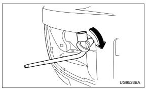
5. Tighten the towing hook securely using the wheel nut wrench.
