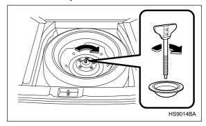
15. Store the flat tire in the spare tire compartment. Put the spacer and tighten the attaching bolt firmly. Also store the jack and wheel nut wrench in their stor-
