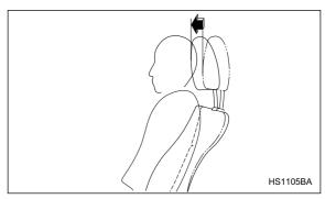
The front seats of your vehicle are equipped with active head restraints. They automatically tilt forward slightly in the event the vehicle is struck from the rear, decreasing the amount of rearward head movement and thus reducing the risk of whiplash. For maximum effectiveness the head restraint should be adjust so
