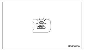
ON position (Recirculation): Interior air is recirculated inside the vehicle. Push the air inlet selection button to the ON position for fast cooling with the air conditioner or when driving on a dusty road. The indicator light will come on.
