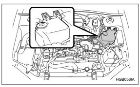
Check the level of the washer fluid at each fuel stop. If the level is low, fill the fluid up to the neck of the reservoir.
