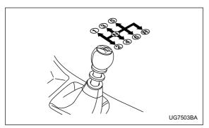
The manual transmission is a fully synchromeshed 6-forward and 1-reverse speed transmission.
