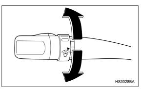
When the headlight switch is in the " <code>=DOE</code> " or " <code>=DO</code> " position, you can adjust brightness of the instrument panel illumination for better visibility.
