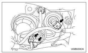
1. Remove two bolts and disconnect connectors.
