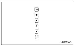
These indicator lights show the current differential-action limiting factor (torque-distribution ratio between the front and rear wheels) of the center differential. The bottom indicator light " ① " flashes in the event of failure of the driver's control center differential. For details, refer to Chapter 7, "Driver's Control Center Differential (DCCD) (WRX-STi)".
