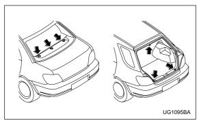
The tether anchorages (upper anchorages) are provided for all the seating positions (middle and both window-side ones) of the rear seat.
