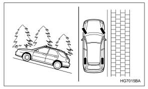
When parking on a hill, always turn the steering wheel. When the vehicle is headed up the hill, the front wheels should be turned away from the curb.
