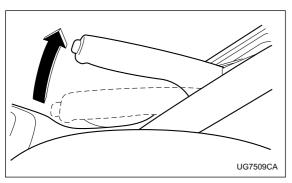
Check the parking brake stroke according to the maintenance schedule in the "Warranty and Maintenance Booklet". When the parking brake is properly adjusted, braking power is fully applied by pulling the lever up seven to eight notches gently but firmly (about 44 lb, 196 N, 20 kg). If the parking brake lever stroke is not within the specified range, have the brake system checked and adjusted at your SUBARU dealer.
