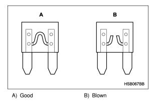
If any lights, accessories or other electrical controls do not operate, inspect the corresponding fuse. If a fuse has blown, replace it.
