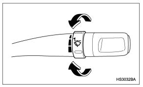
When the wiper switch is in the "\( \opi \)" position, turn the dial to adjust the operating interval of the wiper.
