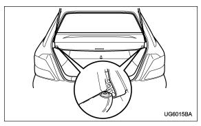
To extend the cover, pull the end of the cover out of the housing, then insert its hooks into the catches as shown. To rewind it, unhook it from the catches and it will rewind automatically. You should hold on to the cover and guide it back into the cover housing while it is rewinding.
