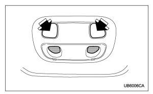
To turn on the spotlight, push the switch. To turn it off, push the switch again.
