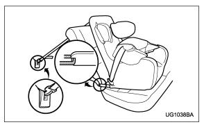
Some types of child restraint systems can be installed on the rear seat of your vehicle without use of the seatbelts. Such child restraint systems are secured to the designated anchorages provided on the vehicle body.
