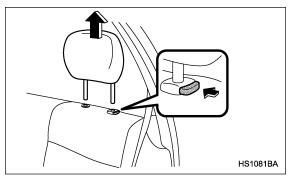
1. Remove the rear seat headrest at the seating position where the child restraint system has been installed with the seatbelt or lower anchorages; lift up the headrest while pressing the release button. Store the headrest in the cargo area. Avoid placing the headrest in the passenger compartment to prevent it from being thrown around in the passenger compartment in a sudden stop or a sharp turn.
