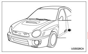
The certification plate attached to the driver's side door jamb shows GVWR (Gross Vehicle Weight Rating) and GAWR (Gross Axle Weight Rating).
