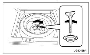
15. Store the flat tire in the spare tire compartment. Put the spacer and tighten the attaching bolt firmly. Also store the jack and wheel nut wrench in their storage locations.
