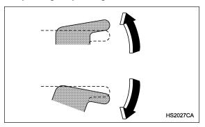
To open the passengers' windows, push the appropriate switch down and hold it until the window reaches the desired position.
