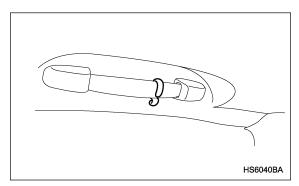
The coat hook is attached to the rear left passenger's hand grip.
