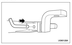
2. Insert the hitch pin into the hole on the hitch receiver tube so that the pin passes through the ball mount.
