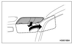
To block out glare, swing down the visors. To use the sun visor at a side window, swing it down and move it sideways.
