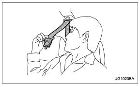
1. Remove the tongue plate from the belt holder located under the right rear quarter glass and pull out the seatbelt slowly.
