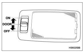
The dome light switch has three positions:
