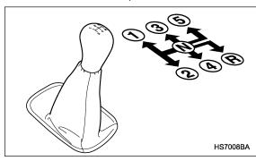
The shift pattern is shown on the shift lever knob. When shifting from 5th gear to reverse gear, first return the shift lever to the neutral position then shift into reverse gear.
