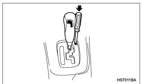
4. Insert the screwdriver into the hole.
