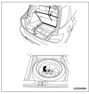
**Wagon:** Open the lid and hang the hook provided on the under side of the lid on the rear edge of the roof to keep the lid open.
