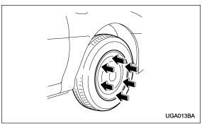
Align the valve with the valve hole in the cover, then fit the cover on the wheel by tapping your hand evenly around the circumference of the cover.
