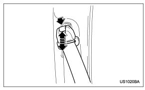
The shoulder belt anchor height should be adjusted to the position best suited for you. To adjust the anchor height, push the release button and slide the anchor up or down. Pull down on the anchor to make sure that it is locked in place.
