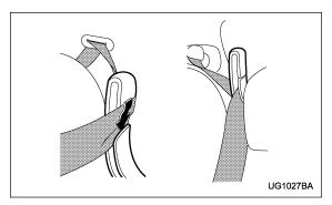
2. After drawing out the seatbelt, pass it through the belt guide as follows: First insert one edge of the belt into the open gap in the comfort guide; then slide the rest of the belt in, so that the whole belt fits inside.
