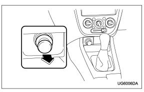
The electrical power outlet located on the lower part of the instrument panel can be used as cigarette lighter socket. A cigarette lighter plug is an optional accessory. It is available from your SUBARU dealer. The cigarette lighter socket may also be used as a power source for an in-car use electrical appliance.
