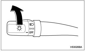
To turn on the headlights, turn the knob on the end of the turn signal lever.
