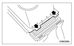
4. To install the air cleaner case cover, insert the two projections on the air cleaner case cover into the slits on the air cleaner case and then snap the two clamps on the air cleaner case cover.
