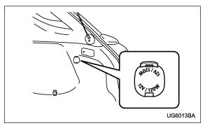
Electrical power (12V DC) from the battery is on tap at the socket when the ignition switch is either in the "ACC" or "ON" position.
