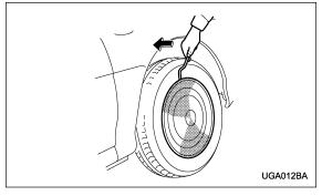
6. (If your vehicle has wheel covers) Insert the wheel cover remover into the notch provided in the wheel cover, and pry it off.
