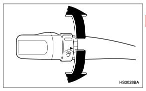
When the lighting switch is in the "₹05" or "≣D" position, you can adjust brightness of the instrument panel illumination for better visibility.
