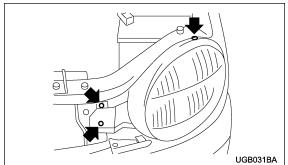
3. Remove three bolts and disconnect connectors,
