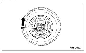
14. Use the wheel nut wrench to securely tighten
