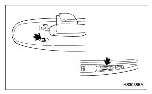
The mirror has a photosensor attached on both the front and back sides. If the glare from the headlights of vehicles behind you strikes the mirror, these sen-
