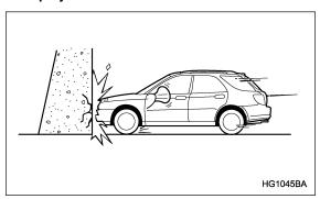
A head-on collision against a thick concrete wall at a vehicle speed of 12 to 19 mph (20 to 30 km/h) or higher activates the SRS frontal airbag. The SRS frontal airbag will also be activated when the vehicle is exposed to a frontal impact similar in fashion and magnitude to the above-mentioned collision.
