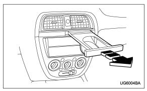
To use the cup holder, push its front surface and pull it out completely.
