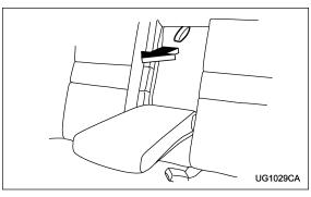
Folding down the armrest and opening the seatback panel affords a loading space for long objects. To open the seatback panel, pull the release tab.
