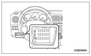
One is located under the instrument panel behind the coin tray on the driver's seat side.
