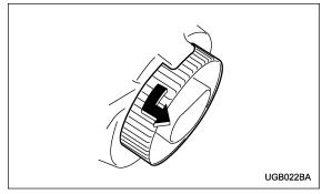
2. Remove the bulb holder from the headlight assembly by turning it counterclockwise.
