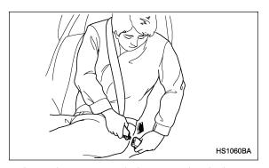
4. Insert the center seatbelt tongue plate in the center seatbelt buckle marked "CENTER" on the left-hand side until it clicks.
