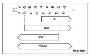
SAE viscosity No. and Applicable Temperature
