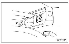
The seat heater operates when the ignition switch is either in the "ACC" or "ON" position.
