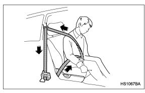
The driver's and front passenger's seatbelts have a seatbelt pretensioner. The seatbelt pretensioners are designed to be activated in the event of an accident involving a moderate to severe frontal collision.
