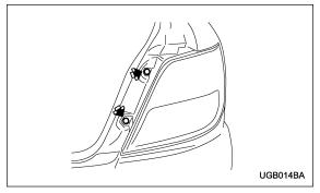
2. Remove the upper and lower screws. Then, slide the rear combination lamp assembly to the rear and remove it from the vehicle.
