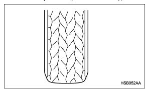
Roadholding is good, and steering is responsive. Rolling resistance is low, so fuel consumption is also lower. • Abnormally low tire pressure (tread worn at shoulders)
