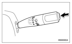
To wash the windshield, push the washer button at the end of the wiper control lever. The washer fluid sprays until you release the washer button. The wipers operate while you push the button.
