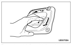
To open the trunk lid from inside the trunk, press the yellow handle downward as indicated by the arrow on the handle.
