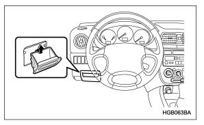
To remove the coin tray, open the cover and pull the coin tray out.
