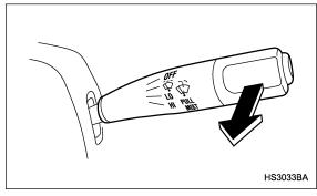
For a single wipe of the wipers, pull the lever toward you. The wipers operate until you release the lever.
