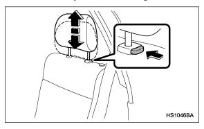
To raise the headrest, pull it up. To lower it, push the head rest down while depressing the release button on the top of the seatback.
