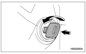
The key can be turned from "ACC" to "LOCK" only when the key is pushed in while turning it.
