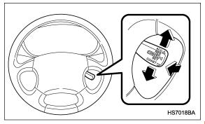
3. Push the control lever downward in the "SET, COAST" direction and release it. Then release the accelerator pedal.
