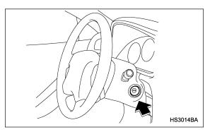
The ignition switch has four positions: LOCK, ACC, ON and START.
