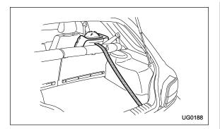
If the child restraint system requires a top tether, latch the hook onto the top tether anchor and tighten the top tether. See the "Top tether anchorages" for additional instructions.
