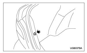
1. Remove the clip from the rear trunk trim with a regular screwdriver.
