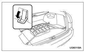
The cargo area is equipped with four tie-down hooks so that cargo can be secured with a cargo net or ropes.
