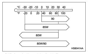
SAE viscosity No. and Applicable Temperature
