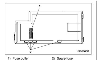
The fuse puller and spare fuses are stored in the main fuse box cover in the engine compartment.
