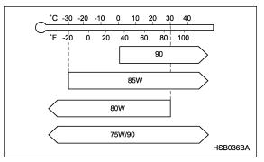
SAE viscosity No. and Applicable Temperature
