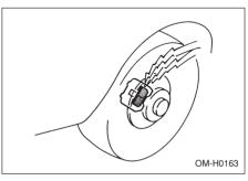
The front disc brakes and the right rear disc brake have an audible wear indicators on the brake pads. If the brake pads wear close to their service limit, the wear indicator makes a very audible scraping noise when the brake pedal is applied.
