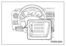
The one is located under the instrument panel behind the fuse box cover on the driver's seat side.
