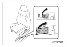
1. To open the fuel filler lid, pull the lid release lever up.
