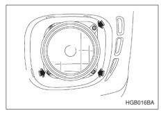
1. Remove the front fog light assembly by removing the three bolts.
