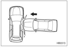
A severe side impact near the front seat activates the SRS side airbag.
