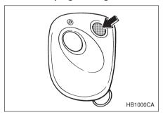
1. Press "UNLOCK/DISARM" button to disarm the security system. (If your vehicle is equipped with the optional security system.)
