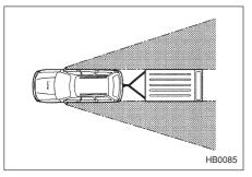
After hitching a trailer to your vehicle, check that the standard side mirrors provide a good rearward field of view without significant blind spots. If significant blind spots occur with the vehicle's standard side mirrors, use towing mirrors that conform with Federal, state/province and/or other applicable regulations.
