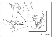
2. Allow the retractor to roll up the belt. You should hold the webbing end and guide it back into the retractor while it is rolling up. Insert the tongue plate into the belt holder.
