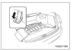
The cargo area is equipped with four anchorage eyelets so that luggage can be secured with a luggage net or ropes.
