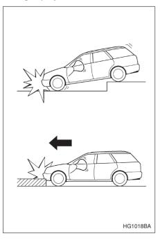
The SRS frontal airbag may be activated when the vehicle sustains a hard impact in the undercarriage area from the road surface (such as when the vehicle plunges into a deep ditch, is severely bumped or knocked hard against an obstacle on the road such as a curb).
