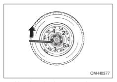
14. Use the wheel nut wrench to securely tighten the wheel nuts to the specified torque, following the tightening order in the illustration.
