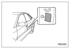
The load capacity of your vehicle is determined by weight, not by available cargo space. The maximum load you can carry in your vehicle is shown as the Vehicle Capacity Weight on the tire information label attached to the driver's side door jamb. It includes the total weight of driver and all passengers and their belongings, any optional equipment such as a trailer hitch, roof rack or bike carrier, etc., and the tongue load of a trailer.
