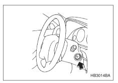
The ignition switch has four positions: LOCK, ACC, ON and START
