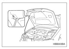
Lift up the hood, release the hood prop from its retainer and put the end of the hood prop into the slot in the hood
