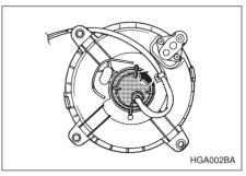
3. Remove the front fog light case cap by turning it counterclockwise.
