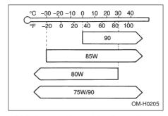
SAE viscosity No. and Applicable Temperature
