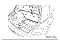
The storage tray is located under the floor of the cargo area and can be used to store small items. To open the lid, pull the tab up.
