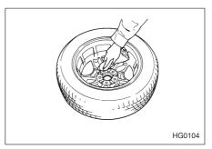
11. Before putting the spare tire on, clean the mounting surface of the wheel and hub with a cloth.
