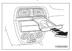
To use the cup holder, push its front surface and pull it out completely.
