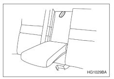
Folding down the armrest and opening the seatback panel affords a loading space for long objects. To open the seatback panel, pull the release tab.
