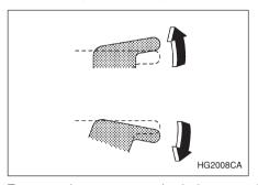
To open the passengers' windows, push the appropriate switch down and hold it until the window reaches the desired position. To close the window, pull the switch up and hold it until it reaches the desired position.
