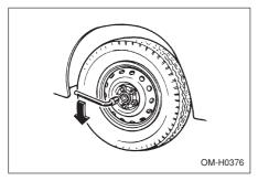
7. Loosen the wheel nuts using the wheel nut wrench but do not remove the nuts.
