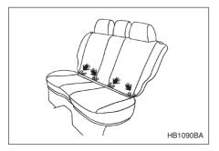
The lower anchorages (bars) are used for installing a child restraint system only on the rear seat window-side seating positions. For each window-side seating position, two lower anchorages are provided.
