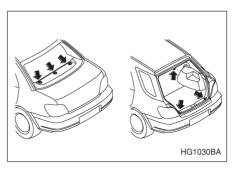
The tether anchorages (upper anchorages) are provided for all the seating positions (middle and both window-side ones) of the rear seat.
