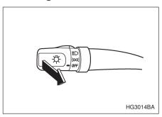
To flash the headlights, pull the lever toward you and then release it. The high beam will stay on for as long as you hold the lever. The headlight flasher works even though the lighting switch is in the "OFF" position.
