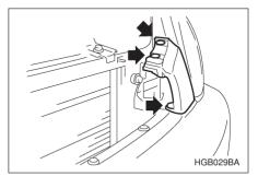
3. Remove three bolts and disconnect connectors, and then detach headlight assembly.
