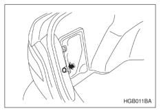
1. Remove the clip from the rear trunk trim with a regular screwdriver.
