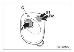
A: LOCK/ARM button Press to Lock all doors. Press and Hold to activate panic alarm.
