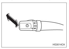
To change from low beam to high beam, push the turn signal lever forward. When the headlights are on high beam, the high beam indicator light "≣○" on the instrument panel is also on.
