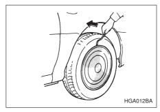
6. (If your vehicle has wheel covers) Insert the wheel cover remover into the notch provided in the wheel cover, and pry it off.
