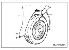
Insert the wheel cover remover into the notch provided, and pry the wheel cover off.
