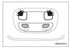
To turn on the spotlight, push the switch. To turn it off, push the switch again.
