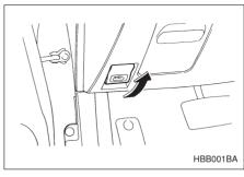
1. Pull the hood release knob under the instrument panel.
