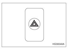
The hazard warning flasher is used to warn other drivers when you have to park your vehicle under emergency conditions. The hazard warning flasher works with the ignition switch in any position.
