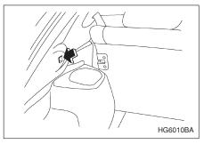
2. Insert the projections located on the both ends of the sleeve into the recesses of the retainers.
