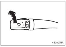
To turn on the headlights, turn the knob on the end of the turn signal lever.
