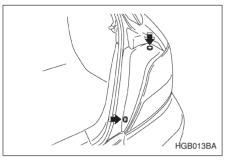
1. Using a Phillips screwdriver, remove the upper and lower screws that secure the side cover of the rear combination light assembly.
