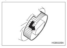
2. Remove the bulb holder from the headlight assembly by turning it counterclockwise.
