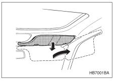
To block out glare, swing down the visors. To use the sun visor at a side window, swing it down and move it sideways.
