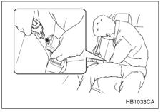
If the belt stops before reaching the buckle, return the belt slightly and pull it out more slowly. If the belt still cannot be unlocked, let the belt retract slightly after giving it a strong pull, then pull it out slowly again. 4. Insert the center seatbelt tongue plate in the center seatbelt buckle marked "CENTER" on the left-hand side until it clicks.
