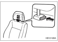
To lower it, push the head restraint down while pressing the release button on the top of the seat-back
