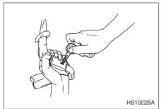
1. Insert a key or other hard pointed object into the slot in the connector (buckle) on the right-hand side and push it in, and the connector (tongue) plate will
