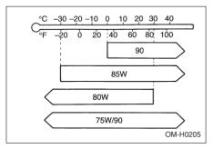
SAE viscosity No. and Applicable Temperature
