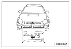
2. Release the secondary hood release located under the front grille by moving the lever toward the left.
