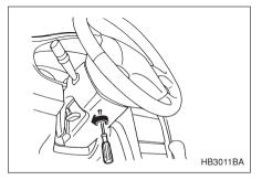
2. Remove the cover under the steering column using a phillips screwdriver.
