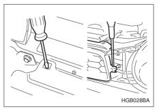
2. Loosen three clips to remove the headlight side cover.
