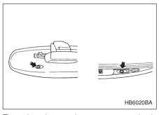
The mirror has a photosensor attached on both the front and back sides. If the glare from the headlights of vehicles behind you strikes the mirror, these sensors detect it and make the reflection surface of the mirror dimmer to help prevent you from being
