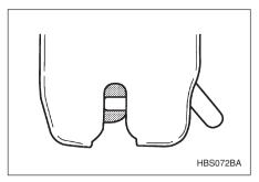
3. Move the release handle, from outside the vehicle, in the direction of the arrow to check if the latch is released
