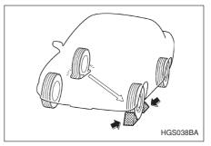
4. Put wheel blocks at the front and rear of the tire diagonally opposite the flat tire.
