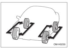
Tire wear varies from wheel to wheel. To maximize the life of each tire and ensure that the tires wear uniformly, it is best to rotate the tires every 7,500 miles (12,500 km). Rotating the tires involves switching the front and rear tires on the right-hand side of the vehicle and similarly switching the front and rear tires on the left-hand side of the vehicle. (Each tire must be kept on its original side of the vehicle.)
