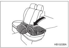
Unlock the seatback by pulling the release knob and then fold the seatback down.
