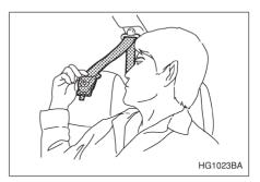
1. Remove the tongue plate from the belt holder located under the right rear quarter glass and pull out the seatbelt slowly.
