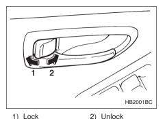
To lock the door from the inside, rotate the lock lever rearward. To unlock the door from the inside, rotate the lock lever forward
