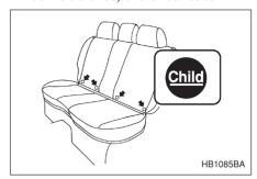
You will find marks "Child" at the bottom of the rear seat seatbacks. These marks indicate the positions of the lower anchorages (bars).
