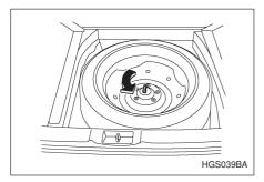
**Sedan:** Remove the floor cover from the trunk. Remove the storage tray (if so equipped). Turn the attaching bolt counterclockwise, then take the spare tire out.
