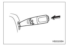
To wash the windshield, push the washer button at the end of the wiper control lever. The washer fluid sprays until you release the washer button. The wipers operate while you push the button.
