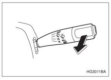
For a single wipe of the wipers, pull the lever toward you. The wipers operate until you release the lever.
