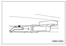
3. Insert the safety pin into the hitch pin securely.
