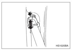
Always adjust the anchor height so that the shoulder belt passes over the middle of the shoulder without touching the neck.
