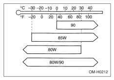
SAE viscosity No. and Applicable Temperature
