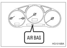
A diagnostic system continually monitors the readiness of the seatbelt pretensioner while the vehicle is being driven. The seatbelt pretensioners share the control module with the SRS airbag system. Therefore, if any malfunction occurs in a seatbelt pretensioner, the SRS airbag system warning light will illuminate. The SRS airbag system warning light will show normal system operation by lighting for about 6 seconds when the ignition key is turned to the "ON" position.
