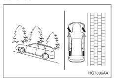
When parking on a hill, always turn the steering wheel. When the vehicle is headed up the hill, the
