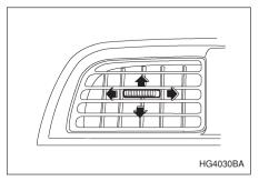
Move the tab up and down or right and left to adjust the flow direction
