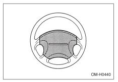
To sound the horn, push the horn pad.
