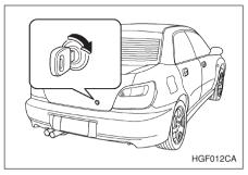
To open the trunk lid from outside, insert the key and turn it clockwise. To close the trunk lid, lightly press the trunk lid down until the latch engages.
