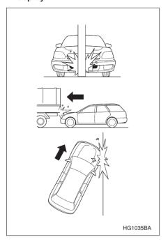
There are many types of collisions which might not necessarily require SRS frontal airbag deployment. If the vehicle strikes an object, such as a telephone pole or sign pole, or if it slides under a truck's load bed, or if it sustains an oblique offset frontal impact, the SRS frontal airbag may not deploy depending on the level of accident forces involved
