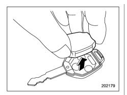
2. Remove the transmitter case from the key head.
