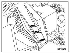
5. To install the air cleaner case (rear), insert the three projections on the air
