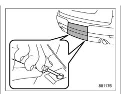
1. Remove the 2 clips from the bottom of the cover.
