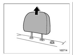
Raise the head restraint to the extended position. If the booster seat still makes contact, remove the head restraint. For details, refer to "Head restraints" \*P47.
