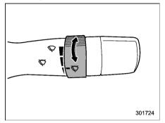
When the wiper switch is in the "\overline"" position, turn the dial to adjust the operating interval of the wiper. The operating interval can be adjusted in several steps from the shortest interval to the longest.
