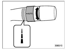
Turn the dial to adjust the sensitivity of the rain/light sensor for wiper control. Turn the dial downward to increase the sensitivity. Turn the dial upward to decrease the sensitivity.
