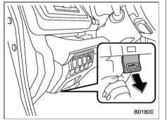
2. Pull the hood release knob under the instrument panel.
