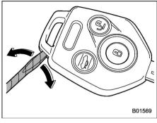
1. Wrap a flat-head screwdriver with vinyl tape or a cloth. Open the key head using a flat-head screwdriver.
