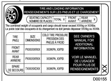
The vehicle placard shows original tire size, recommended cold tire inflation pressure on each tire at maximum loaded vehicle weight. seating capacity and loading information
