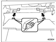
(4) Pull out the glove box horizontally and remove the hinge portion. When doing this, be careful not to damage the hinge.
