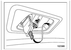
3. With the belt held by hand, allow the retractor to roll up the belt slowly. You should hold the webbing end and guide it back into the retractor while it is rolling up. Neatly store the tongue plate in the recess on the ceiling and then insert the tongue plate and anchor tongue plate into the slot as shown in the illustration.
