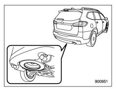
The spare tire is stored in the spare tire holder located under the cargo area.
