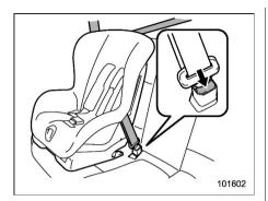
12. To remove the child restraint system, press the release button on the seatbelt buckle and allow the belt to retract completely. The belt will return to the ELR mode.
