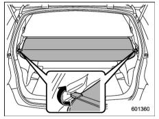
To extend the cover, pull the end of the cover out of the housing, then insert its hooks into the catches as shown. To rewind it, unhook it from the catches and it will rewind automatically. You should hold on to the cover and quide it back into the cover housing while it is rewinding.
