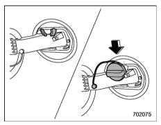
6. Set the fuel filler cap on the cap holder inside the fuel filler lid.
