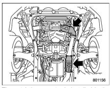
The catalytic converter is installed in the exhaust system. It serves as a catalyst to reduce HC, CO and NOx in exhaust gases, thus providing cleaner exhaust.
