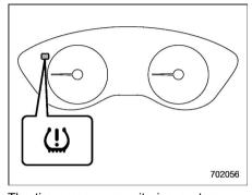
The tire pressure monitoring system provides the driver with the warning message indicated by sending a signal from a sensor that is installed in each wheel when tire pressure is severely low.
