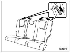
Pull the strap up and adjust the seatback to the desired position. Then release the strap and make sure the seatback is securely locked into place.
