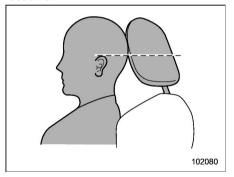
Each head restraint should be adjusted so that the center of the head restraint is closest to the top of the occupant's ears.
