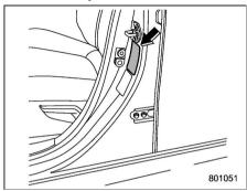
The vehicle placard is attached to the driver's side door pillar.
