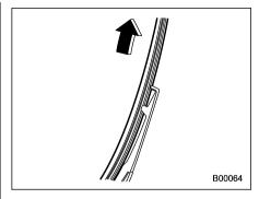
2. Pull the blade rubber assembly out of the plastic support.
