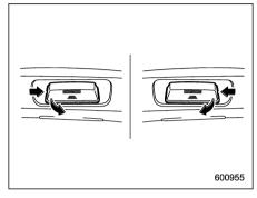
1. The license plate lights must be pushed inside, and then pulled out to be removed.
