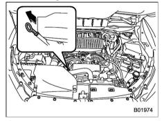
3. Be sure the level gauge is correctly inserted until it stops.
