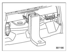
Hitch harness connector (4-pin type)
