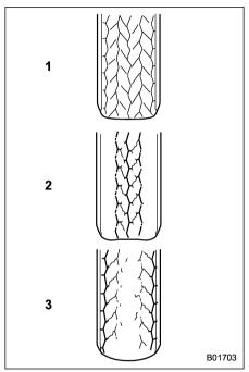
1) Correct tire pressure (tread worn evenly) Roadholding is good, and steering is responsive. Rolling resistance is low, so fuel consumption is also lower.
