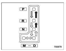
With the brake pedal depressed, shift while pressing the select lever button in
