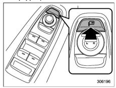
The power folding mirror switch operates only when the ignition switch is in the "ON" or "ACC" position.
