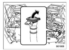
Remove the washer tank filler cap, then add windshield washer fluid.
