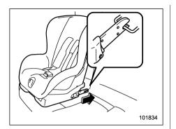
6. While following the instructions supplied by the child restraint system manufacturer, connect the lower hooks onto the lower anchorages located at "©" marks on the bottom of the rear seatback. When the hooks are connected, make sure the adjacent seatbelts are not caught.
