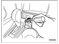
2. Wrap the tip of a flat-head screwdriver with vinvl tape or a cloth and use it to remove the shift lock cover. The shift lock release button is located under the shift lock cover.
