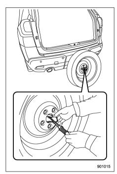
9. Tilt up the spare tire, then remove the tire retainer as showing in the figure.
