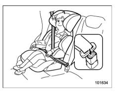
7. To remove the booster seat/cushion, press the release button on the seatbelt buckle and allow the belt to retract.
