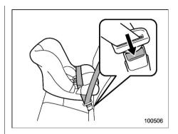
10. To remove the child restraint system, press the release button on the seatbelt buckle and allow the belt to retract completely. The belt will return to the ELR mode.
