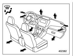
Heat-def: Windshield defroster outlets. foot outlets and both side outlets of the instrument panel (Refer to "Defrosting" @P280.)
