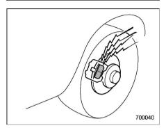
The disc brakes have audible wear indicators on the brake pads. If the brake pads wear close to their service limit, the wear indicator makes a very audible scraping noise when the brake pedal is applied.
