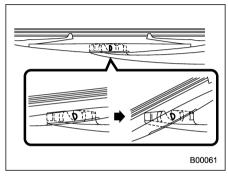
2. Turn the wiper blade assembly counterclockwise.
