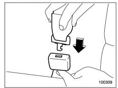
3. After confirming that the webbing is not twisted, insert the anchor tongue plate attached at the webbing end into the buckle on the right-hand side until a click
