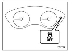
When the switch is pressed with the ignition switch in the "ON" position, the Vehicle Dynamics Control OFF indicator light "3" on the combination meter illuminates. The Vehicle Dynamics Control system will be deactivated and the vehicle will behave like a model not equipped with the Vehicle Dynamics Control system. When the switch is pressed again to reactivate the Vehicle Dynamics Control system, the Vehicle Dynamics Control OFF indicator light turns off.
