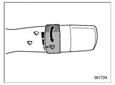
When the wiper switch is in the "\overline{\sigma}" position, turn the dial to adjust the operating interval of the wiper. The operating interval can be adjusted in several steps from the shortest interval to the longest.
