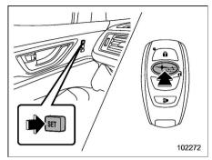
2. While holding the access key fob and pressing the "SET" button, press the "a" button of the access key fob.
