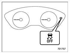
When the switch is pressed with the ignition switch in the "ON" position, the Vehicle Dynamics Control OFF indicator light "3" on the combination meter illuminates. The Vehicle Dynamics Control system will be deactivated and the vehicle will behave like a model not equipped with the Vehicle Dynamics Control system. When the switch is pressed again to reactivate the Vehicle Dynamics Control system, the Vehicle Dynamics Control OFF indicator light turns off.
