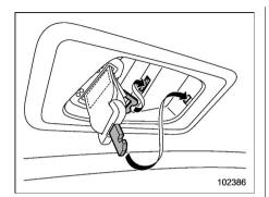
3. With the belt held by hand, allow the retractor to roll up the belt slowly. You should hold the webbing end and guide it back into the retractor while it is rolling up. Neatly store the tongue plate in the recess on the ceiling and then insert the tongue plate and connector (tongue) plate into the slot as shown in the illustration.
