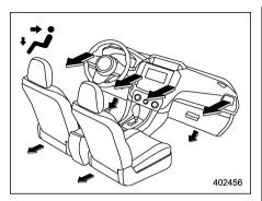
Ventilation 2: Instrument panel outlets and foot outlets
