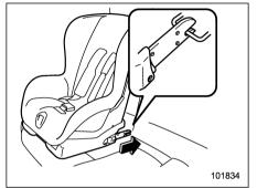
5. While following the instructions supplied by the child restraint system manufacturer, connect the lower hooks onto the lower anchorages located at "©" marks on the bottom of the rear seatback. When the hooks are connected, make sure the adjacent seatbelts are not caught.
