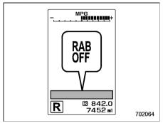
After the brake pedal is depressed, the Reverse Automatic Braking system OFF indicator will illuminate and the system will temporarily stop operating. The Reverse Automatic Braking system OFF indicator will turn off when the select lever is shifted. to a position other than the "R" position.
