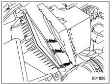
5. To install the air cleaner case (rear), insert the three projections on the air cleaner case (rear) into the slits on the air cleaner case (front).
