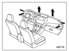
Select the "\(\vec{\psi}\)" or "\(\vec{\psi}\)" mode to defrost or dehumidify the windshield and front door windows
