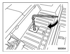
3. Turn the hoist shaft end clockwise with the wheel nut wrench to wind the cable up completely until you hear a few clicking sounds. Confirm that the temporary spare tire holding cable has been wound up completely by shaking the temporary tire.
