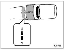
Turn the dial to adjust the sensitivity of the rain/light sensor for wiper control. Turn the dial downward to increase the sensitivity. Turn the dial upward to decrease the sensitivity.
