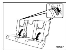
4. While pulling the straps, fold down the seatbacks.
