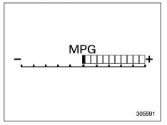
The ECO gauge shows the difference between the current rate of fuel consumption and the average rate of fuel consumption since the trip meter was last reset.
