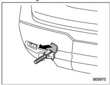
2. Cover the tip of a flat-head screwdriver with vinyl tape or cloth so that it will not scratch the bumper. Pry off the cover on the rear bumper using a screwdriver, and you will find a threaded hole for attaching the towing hook.
