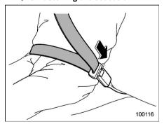
1. Push the release button of the center seatbelt buckle (on the left-hand side) to
