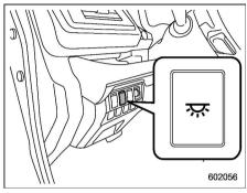
Push the One-touch Interior Illumination switch once to illuminate the map light (if the map light switch is in the "DOOR" position) and reading light.
