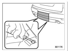
1. Remove the 2 clips from the bottom of the cover.
