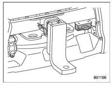
Hitch harness connector (4-pin type)
