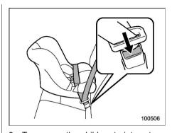
To remove the child restraint system, press the release button on the seatbelt buckle and allow the belt to retract completely. The belt will return to the ELR mode.
