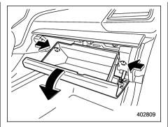
(3) Push in the stoppers located on both sides of the glove box and then pull down the glove box as far as it will go.
