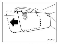
With the sun visor positioned over the side window, you can slide the sun visor toward the rear to prevent glare through the gap between the sun visor and center pillar. To slide the sun visor, pull it toward the rear of the vehicle. When you have finished sliding it, push it toward the front of the vehicle.
