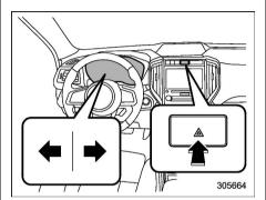
The hazard warning flasher is used to warn other drivers when you have to park your vehicle under emergency conditions. The hazard warning flasher works regardless of the position of the ignition switch.
