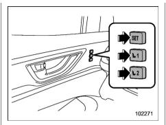
2. While pressing the "SET" button, press and hold the desired button "1" or "2".
