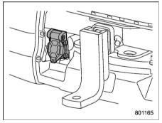
Hitch harness connector (7-pin type)
