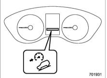
This indicator appears while the hill descent control function is in the standby mode. It flashes while the function is operating. It will disappear when the function is in the disabled mode. When this function is changed from operational to non-operational, it will disappear when the vehicle speed reaches more than approximately 18 mph (30 km/h).
