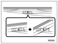
2. Turn the wiper blade assembly counterclockwise.
