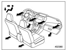
Bi-level: Instrument panel outlets and foot outlets
