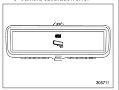
When the camera calibration error, the warning indicators will appear as shown in the illustration.
