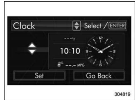
4. Select "Type A clock", "Type B clock", "Calendar" or "Off" by operating the "▼" switch. Then push the **ENTER** button.
