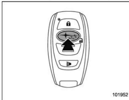
2. Unlock the driver’s door by pressing the “
