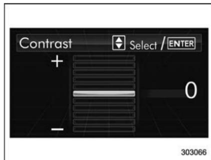
3. Select a contrast level by operating the “▲” or “▼” switch, and confirm the setting by pushing the **ENTER** button.
