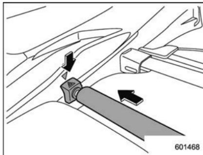
1. Align the right side of the front cover with the triangle mark before fixing the cover in place.
