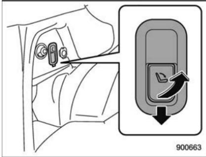
2. After pushing the rear seat release latch down once, remove the latch.
