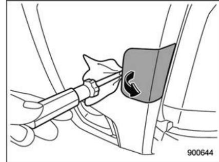
2. Cover the tip of a flat-head screwdriver with vinyl tape or cloth so that it will not scratch the bumper. Insert the flat-head screwdriver into the cutout of the cover and pry open the cover.
