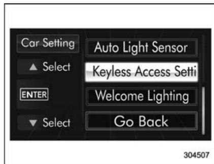
2. Operate the "▲" or "▼" switch to select the "Keyless Access Setting" item. Then push the **ENTER** button.
