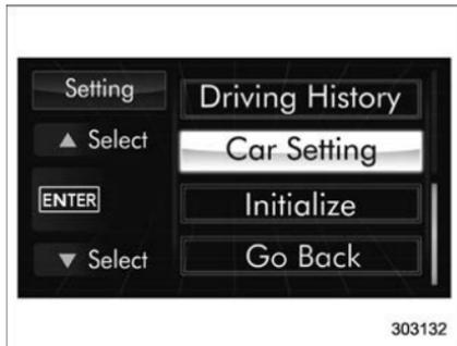
3. After the selection screen is displayed, operate the “▲” or “▼” switch to show the “Car Setting” item. Then, push the **ENTER** button.
