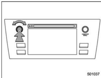
Press the power/VOLUME knob to turn the audio/visual system on and off. When the system turns on, the mode that was in use the last time the system was turned off will be displayed. Press and hold the knob to turn the display off.
