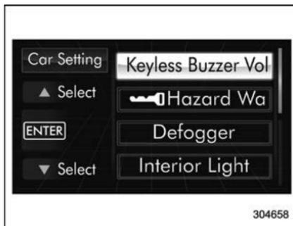
2. Operate the “▲” or “▼” switch to select the “Keyless Buzzer Volume” item. Then push the **ENTER** button.
