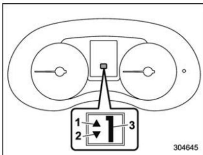
**Select lever/gear position indicator (type B)**
