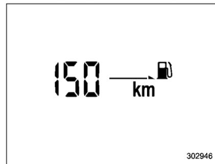
The driving range indicates the distance that can be driven taking into account the amount of fuel remaining in the tank and
