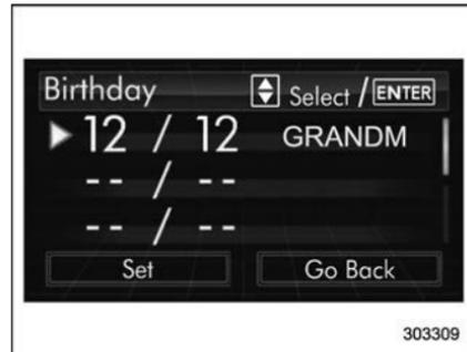
3. Select an entry in the list to set by operating the “▲” or “▼” switch. Then push the **ENTER** button.
