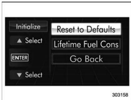
2. Operate the “▲” or “▼” switch to select the “Reset to Defaults” item. Then push the **ENTER** button.
