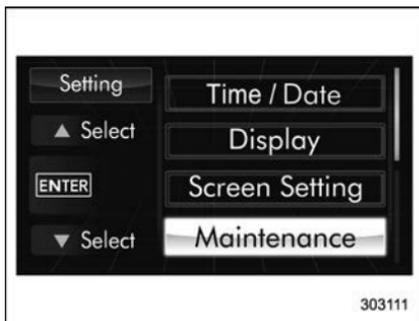
3. After the selection screen is displayed, operate the “▲” or “▼” switch to show the “Maintenance” item. Then, push the **ENTER** button.
