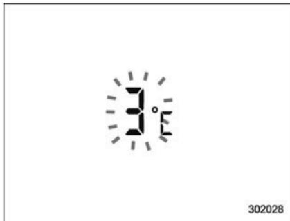
When the outside temperature drops to 37°F (3°C) or lower, the temperature indication flashes to show that the road surface may be frozen.
