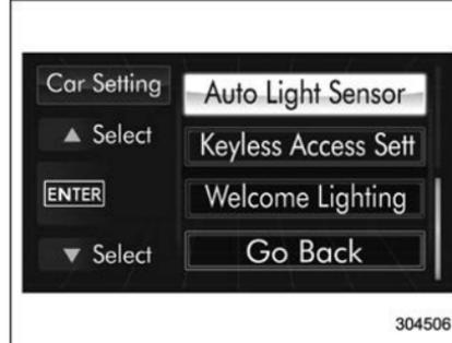
2. Operate the "▲" or "▼" switch to select the "Auto Light Sensor" item. Then push the ENTER button.
