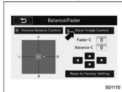
2. Adjust the balance by pressing “◀” or “▶” key.
