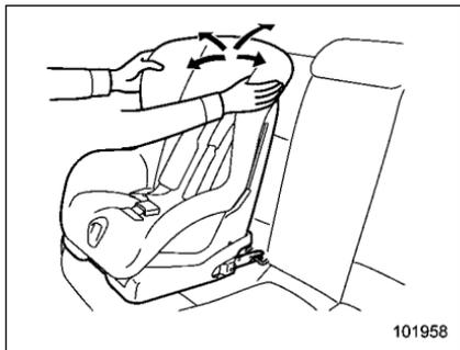
8. Before seating a child in the child restraint system, try to move it back and forth and right and left to verify that it is held securely in position.
