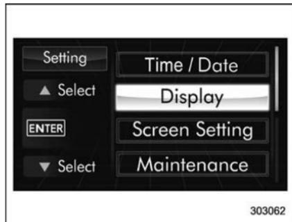
3. After the selection screen is displayed, operate the “▲” or “▼” switch to show the “Display” item. Then, push the **ENTER** button.
