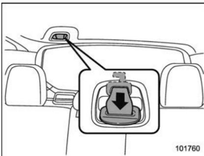
Rear center seatbelt is stowed in the recess of the ceiling above the cargo area.
