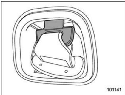
3. Allow the retractor to roll up the belt.
