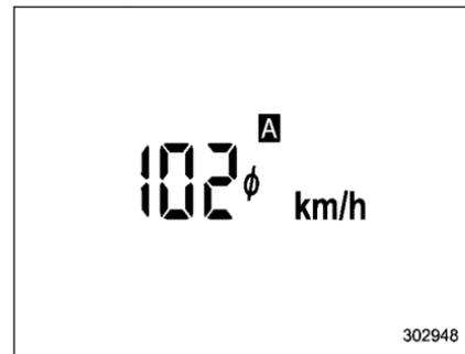
This display shows the average vehicle speed since the trip meter was last reset.
