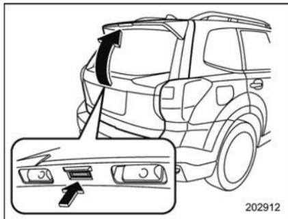
1. Press and hold the rear gate opener button. If the rear gate does not open, perform the procedure described in “Rear gate – if the rear gate cannot be opened” 9-18.
