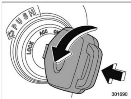
The key can be turned from the “ACC” to “LOCK” position only when the select lever is in the “P” position (CVT models) and the key is pushed in while turning it (all models).
