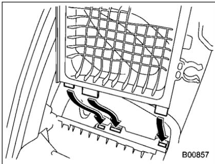
4. To install the air cleaner case (rear), insert the three projections on the air cleaner case (rear) into the slits on the air cleaner case (front).
