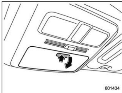
To open the console, push on the console lid lightly. The lid will automatically open.
