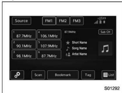
1. Touch the “Sub CH” key on the control screen and the following screen will be displayed.
