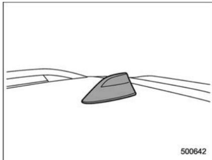
The roof antenna is installed in the center of the roof at the rear.
