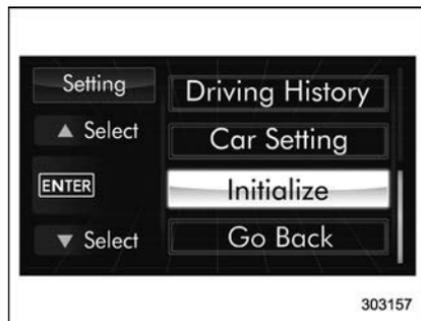
3. After the selection screen is displayed, operate the “▲” or “▼” switch to show the “Initialize” item. Then, push the **ENTER** button.
