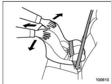
6. Push and pull the child restraint system forward and from side to side to check if it is firmly secured. Sometimes a child restraint can be more firmly secured by pushing it down into the seat cushion and then tightening the seatbelt.
