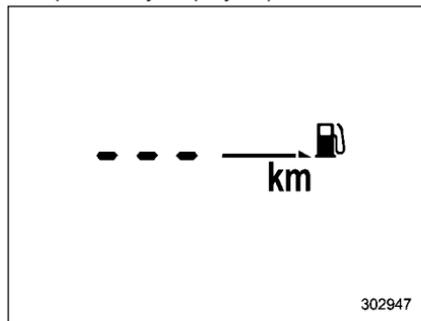
If the driving range is shown as “---”, there is only a tiny amount of fuel left in the tank. You must refuel the vehicle immediately.
