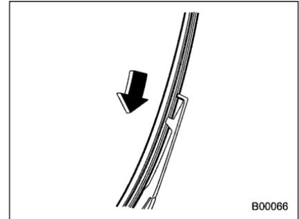
4. Align the claws of the plastic support with the grooves in the blade rubber assembly, then slide the blade rubber assembly into place.
