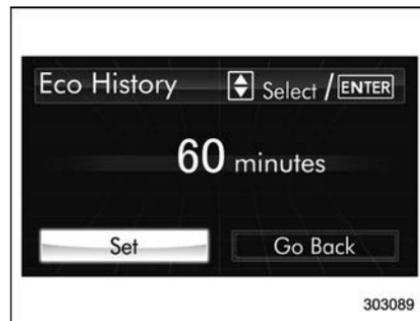
6. Select “Set” by operating the “▲” switch and confirm the setting by pushing the **ENTER** button.
