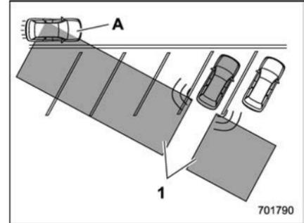
1) The detection range of the radar sensors
