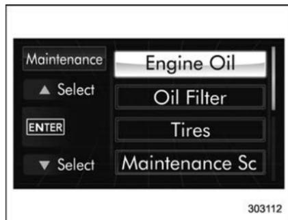
2. Operate the “▲” or “▼” switch to select the “Engine Oil” item. Then push the **ENTER** button.
