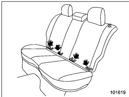
The lower anchorages (bars) are provided for installing a child restraint system only
