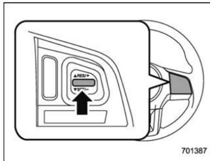
To resume the cruise control after it has been temporarily canceled and with vehicle speed of approximately 20 mph (30 km/h) or more, press the “RES/SET” switch to the “RES” side to return to the original cruising speed automatically.
