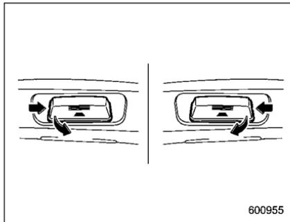
1. License plate light must be pushed inwards, then pulled out to be removed.
