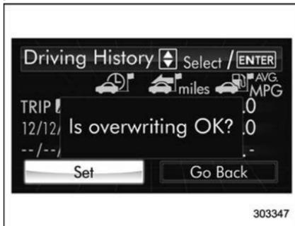
7. To overwrite the previous registration, push the **ENTER** button. When registration is performed the first time, it is registered
