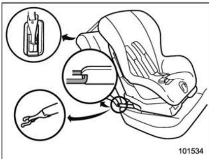
Some types of child restraint systems can be installed on the rear seat of your vehicle without use of the seatbelts. Such child restraint systems are secured to the designated anchorages provided on the vehicle body. The lower and tether anchorages are sometimes referred to as the LATCH system (Lower Anchors and Tethers for CHildren).
