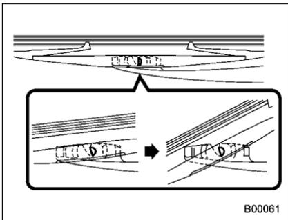
2. Turn the wiper blade assembly counterclockwise.
