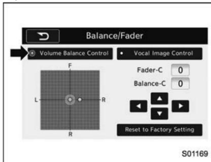
2. Adjust the balance by pressing “◀” or “▶” key.
