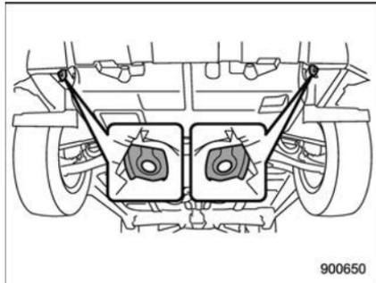
The front tie-down hooks are located between each of the front tires and the
