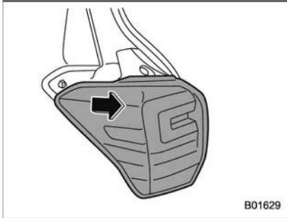
2. Slide the rear combination light assembly rearward and remove it from the vehicle.
