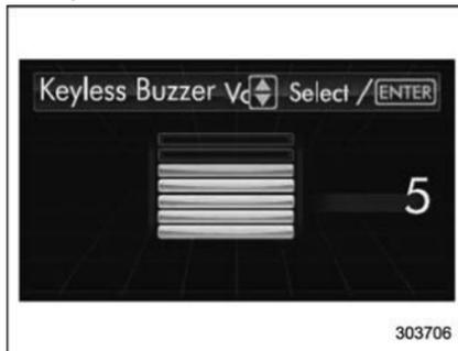
3. Select a volume level by operating the “▲” or “▼” switch, and confirm the setting by pushing the **ENTER** button.
