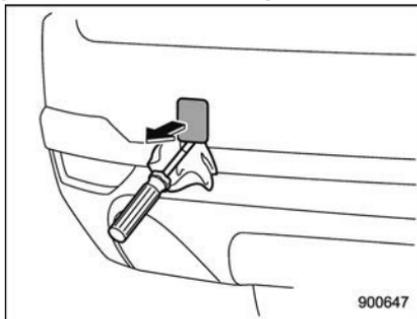
2. Pry off the cover on the rear bumper using a screwdriver, and you will find a
