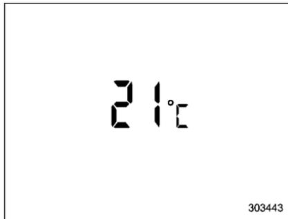
This indicator displays the outside temperature between -40°F (-40°C) and 122°F (50°C).
