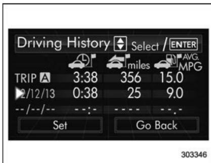
6. Select one of the registration lines by operating the “▲” or “▼” switch. Then push the **ENTER** button.
