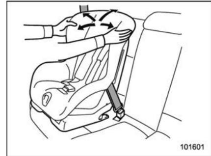
9. Before having a child sit in the child restraint system, try to move it back and forth and right and left to check if it is firmly secured. Sometimes a child restraint can be more firmly secured by pushing it down into the seat cushion and then tightening the seatbelt.
