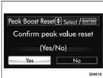
2. Select “Yes” by operating the “▼” switch, and confirm the resetting by pushing the **ENTER** button.
