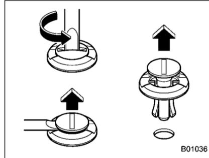
1. Turn the clips counterclockwise using a flat-head screwdriver until the center portion of the clip is raised.
