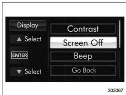
2. Operate the “▲” or “▼” switch to select the “Screen Off” item. Then push the **ENTER** button.
