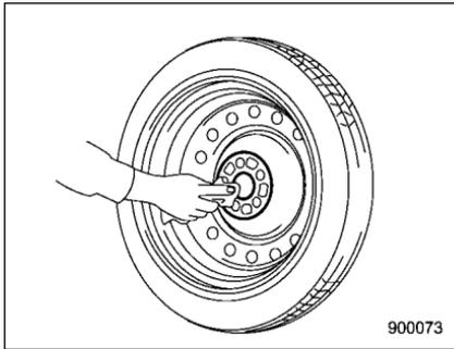
12. Before putting the spare tire on, clean the mounting surface of the wheel and hub with a cloth.
