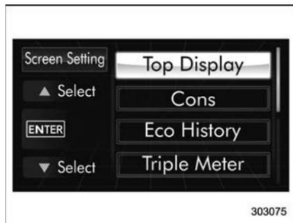
2. Operate the “▲” or “▼” switch to select the “Top Display” item. Then push the **ENTER** button.
