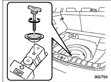
16. Store the flat tire in the spare tire compartment. Be sure to place the spacer in the manner shown in the illustration, and then tighten the bolt in the front side of the bracket.
