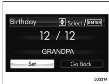
8. After entering the name by repeating step 7, select "Set" by operating the "▼" switch and confirm the setting by pushing the **ENTER** button.
