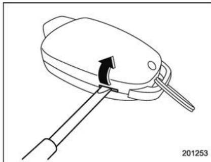
2. Carefully pry the remote engine start transmitter halves apart using a small flat-head screwdriver.
