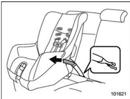
6. [If your child restraint system is of a flexible attachment type (which uses tether belts to connect the child restraint system properly to the lower anchorages)] While pushing the child restraint into the seat cushion, pull both left and right lower tether belts up to secure the child restraint system firmly by taking up the slack in the belt.
