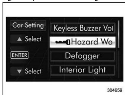
2. Operate the "▲" or "▼" switch to select the "Hazard Warning Flasher" item. Then push the **ENTER** button.
