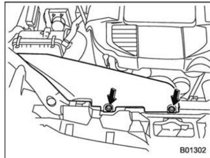
To replace the right side headlight bulb, use a screwdriver to undo the clips on the air intake duct, then remove the air intake duct.
