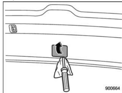
1. Remove the access cover at the bottom-center of the rear gate trim using a flat-head screwdriver wrapped with vinyl tape or a cloth.
