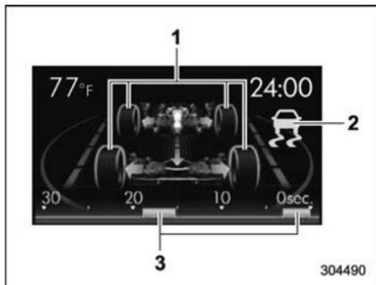
When the Vehicle Dynamics Control system has been activated: the tires remain illuminated in yellow while the Vehicle Dynamics Control System is activated.
