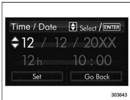
4. Select a number by operating the “▲” or “▼” switch. Then push the **ENTER** button. When “12 h” is selected, the clock will be set to a 12-hour display. When “24 h” is selected, the clock will be set to a 24-hour display.
