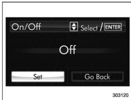
5. Select “Set” by operating the “▼” switch, and confirm the setting by pushing the **ENTER** button.
