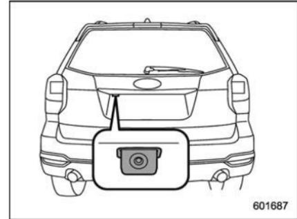
A rear view camera is attached to the rear gate. When the ignition switch is "ON" and the shift lever (MT models) or select lever (CVT models) is set to "R", the rear view camera automatically displays the rear view image behind the vehicle on the monitor of the navigation system or the audio display.
