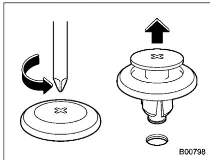
1. Turn the clip counterclockwise using a Phillips screwdriver until the center portion of the clip is raised.
