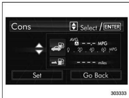
4. Select the displayed configuration by operating the “▲” or “▼” switch. Then push the **ENTER** button.
