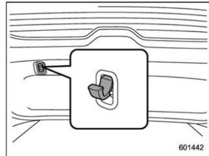
A convenient hook is attached to the rear gate trim. When the rear gate is open, you can hang a candle lantern, wet suit, etc. on the hook.
