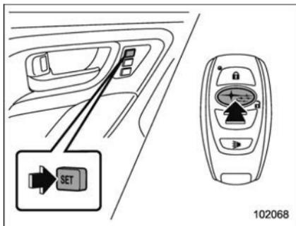
2. While holding the access key and pressing the “SET” button, press the “
