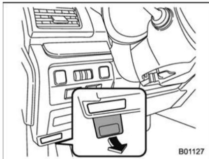
2. Pull the hood release knob under the instrument panel.
