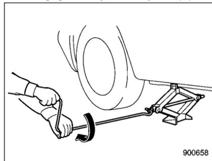
10. Insert the jack handle into the jackscrew, and turn the handle until the tire clears the ground. Do not raise the vehicle higher than necessary.
