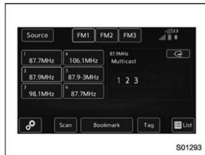
2. The indication that shows whether the current broadcast is digital or analog is displayed on the top right of the control screen.
