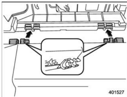
4. Reinstall the glove box, and connect the damper shaft.
