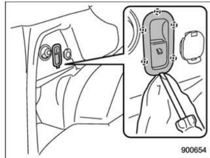
1. Release the fitting on the left side rear seat release latch.
