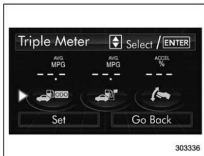
3. Select the setting location (left, center or right) by operating the "▼" or "▲" switch. Then push the **ENTER** button.
