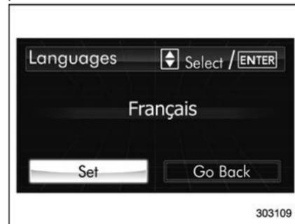
5. Select “Set” by operating the “▼” switch and confirm the setting by pushing the **ENTER** button.
