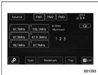
1. Touch the “Tag” key in the control screen while receiving HD Radio, the tag setting screen will be displayed.
