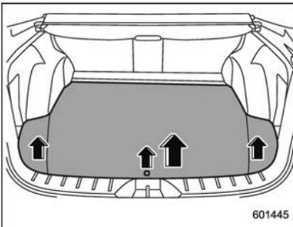
1. Pull the strap to open the center part of the cargo floor lid, and then remove the lid.
