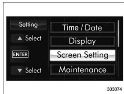
3. After the selection screen is displayed, operate the “▲” or “▼” switch to show the “Screen Setting” item. Then, push the **ENTER** button.
