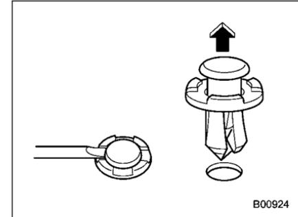
1. Pull out the center portion of the clip using a flat-head screwdriver as shown in the illustration.
