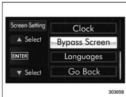
2. Operate the "▲" or "▼" switch to select the "Bypass Screen" item. Then push the **ENTER** button.
