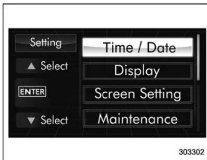
3. After the selection screen is displayed, operate the “▲” or “▼” switch to show the “Time/Date” item. Then, push the **ENTER** button.
