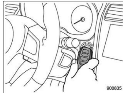
4. Hold the access key with the buttons facing you, and touch the push-button ignition switch with it.
