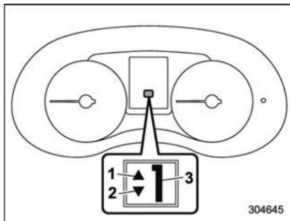
**Select lever/gear position indicator (type B)**
