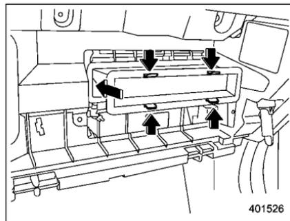
3. Replace the air filter element with a new one.
