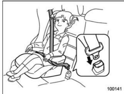
2. Place the booster seat in the rear seating position and sit the child on it. The child should sit well back on the booster seat.
