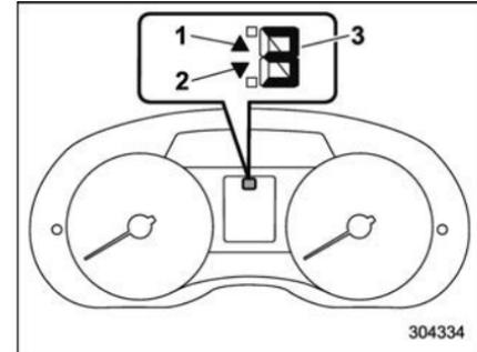
**Select lever/gear position indicator (type A)**
