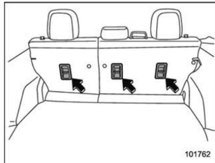
The tether anchorages (upper anchorages) are provided at the locations shown in the above illustration. For details, refer to "Top tether anchorages" 1-40.
