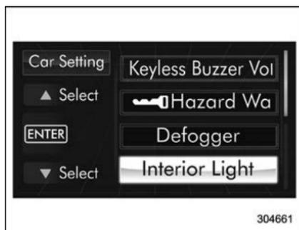
2. Operate the "▲" or "▼" switch to select the "Interior Light" item. Then push the ENTER button.
