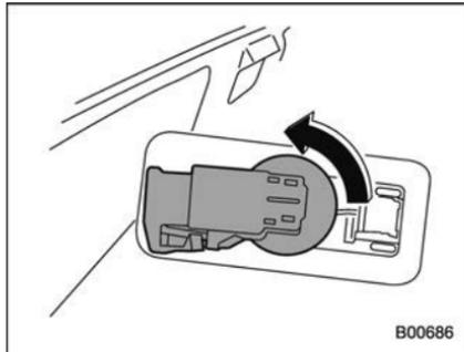
2. Turn the bulb socket counterclockwise and pull out the socket.
