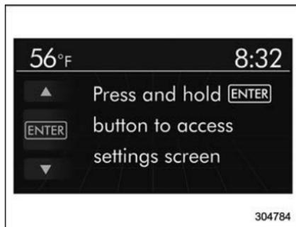
When the **ENTER** button is pushed and held, the selection screen can be displayed. The displayed contents can be set or customized from the selection screen. For details, refer to "Selection screen" 3-56.
