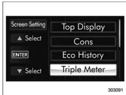
2. Operate the "▲" or "▼" switch to select the "Triple Meter" item. Then push the **ENTER** button.
