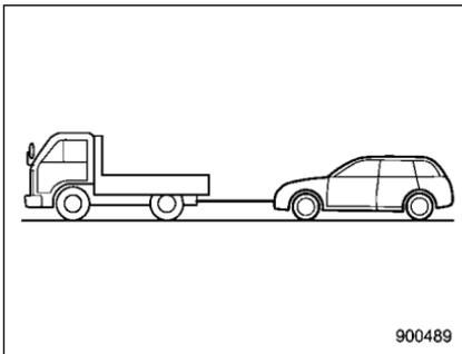
1. Release the parking brake and put the transmission in the "N"/neutral position.
