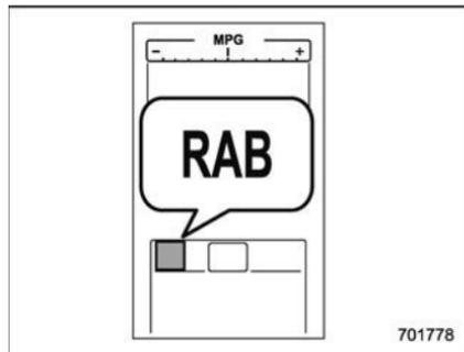
If the Reverse Automatic Braking System malfunctions, the above indicator illuminates in the combination meter. Contact the nearest SUBARU dealer for details.
