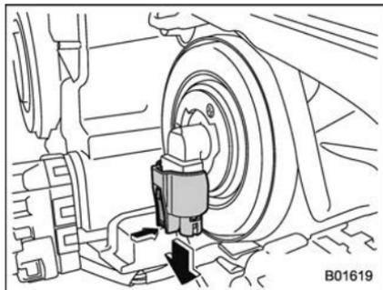
1. Disconnect the electrical connector from the bulb.
