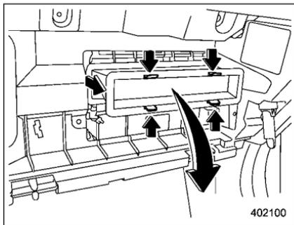
2. Remove the air filter according to the following procedure in order to prevent dust on the air cleaner from falling to the inside of its housing.
