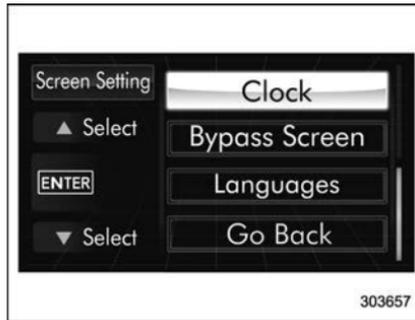
2. Operate the "▲" or "▼" switch to select the "Clock" item. Then push the **ENTER** button.
