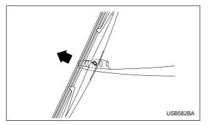
3. Having turned the wiper blade assembly to the angle shown in the illustration, pull it in the direction of the arrow to remove it from the wiper arm.
