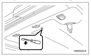
1. Remove the plug on the roof trim located to the rear of the moonroof by inserting the end of a flat-head screwdriver between the roof and plug and prying it off.
