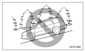
The Hill holder does not operate when the vehicle is facing downhill. And the Hill holder may not operate on slight grades.
