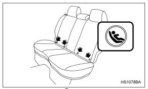
You will find marks " ( ) " at the bottom of the rear seat seatbacks. These marks indicate the positions of the lower anchorages (bars).
