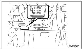
One is located under the instrument panel behind the coin tray on the driver's seat side.
