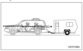
The self-leveling system is incorporated in the rear suspension shock absorber and operates only when the vehicle is in motion.
