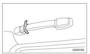
The coat hook is attached to the rear left passenger's hand grip.
