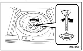
14. Store the flat tire in the spare tire compartment. Put the spacer and tighten the attaching bolt firmly. Also store the jack and wheel nut wrench in their stor-
