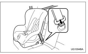
9. To remove the child restraint system, press the release button on the seatbelt buckle and allow the belt to retract completely. The belt will return to the ELR mode. Unhook the top tether hook from the top tether anchor.
