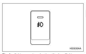
The fog lights operate only when the headlights are on low beam. Push the fog light button to turn the fog lights on.
