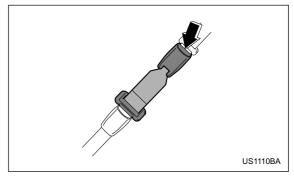
To connect the extender to the seatbelt, insert the tongue plate into the seatbelt buckle so that the "PRESS" signs on the buckle-release buttons of the extender and the seatbelt are both facing outward as shown in the diagram. You will hear a click when the tongue plate locks into the buckle.
