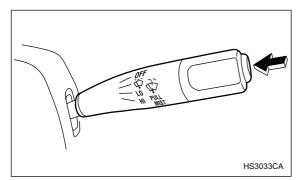
To wash the windshield, push the washer button at the end of the wiper control lever. The washer fluid sprays until you release the washer button. The wipers operate while you push the button.
