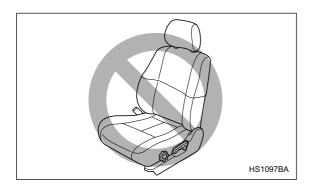
Do not put any kind of cover or clothes or other objects over either front seatback and do not attach labels or stickers to the front seat surface on or near the SRS side airbag. They could prevent proper deployment of the SRS side airbag, reducing protection available to the front seat's occupant.
