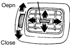
Move the thumb-wheel up and down or right and left to adjust the air flow direction
