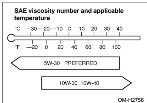
▼ **Recommended grade and viscosity under severe driving conditions**
