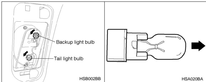
1. Remove the rear combination light cover by prying the edge of the cover with screwdriver.
