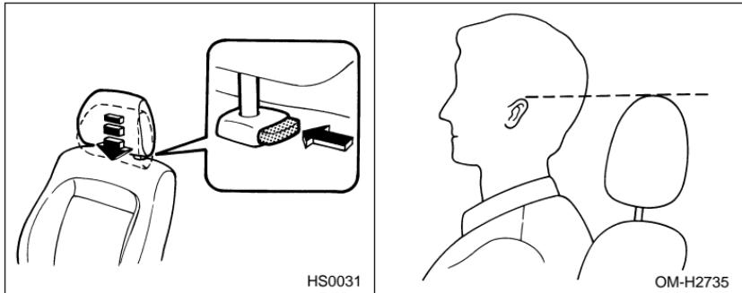
To raise the head restraint, pull it up. To lower it, push the head restraint down while pressing the release button on the top of the seat-back.
