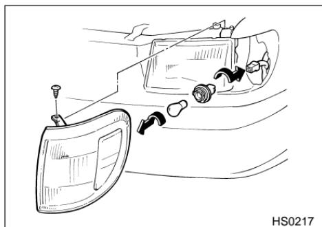
1. Remove the front turn signal light assembly mounting screw located at the top of the headlight assembly using a phillips screwdriver.
