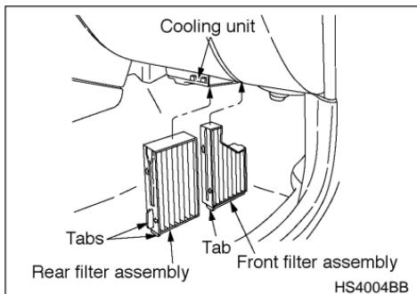
3. Insert the front filter assembly in the cooling unit, then install the rear filter assembly.
