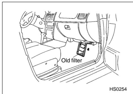
1. Remove the filter cover from the cooling unit by removing the two (2) clips with a blade screwdriver and unhooking the hinge. The screwdriver must be inserted into the top of the clip. Do not pry the middle on the clip.
