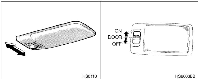
The interior light switch has three positions:
