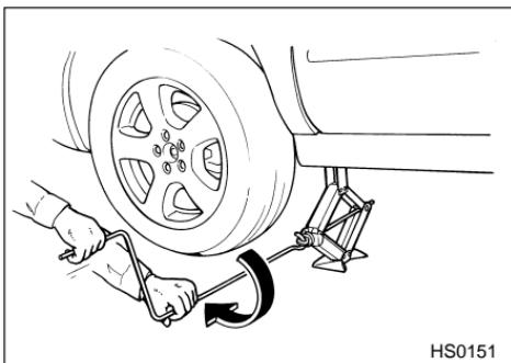
9. Remove the wheel nuts and the flat tire.
