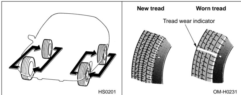
A tire should be replaced when the tread wear indicator appears as a solid band across the tread. The indicators appear when the remaining tread has been worn to 0.063 in (1.6 mm) or less.
