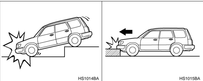
▽ **Examples of the types of accidents in which the SRS frontal airbag is unlikely to deploy.**
