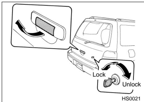
To unlock the rear gate, insert the key in the keyhole and turn it clockwise. To lock the rear gate, insert the key in the keyhole and turn it counterclockwise. Since your vehicle is equipped with power door locks, the rear gate can also be locked and unlocked by operating the driver's door lock.
