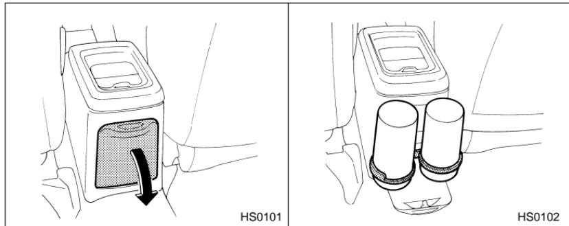
The rear passenger's cup holder is located at the back of the center
