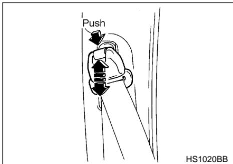
The shoulder belt anchor height should be adjusted to the position best suited for you. To adjust the shoulder belt anchor height, push the release button and slide the anchor down or up. Pull down on the anchor to make sure that it is locked in place.
