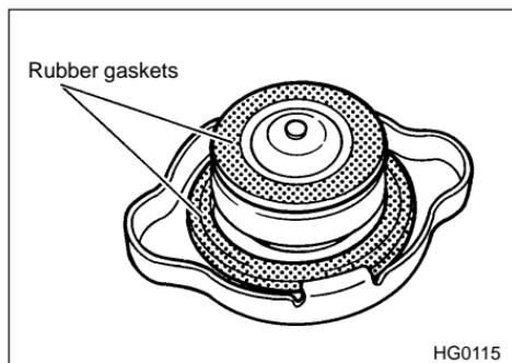
6. Put the radiator cap back on and tighten firmly. At this time, make sure that the rubber gaskets in the radiator cap are correctly in place.
