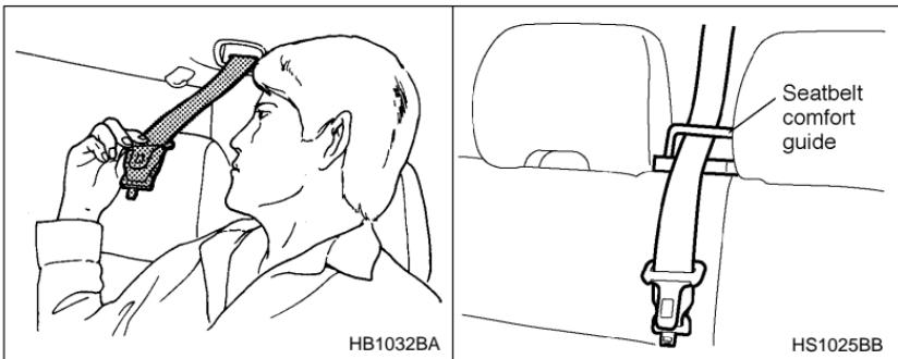
1. Pull out the seatbelt slowly from the overhead retractor, then pass the seatbelt through the seatbelt comfort guide located beside the
