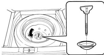
The spare tire is stored under the floor of the cargo area. To remove the spare tire, first open the spare tire cover and remove the storage tray, turn the attaching bolt counterclockwise, then take the spare tire out.
