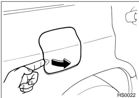
1. To open the fuel filler door, pull it outward. After refueling, be sure to close the fuel filler door completely.
