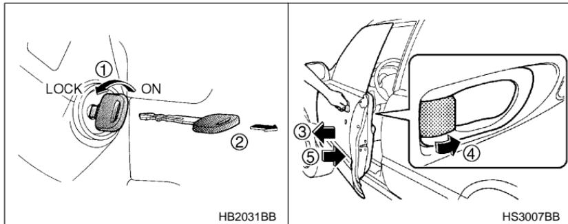
1. Turn the ignition switch to the “ON” position.
