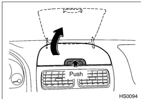
To open the dashboard compartment, push the button and pull up on the
