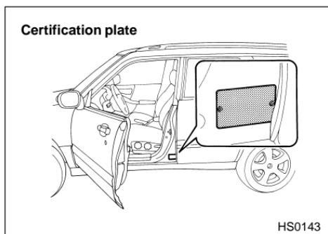
The certification plate attached to the driver's side door jamb shows GVWR (Gross Vehicle Weight Rating) and GAWR (Gross Axle Weight Rating).
