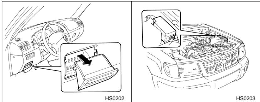
The fuses are designed to melt during an overload to prevent damage to the wiring harness and electrical equipment. The fuses are located in two fuse boxes.
