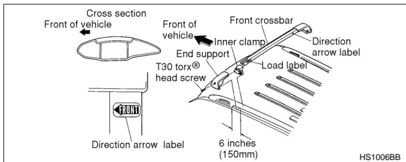
1. Before placing the crossbar on the roof rails, make sure that the T-30 torx® head screw is fully loosened from each end support.
