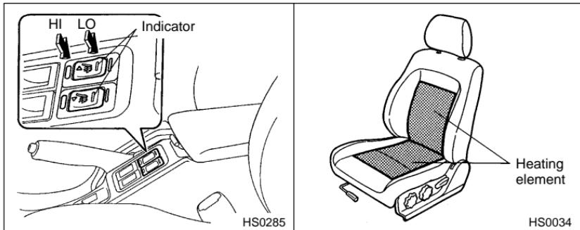
To turn on the seat heater, push the "LO" or "HI" position on the switch, as desired, depending on the temperature.
