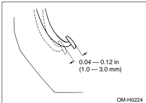
Stop the engine and firmly depress the brake pedal several times. Lightly press the brake pedal down with one finger to check the free play with a force of less than 10 N (2 lb, 1 kg).
