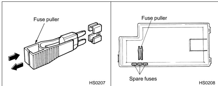
5. Pull out the fuse with the fuse puller provided in the main fuse box cover.
