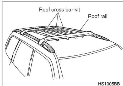
The roof rail is not designed to carry cargo by itself.
