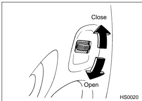
To open the window, push the switch down and hold it until the window reaches the desired position. To close the window, push the switch up and hold it until the window reaches the desired position.
