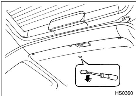
2. Remove the plug on the roof trim located to the rear of the moonroof by inserting the end of the regular screwdriver between the roof and plug and prying it off.
