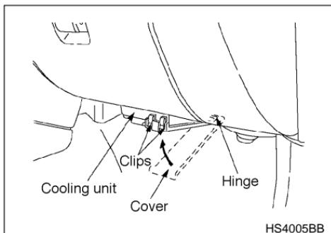
4. Reinstall the cover and secure it using the clips.
