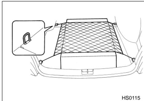
The cargo area is equipped with four anchorage eyelets so that cargo can be secured with a cargo net or ropes.
