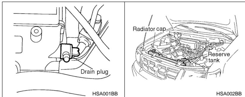
3. Loosen the radiator cap to drain the coolant from the radiator. Then drain the coolant from the reserve tank. Tighten the drain plug securely.
