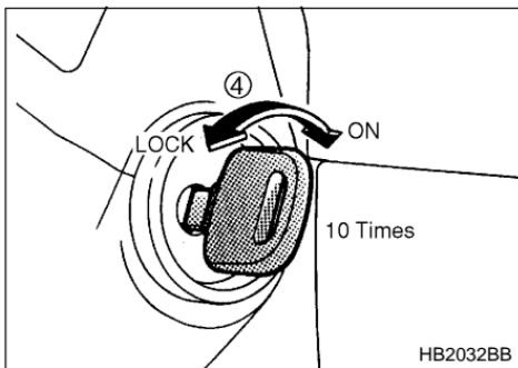
4. Place the ignition key into the ignition switch and cycle the switch from LOCK to ON ten times **within 15 seconds**. Be sure to stop at the LOCK position **and leave the key in the ignition**. The horn will sound once to indicate that you are in the transmitter programming mode.
