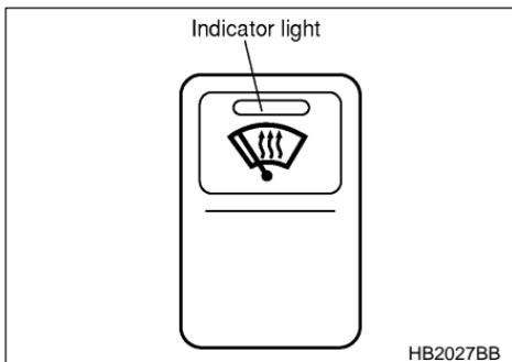
Before turning on the windshield wiper deicer, remove any snow from the windshield. To turn on the windshield wiper deicer, push the switch. The indicator light located on the switch lights up while the windshield wiper deicer is operating.
