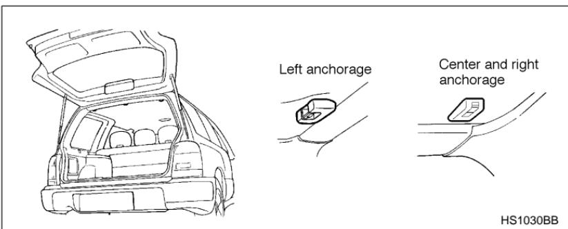
Three anchor brackets, i.e., ones for the right, center and left positions, are already installed on the rear edge of the roof.
