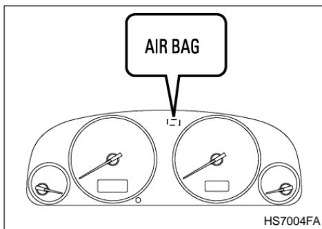
A diagnostic system continually monitors the readiness of the SRS airbag system while the vehicle is being driven. The SRS airbag system warning light "AIRBAG" will show normal system operation by lighting for about 6 seconds when the ignition key is turned to the "ON" position.
