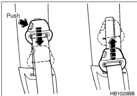
The shoulder belt anchor height should be adjusted to the position best suited for you. To lower the anchor height, push the release button and slide the anchor down. To raise the anchor height, slide the anchor up. Pull down on the anchor to make sure that it is locked in place.
