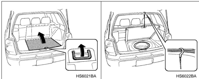
To open the lid, pull the handle up. To keep the lid open, hang the hook provided on the backside of the lid on the rear edge of the roof. The spare tire is stored under the storage tray.
