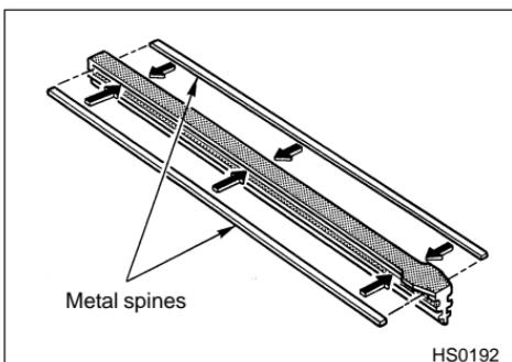
5. Align the claws of the metal support with the grooves in the rubber and slide the blade rubber assembly into the metal support until it locks. Be sure to position the claws at the end of the metal support between the stoppers on the rubber as shown. If the rubber is not retained properly, the wiper blade may scratch the windshield.
