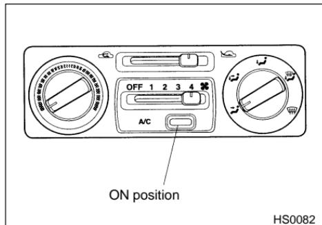
For cooling and dehumidification of the passenger compartment, air flows through the instrument panel outlets:
