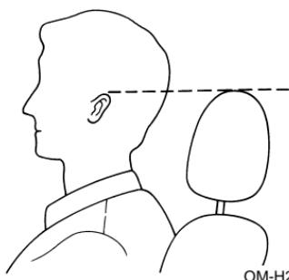
To raise the head rest, pull it up. To lower it, push the head rest down while depressing the release button on the top of the seatback.
