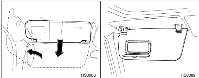
To block out glare, swing down the visors. To use the sun visor at a side window, swing it down and move it sideways.
