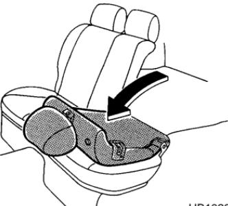
Unlock the seatback by pulling the release knob and then fold the seatback down.
