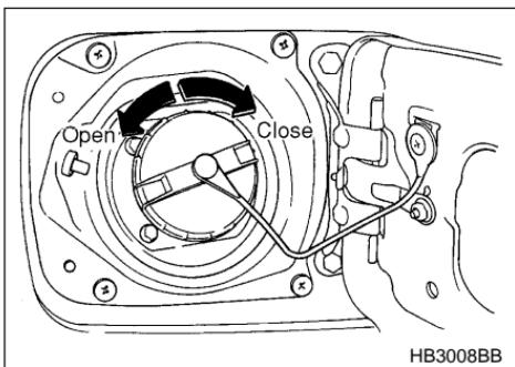
2. To take off the fuel filler cap, turn it slowly counterclockwise and remove the cap.
