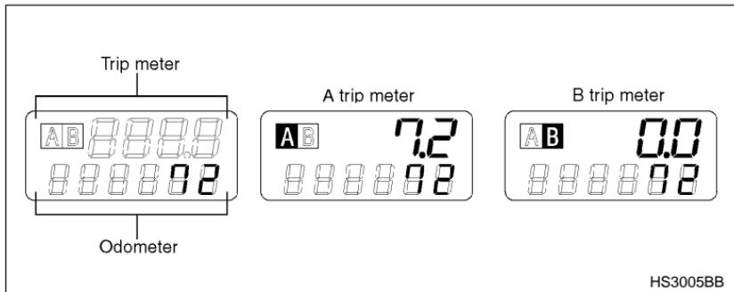
This meter displays the odometer and two trip meters when the ignition
