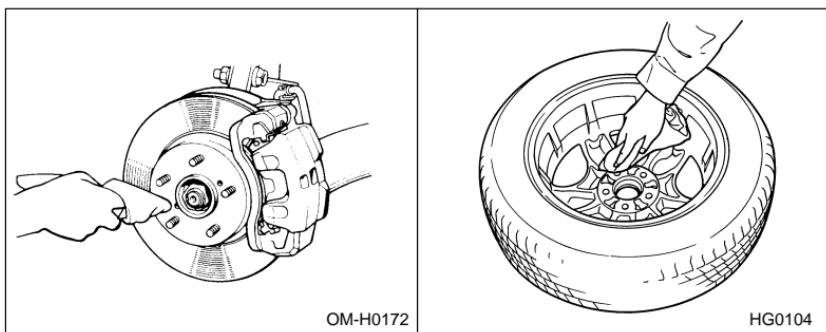
11. Put on the spare tire. Replace the wheel nuts. Tighten them by hand.
