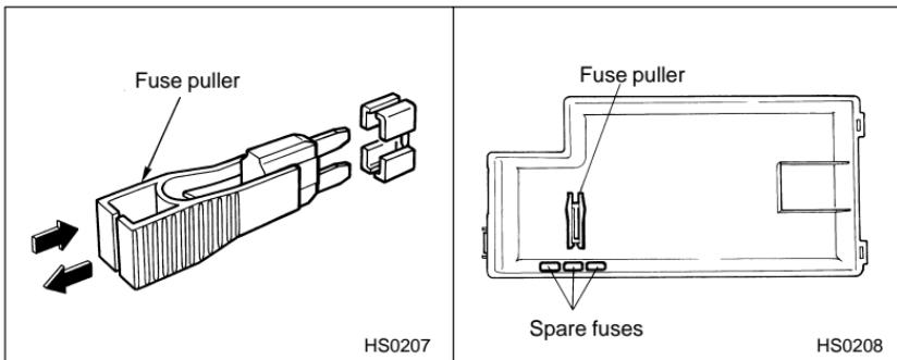
4. Pull out the fuse with the fuse puller. The fuse puller is stored in the
