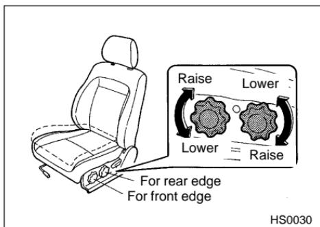
Turn either dial to adjust the angle and height of the seat cushion to the desired position.
