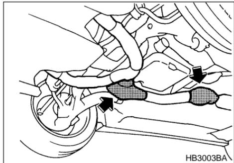
The catalytic converter is installed in the exhaust system. It serves as a catalyst to reduce HC, CO and NOx in exhaust gases, thus providing cleaner exhaust.
