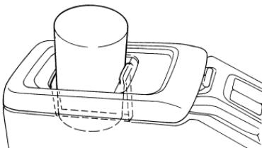
A front passenger's cup holder is also built in the lid of the center console. To use the cup holder, open the lid by sliding it forward and unfold the arm. Adjust the opening area by sliding the lid forward or rearward to fit the cup. When not in use, fold the arm and close the lid.
