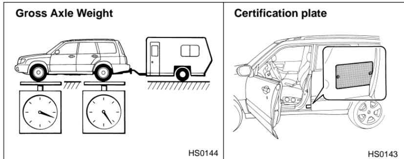
To check both GVWR and GAWR and to confirm that the total weight and weight distribution are within safe driving limits, you should have your vehicle and trailer weighed at a commercial weighing station.
