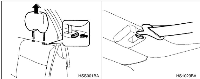
1. Remove the head rest at the seat position where the child restraint has been installed with the seatbelt: lift up the head rest while pressing the release button. Store the head rest in the cargo area. Avoid placing the head rest in the passenger compartment to prevent it from being thrown around in the passenger compartment in a sudden stop or a sharp turn.
