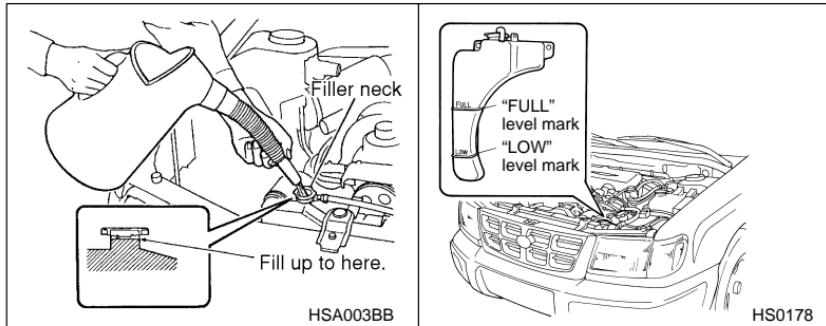
5. Slowly pour the coolant and fill to the radiator filler neck and to the reserve tank's "FULL" level mark. Do not pour the coolant too quickly, as this may lead to insufficient air bleeding and trapped air in the system.
