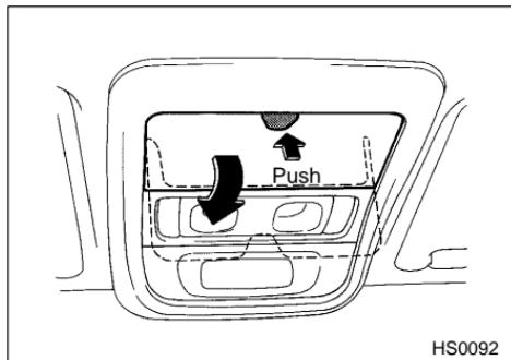
To open the console, push the button and the console lid will automatically open.
