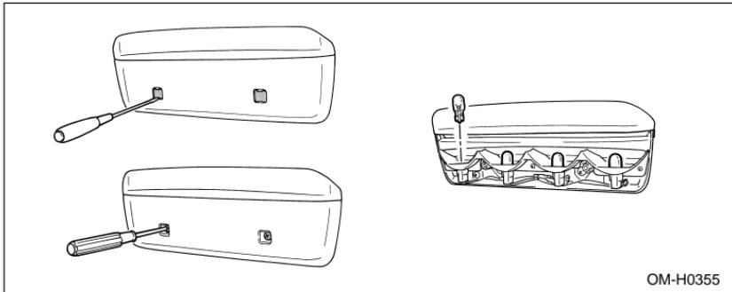
1. Remove the mounting screw covers by prying on the edge with a screwdriver.
