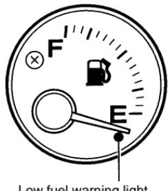
The fuel gauge shows the approximate amount of fuel remaining in the tank.
