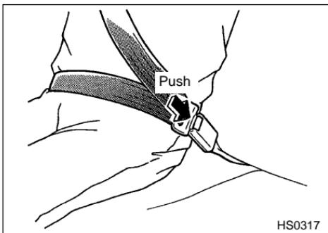
Push the release button of the center seatbelt buckle (on the left-hand side) to unfasten the seatbelt.
