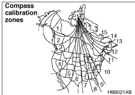
1. The zone setting is factory preset to Zone 8. Refer to the "Compass calibration zone" map shown above or one attached to the end of this manual to verify that the compass zone setting is correct for your geographical location.
