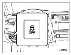
Pressing the Vehicle Dynamics Control OFF switch deactivates the Vehicle Dynamics Control system.
