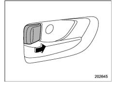
2. Rotate the lock lever forward.
