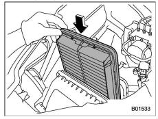
5. Install a new air cleaner element in the way the longitudinal side and the transverse side face as shown in the illustration.
