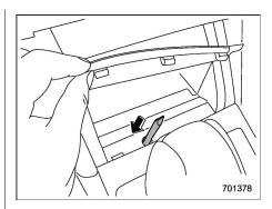
5. While depressing the brake pedal, insert the screwdriver into the hole, press the shift lock release portion using the screwdriver, and then move the select lever.
