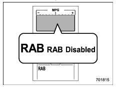
If the Reverse Automatic Braking System malfunctions, the above indicator illuminates on the combination meter. Contact the nearest SUBARU dealer for details.
