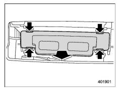
Remove the cover of the cabin air filter.
