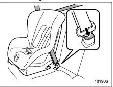
12. To remove the child restraint system, press the release button on the seatbelt buckle and allow the belt to retract completely. The belt will return to the ELR mode.
