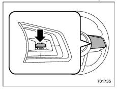
2. Press the "RES/SET" switch to the "SET" side once. Now the desired speed is set and the vehicle will keep running at that
