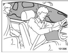
The following airbags deploy independently of each other because each has its own impact sensor.
