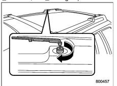
7. Install the plastic plug by pushing it into the hole until it is fully seated.
