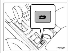
You can activate/deactivate the Hill Holder function by pressing the Hill Holder switch.
