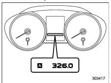
This meter displays the two trip meters when the ignition switch is in the "ON" position.
