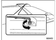
2. Remove the cap of the roof rail holder by using the torque wrench.
