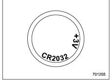
3. Remove the circuit board from the bottom half of the case and remove the battery and replace with a new one. Be sure to observe the (+) sign on the old battery before removing it to ensure that the new battery is inserted properly (battery "+" should be pointed away from the transmitter circuit board on the battery).
