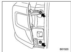
Tighten the upper and lower screws.
