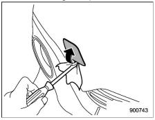
2. Prv off the towing access cover on the front bumper using a screwdriver, and you will find a threaded hole for attaching the towing hook.
