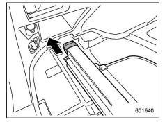
5. Insert the left end of the cover housing into the retainer.
