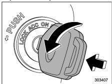
The key can be turned from "ACC" to "LOCK" only when the key is pushed in while turning it (all models) and the select lever is in the "P" position.
