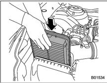
4. Install a new air cleaner element in the way the longitudinal side and the transverse side face as shown in the illustration.
