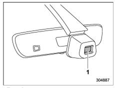
Type A Camera for high beam assist function
