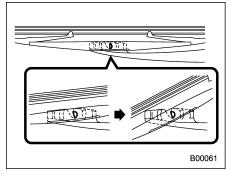
2. Turn the wiper blade assembly counterclockwise.
