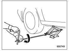
11. Insert the jack handle into the jackscrew, and turn the handle until the tire clears the ground. Do not raise the vehicle higher than necessary.
