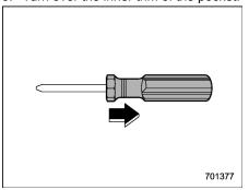
4. Remove the grip portion of the screw-driver.
