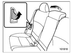
Adjust the seatback to the desired position while pulling the lever.
