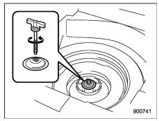
6. Take out the under-floor storage compartment and turn the attaching bolt counterclockwise, then take the spare tire out.
