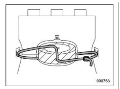
6. Fasten the tire fixing band to secure the tire bag.
