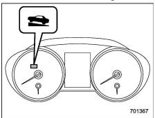
When the Hill Holder function is activated, the Hill Holder indicator light illuminates. Refer to "Hill Holder indicator light" \$\tilde{\pi}\$-3-22.
