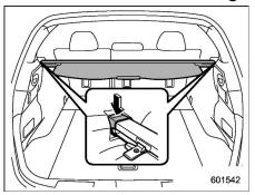
1. Insert both ends of the cover housing into the retainers.
