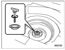
Store the flat tire in the spare tire compartment. Put the spacer and tighten the attaching bolt firmly.
