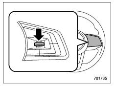
Press the "RES/SET" switch to the "SET" side and hold it until the vehicle reaches the desired speed. Then, release the switch. The vehicle speed at that moment will be memorized and treated as the new set speed.
