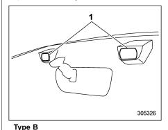
Stereo camera for high beam assist
