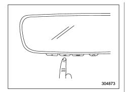
7. Return to the vehicle and firmly press, hold for 2 seconds and release the HomeLink® button up to three times. At this point programming is complete and vour device should operate when the HomeLink® button is pressed and released.
