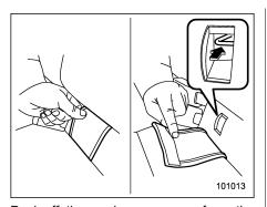
Peel off the anchorage cover from the selected side of the rear seatback to expose the anchorages (bars) to be used for installation of the child restraint system.
