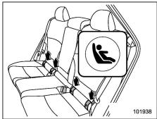
You will find marks "at the rear seat cushion. These marks indicate the positions of the lower anchorages (bars).
