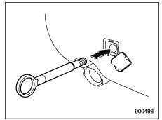
3. Screw the towing hook into the threaded hole until its thread can no longer
