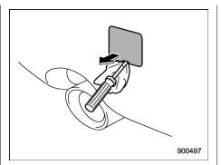
2. Pry off the cover on the rear bumper using a screwdriver, and you will find a threaded hole for attaching the towing hook.
