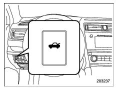
Press and hold the trunk lid opener switch for more than 1 second.
