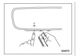
3. While the HomeLink® indicator light is flashing orange, press and hold the handheld remote button. Continue pressing the hand-held remote button until the HomeLink® indicator light changes from orange to green. You may now release the hand-held remote button
