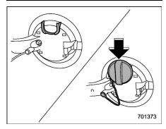
5. Set the fuel filler cap on the cap holder inside the fuel filler lid.
