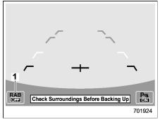
Reverse Automatic Braking system OFF indicator
