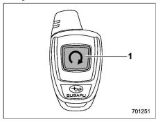
Remote engine starter transceiver (fob)
