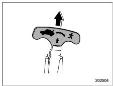
To open the trunk lid from inside the trunk, pull the vellow handle as indicated by the arrow on the handle. This operation unlocks the trunk lid. Then, push up the lid. The handle is made of material that remains luminescent for approximately an hour in the dark trunk space after it is exposed to ambient light even for a short time.
