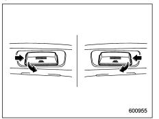
1. The license plate light must be pushed inwards, and then pulled out to be removed.
