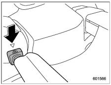
2. Make sure to fix the front part of the cargo area cover behind the rear seat.
