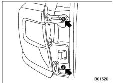
3. Remove the upper and lower screws.
