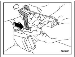
2. Insert a tongue plate or other hard pointed object into the slot in the connector (buckle) on the right-hand side and push it in. The connector (tongue) plate will then disconnect from the buckle.
