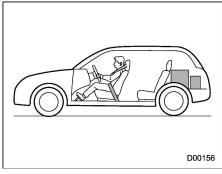
Vehicle capacity weight of the vehicle is 800 lbs (363 kg), which is indicated on the vehicle placard with the statement "The combined weight of occupants and cargo should never exceed 363 kg or 800 lbs".
