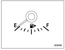
The fuel gauge shows the approximate amount of fuel remaining in the tank. When the ignition switch is in the "LOCK"/ "OFF" or "ACC" position, the fuel gauge shows "F" even if the fuel tank contains
