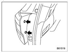
1. Undo the clips. For the method to undo the clips, refer to "Type C clips" \$\tilde{T}\$11-6.
