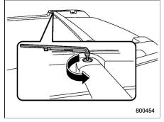
3. Remove the bolt of the crossbar by using the torque wrench.
