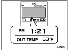
This screen displays the clock and the outside temperature.
