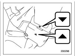
4. After fastening the seatbelt, make sure that the "▼" mark on the connector (tongue) and the "▲" mark on the buckle face outwards.
