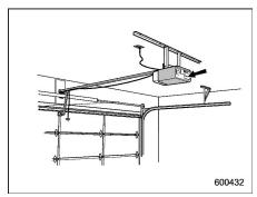
Locate the training button on the garage door opener motor head unit. The exact location and color of the button may vary by brand of garage door opener. If it is difficult to locate the training button, refer to your garage door opener's instruction manual.
