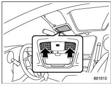
To turn on the map light, press the lens. To turn it off, press the lens again.
