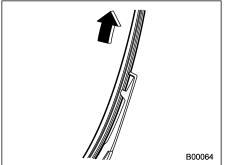
2. Pull the blade rubber assembly out of the plastic support.
