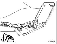
4. Fasten the top tether hook of the child restraint system to the appropriate upper
