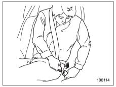
5. Insert the center seatbelt tongue plate into the center seatbelt buckle marked
