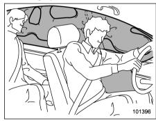
The driver's and front passenger's SRS side airbags and SRS curtain airbags deploy independently of each other because each has its own impact sensor. Therefore, they may not both deploy in the same accident. Also, the SRS side airbag and SRS curtain airbag deploys indepen-
