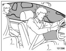
The driver's and front passenger's SRS side airbags and SRS curtain airbags deploy independently of each other because each has its own impact sensor. Therefore, they may not both deploy in the same accident. Also, the SRS side airbag deploys independently of the driver's and front passenger's SRS frontal airbags in the steering wheel and instrument panel.
