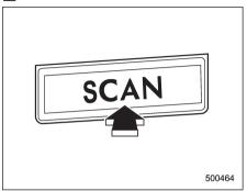
The scan mode lets you listen to the first 10 seconds of each track/file in succession. Press the "SCAN" button to start scanning upward beginning with the track/file(s) following the currently selected one. After all track/file(s) in the disk/folder have been scanned, normal playback will be resumed. To cancel the scan mode, press the "SCAN" button again.
