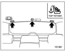
Three tether anchorages, i.e., ones for the right, center and left positions, are already installed on the rear edge of the roof. Open the cover flap to use each anchorage.
