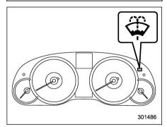
If you spray washer fluid on the windshield but the windshield washer fluid warning light illuminates or the supply of washer fluid runs out, add washer fluid in the tank.
