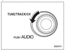
Turn the "TUNE/TRACK/CH" dial counterclockwise to skip to the beginning of the current track/file (track). Each time the dial is turned, the indicated track/file (track) number will decrease.
