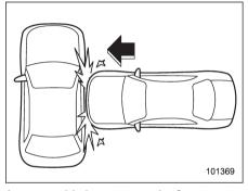
A severe side impact near the front seat or the rear seat activates the SRS curtain airbag.
