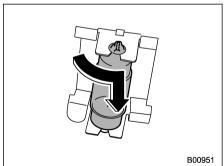
2. Turn the bulb until the flat surfaces at its ends are aligned vertically. Pull the bulb straight downward to remove it.
