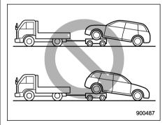
If towing is necessary, it is best done by vour SUBARU dealer or a commercial towing service. Observe the following procedures for safety.
