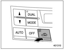
Select airflow by pressing the air inlet selection button "-----".
