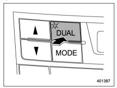
It is possible to make separate temperature settings for the driver's side and passenger's side (DUAL mode).
