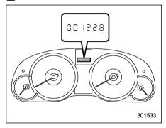
This meter displays the odometer when the ignition switch is in the "ON" position. The odometer shows the total distance that the vehicle has been driven.
