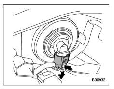
3. Disconnect the electrical connector from the bulb.
