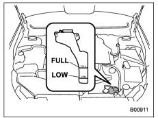
Check the coolant level at each fuel stop.
