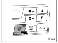
To defrost or dehumidify the windshield and front door windows, press the defroster button "\(\frac{1}{1444}\)". When the "\(\frac{1}{1444}\)" button is pressed, the air conditioner compressor automatically operates to quickly defog the windshield, outside air is drawn into the passenger compartment, airflow is directed towards the windshield and front door windows, and the indicator light on the button illuminates.
