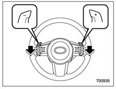
Pull the "+" of the paddle shift to upshift one level. Also pull the "-" of the paddle shift to downshift one level.
