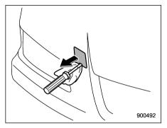
2. Prv off the cover on the front bumper using a screwdriver, and you will find a threaded hole for attaching the towing hook
