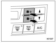
The fan speed control button has 6 different fan speed positions.
