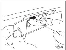
3. Pull the bulb out of the socket.
