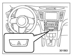
The hazard warning flasher is used to warn other drivers when you have to park vour vehicle under emergency conditions. The hazard warning flasher works with the ignition switch in any position.
