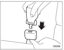
3. After confirming that the webbing is not twisted, insert the connector (tongue) attached at the webbing end into the buckle on the right-hand side until a click is heard. If the belt stops before reaching the buckle, return the belt slightly and pull it out more slowly. If the belt still cannot be unlocked, let the belt retract slightly after giving it a strong pull, then pull it out slowly again.
