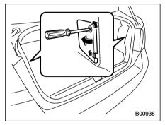
1. Turn the knobs of the cover 90 degrees counterclockwise to remove the cover.
