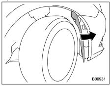
6. After replacing the bulb, reattach the fender lining.
