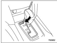
2. Remove the shift lock cover using a flat-head screwdriver.
