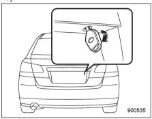
To open the trunk lid, insert the key into the key cylinder and turn it clockwise.
