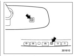
The mirror has a photosensor attached on both the front and back sides. During nighttime driving, these sensors detect distracting glare from vehicle headlights behind you and automatically dim the mirror to eliminate glare and preserve vour vision. For this reason, use care not to cover the sensors with stickers, or other similar items. Periodically wipe the sensors clean using a piece of dry soft cotton cloth or an applicator.
