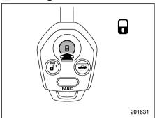
Press the "a" button to lock all doors and rear gate (Outback). An electronic chirp will sound once and the turn signal lights will flash once.
