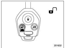
Press the "\" button to unlock the driver's door. An electronic chirp will sound twice and the turn signal lights will flash twice. To unlock all doors and the rear gate (Outback), briefly press the "" button a second time within 5 seconds.
