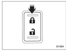
5. Before the electronic tone stops sounding, press the lock side of the power door lock switch the same number of times as the leftmost digit of the transmitter code. For example, press the lock switch eight times if the leftmost digit of the code is 8.
