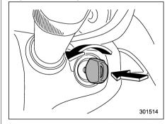
The key can be turned from "Acc" to "LOCK" only when the key is pushed in while turning it (all models) and the select lever is in the "P" position (AT and CVT models).
