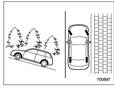
When parking on a hill, always turn the steering wheel as described here. When the vehicle is headed up the hill, the front wheels should be turned away from the curb.
