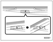
2. Turn the wiper blade assembly counterclockwise.
