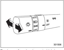
To change from low beam to high beam, push the turn signal lever forward. When the headlights are on high beam, the high beam indicator light "\( \bar{\bar{\texts}} \)" on the combination meter is also on.
