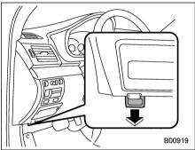
2. Pull the hood release knob under the instrument panel.
