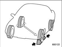
4. Put wheel blocks at the front and rear of the tire diagonally opposite the flat tire.
