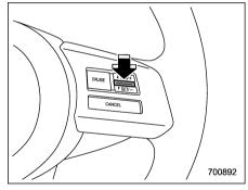
Press the "RFS/SFT" switch to the "SFT" side and hold it until the vehicle reaches the desired speed. Then, release the switch. The vehicle speed at that moment will be memorized and treated as the new set speed.
