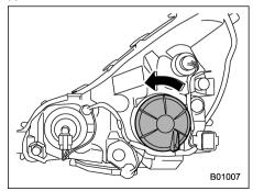
2. Remove the bulb cover, by turning it
