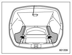
3. Remove the left and right parts of the cargo floor lid.
