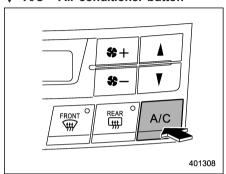
If the windshield starts to fog when the climate control system is operated in the AUTO mode, press the air conditioner button "A/C" to defog and dehumidify.
