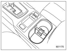
The dual cup holder is built into the center console.
