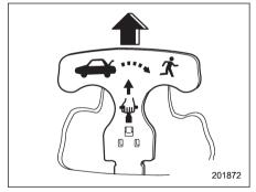
To open the trunk lid from inside the trunk, pull the vellow handle as indicated by the arrow on the handle. This operation unlocks the trunk lid. Then, push up the lid.
