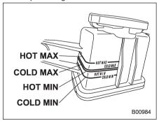
2. Check the fluid level of the reservoir
