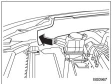
4. After replacing the bulbs, reposition the protective cover of the engine compartment.
