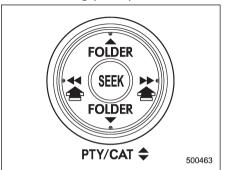
If you press the "\( \ "\) or "\( \)" side of the "SEEK" button briefly, the radio will automatically search for a receivable station and stop at the first one it finds. This function may not be available, however, when radio signals are weak. In such a situation, perform manual tuning to select the desired station.
