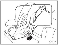
1. While following the instructions supplied by the child restraint system manufacturer, connect the lower hooks onto the lower anchorages located at "s" marks on the bottom of the rear seatback. When the hooks are connected, make sure the adjacent seatbelts are not caught.
