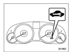
6. Briefly press the "A" button (for less than 2 seconds). All doors (and the rear gate (Outback)) will lock, an electronic chirp will sound once, the turn signal lights will flash once, and the security indicator light will start flashing rapidly. After rapid flashing for 30 seconds (standby time), the security indicator light will then flash slowly (twice approximately every 2 seconds), indicating that the system has been armed for surveillance
