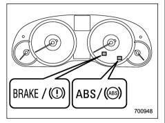
If a malfunction occurs in the EBD system. the system stops working and the brake system warning light and ABS warning light illuminate simultaneously.
