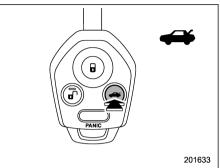
Pressing the "a" button unlocks the rear gate.
