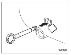
3. Screw the towing hook into the threaded hole until its thread can no longer be seen.
