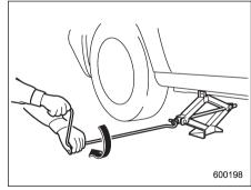
9. Insert the jack handle into the jackscrew, and turn the handle until the tire clears the ground. Do not raise the vehicle higher than necessary.
