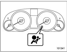
A diagnostic system continually monitors the readiness of the SRS airbag system (including front seatbelt pretensioners) while the vehicle is being driven. The SRS airbag system warning light will show normal system operation by illuminating for approximately 6 seconds when the ignition switch is turned to the "ON" position.
