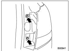
3. Remove the upper and lower screws.
