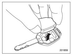
3. Remove the transmitter case from the kev head.
