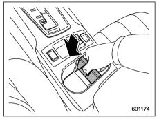
Insert the divider plate into the console box.
