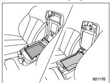
The center console box has a two-layer structure consisting of an upper compartment and a lower compartment.
