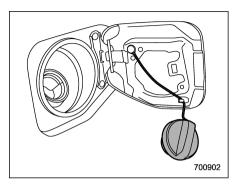
4. Hook the cord that is attached to the fuel filler cap onto the hook inside the fuel filler lid.
