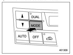
Select the desired airflow mode by pressing the airflow mode selection button. The selected airflow mode is shown on the display.
