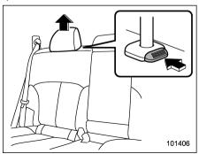
1. Remove the head restraint at the seating position where the child restraint system has been installed with the seat-belt or lower anchorages; lift up the head restraint while pressing the release button. Store the head restraint in the cargo area. Avoid placing the head restraint in the passenger compartment to prevent it from being thrown around in the passenger compartment in a sudden stop or a sharp turn.
