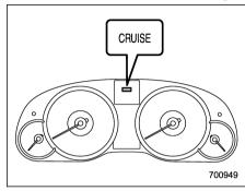
The cruise control indicator light illuminates when the ignition switch is turned to the "ON" position and turns off after approximately 3 seconds.
