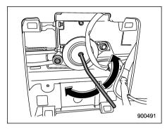
4. Insert the hex-head wrench in the end of the motor shaft.
