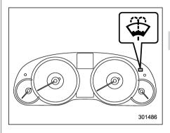
The windshield washer fluid warning light illuminates when the washer fluid level in the tank has dropped to the lower limit. If the warning light illuminates, refill the tank with fluid. For the tank refilling method, refer to "Windshield washer fluid" @11-40.
