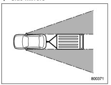
After hitching a trailer to your vehicle, check that the standard side mirrors provide a good rearward field of view without significant blind spots. If significant blind spots occur with the vehicle's standard side mirrors, use towing mirrors that conform with Federal, state/province and/or other applicable regulations.
