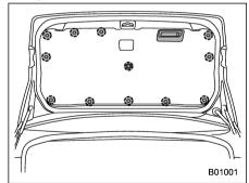
2. Remove the trunk trim lining by removing the 12 clips and the trunk trim handle.
