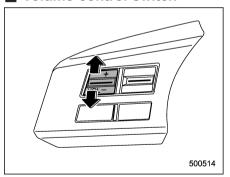
Press the switch to the "+" side to increase the volume. Press the switch to the "-" side to reduce the volume.
