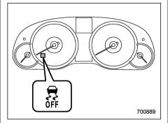
The light illuminates when the ignition switch is turned to the "ON" position and turns off after approximately 2 seconds. The light illuminates when the Vehicle Dynamics Control OFF switch is pressed to deactivate the Vehicle Dynamics Control system.
