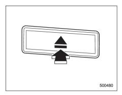
2. Briefly press the "\_A" button. The selected disc will be ejected. The disc number indicator will flash at this time. When you remove the ejected disc, the disc number indicator will turn off.
