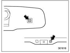
The mirror has a photosensor attached on the front and back sides. During nighttime driving, these sensors detect distracting glare from vehicle headlights behind you and automatically dim the mirror to eliminate glare and preserve your vision. For this reason, use care not to cover the sensors with stickers, or other similar items. Periodically wipe the sensors clean using a piece of dry soft cotton cloth or an applicator.
