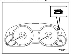
When the Hill Holder function is activated. the Hill Holder indicator light illuminates. Refer to "Hill Holder indicator light" \$\tilde{\pi}\$3-19.
