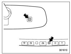
The mirror has a photosensor attached on both the front and back sides. During nighttime driving, these sensors detect distracting glare from vehicle headlights behind you and automatically dim the mirror to eliminate glare and preserve your vision. For this reason, use care not to cover the sensors with stickers, or other similar items. Periodically wipe the sensors clean using a piece of dry soft cotton cloth or an applicator.
