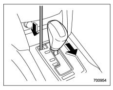
3. While depressing the brake pedal. insert the electronic parking brake release tool into the hole, press the shift lock release button using the tool, and then move the select lever
