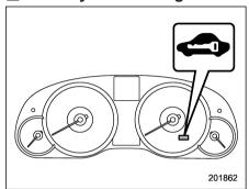
The security indicator light deters potential thieves by indicating that the vehicle is equipped with an immobilizer system. It begins flashing approximately 60 seconds after the ignition switch is turned from the "ON" position to the "Acc" or "LOCK" position or immediately after the key is pulled out.
