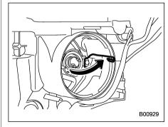
4. Remove the retainer spring.
