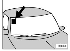
For some models, the satellite radio antenna is fixed to the upper right hand corner of the windshield.
