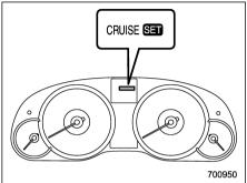
At this time, the cruise control set indicator light is illuminated in the combination meter
