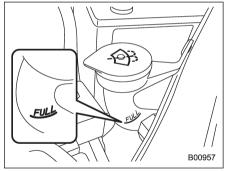
Remove the washer tank filler cap, then add fluid until it reaches the "FULL" mark on the tank.
