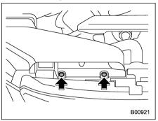
Use a screwdriver to undo the clips on the air intake duct, then remove the air intake duct. Refer to "Type A clips" \$\tilde{\pi}\$11-5.
