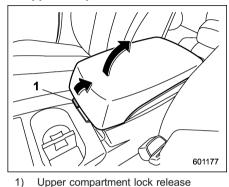
Pull up the upper compartment lock release to open the upper compartment.
