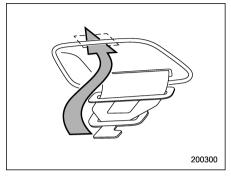
2. Allow the retractor to roll up the belt. You should hold the webbing end and guide it back into the retractor while it is rolling up. Neatly store the tongue plate in the recess and then insert the connector (tongue) plate into the slot.
