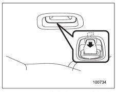
Rear center seatbelt is stowed in the recess of the ceiling.
