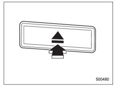
When a disc is being played back or when a disc is in the player, press the eject button "\_a". The disc will be ejected.
