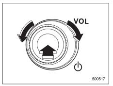
The dial is used for both power (ON/OFF) and volume control. The radio is turned ON and OFF by pressing the dial, and the volume is controlled by turning the dial.
