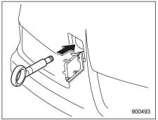
3. Screw the towing hook into the threaded hole until the threads can no longer be seen.
