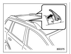
1. Pull out the crossbars from the roof rail holders by pulling up the covers.
