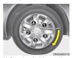
11. Once the wheel lug nuts have been tightened, lower the vehicle fully to the ground and continue to tighten the lug nuts until they are fully secured. Tighten the wheel lug nuts firmly in a "star" pattern. If you are unsure of the tightness of the wheel lug nuts, have them checked at the nearest service station. The specified tightening torque is 65-79 lb•ft (9~11 kg•m, 88-107 N•m). Improperly tightened wheel lug nuts could cause brake pedal vibration while braking.
