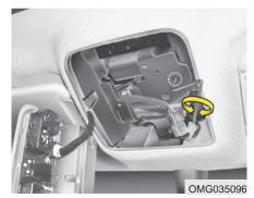
Insert the emergency handle (provided with the vehicle) and turn the handle clockwise to open or counterclockwise to close.
