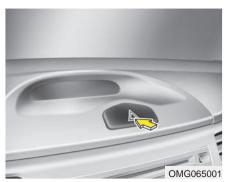
The hazard warning flasher causes the rear tail lights and front turn signal lights to flash on and off, which serves as a warning to other drivers to exercise caution when approaching or passing your vehicle.
