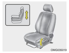
Adjusting height of the driver's seat cushion (if equipped)
