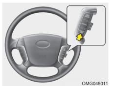
3. Press the COAST/SET switch, located on the steering wheel, and release it at the speed you want. Release the accelerator at the same time. The desired speed will automatically be maintained.
