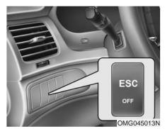
The Electronic Stability Control (ESC) monitors information from various vehicle sensors and then compares the driver's commands with the actual behavior of the vehicle. If an unstable condition occurs - a sudden evasive movement for example - ESC intervenes within fractions of a second via the engine computer and brake system and attempts to stabilize the vehicle.
