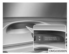
If there is no passenger in the front passenger seat or if the passenger in the front passenger's seat is very small (such as a child), the front PASSENGER AIR BAG OFF indicator may go ON.
