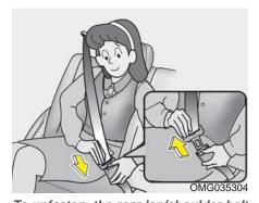
To unfasten: the rear lap/shoulder belt Press the release button on the buckle and allow the belt to slowly retract.
