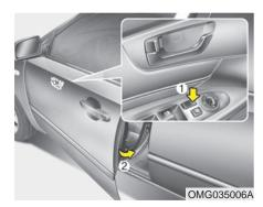
To lock a door without the key, push the inside central door lock switch (1) to the "LOCK" position and close the door (2).
