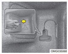
When fuel filler lid does not open with the release button
