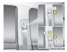
Adjust the shoulder anchor position to your size. To raise the anchor position, push the anchor up (1). To lower the anchor position, press (2) the button (A) and slide the anchor down (3). After adjustment, make sure the anchor is locked in position.
