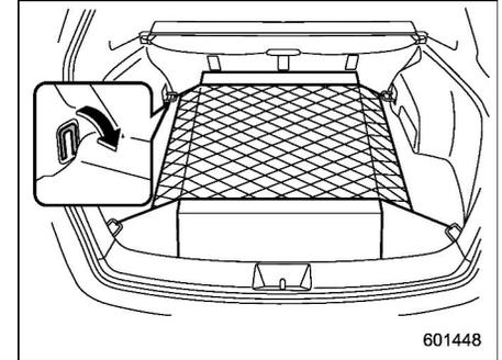
The cargo area is equipped with several tie-down hooks so that cargo can be secured with a cargo net or ropes. When using the tie-down hooks, turn them down out of the storing recesses.
