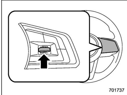
To resume the cruise control after it has been temporarily canceled and with vehicle speed of approximately 20 mph (30 km/h) or more, press the “RES/SET”
