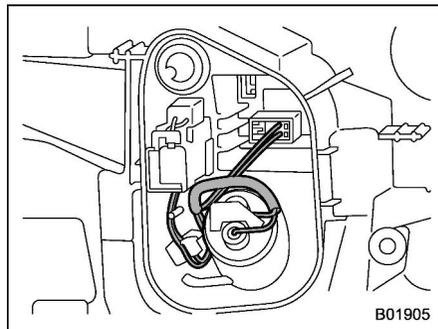
6. Install the light cover on the rear gate.
