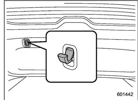
A convenience hook is attached to the rear gate trim. When the rear gate is open, you can hang a lantern, wet suit, etc. on the hook.
