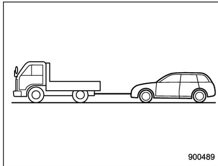
1. Release the parking brake and put the transmission in the neutral position.
