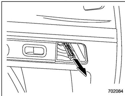
3. Pull the orange knob to unlock the fuel filler lid.
