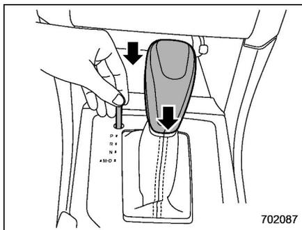
3. While depressing the brake pedal, insert a screwdriver into the hole, press the shift lock release button using a screwdriver, and then move the select lever.
