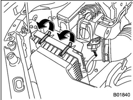
1. Unsnap the two clips holding the air cleaner case (rear).
