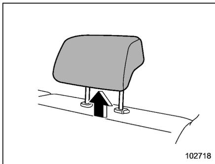
(1) Raise the head restraint to the extended position (center seat). Do not remove the head restraint.
