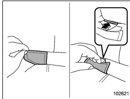
3. Peel off the anchorage cover from the selected side of the rear seatback. Fold the peeled anchorage cover in half and affix it with hook and loop tape to expose the anchorages (bars) to be used for installation of the child restraint system.
