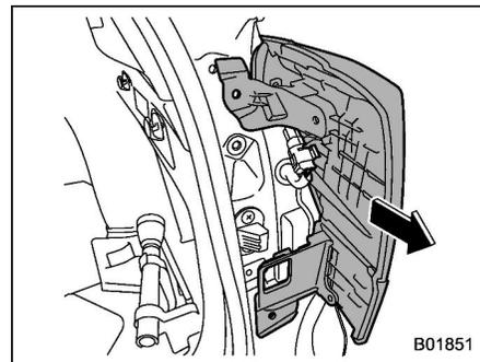
6. Slide the rear combination light assembly rearward to remove it from the vehicle.
