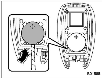
3. Take out the battery using a flat-head screwdriver with vinyl tape or a cloth.
