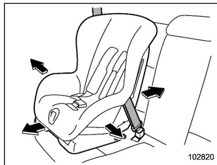
8. Before having a child sit in the child restraint system, try to move it back and forth and right and left to check if it is firmly secured. Sometimes a child restraint system can be more firmly secured by pushing it down into the seat cushion and then tightening the seatbelt. It should not be possible to move the child restraint system more than 1 in (2.5 cm) in any direction along the seatbelt path.
