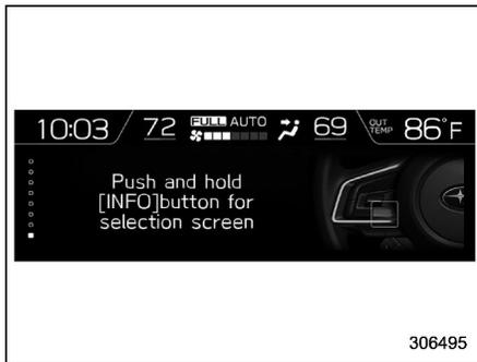
When the INFO button on the steering wheel is pressed and held on this screen, the setting screen can be displayed.
