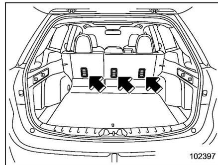
The tether anchorages (upper anchorages) are provided at the locations shown in the above illustration. For details, refer to "Top tether anchorages" P77.
