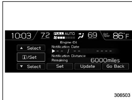
2. Set the date and distance of the reminder by using the control switches.
