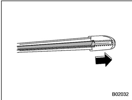
4. Insert the wiper blade rubber into the slit, then return to the tip of the position.
