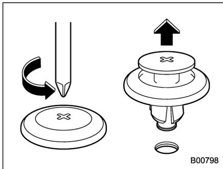
1. Turn the clip counterclockwise using a Phillips screwdriver until the center portion of the clip is raised.
