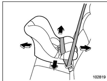
6. Before having a child sit in the child restraint system, try to move it back and forth and right and left to check if it is firmly secured. Sometimes a child restraint system can be more firmly secured by pushing it down into the seat cushion and then tightening the seatbelt. It should not be possible to move the child restraint system more than 1 in (2.5 cm) in any direction along the seatbelt path.
