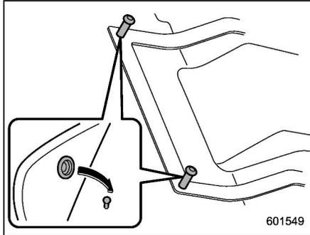
Retaining pins are located on the driver's side floor.
