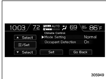
2. Select “Normal”, “Mild”, “Power” or “ECO” by using the control switches. For details about “Mode Setting”, refer to “Automatic climate control customization (for type B and C)” P272.
