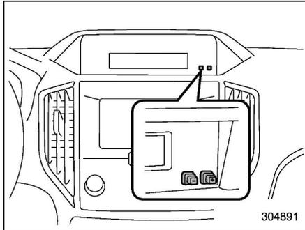
1. Press and hold the “+” button located on the side of the information display. The stopped time will then flash.
