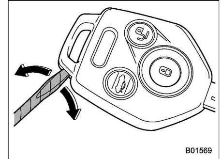
1. Wrap a flat-head screwdriver with vinyl tape or a cloth. Open the key head using a flat-head screwdriver.
