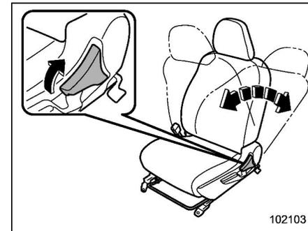
Pull the reclining lever up and adjust the seatback to the desired position. Then release the lever and move the seatback back and forth to confirm that it is securely fixed in place.
