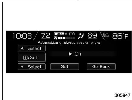
2. Select “On” or “Off” to turn the auto entry/exit function on or off by using the control switches.
