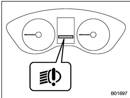
The LED headlight warning light illuminates if the LED headlights malfunction. Have your vehicle inspected at a SUBARU dealer as soon as possible.
