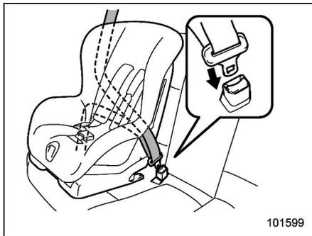
4. Run the lap and shoulder belt through or around the child restraint system following the instructions provided by its manufacturer.
