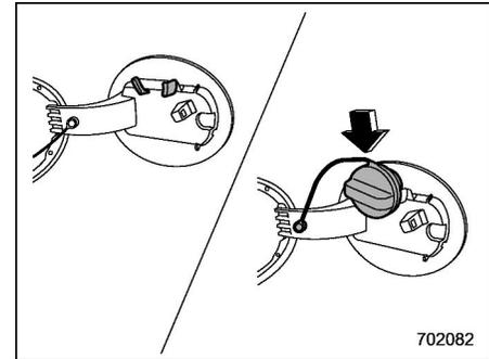
6. Set the fuel filler cap on the cap holder inside the fuel filler lid.
