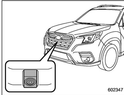
The image from the camera mounted inside the front grille is displayed in the multi-function display (color LCD). This eliminates blind spots and allows the driver to check the forward direction of both sides.
