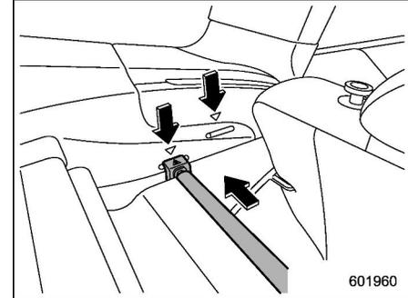
1. Align the right side of the front cover with the triangle mark before fixing the cover in place.
