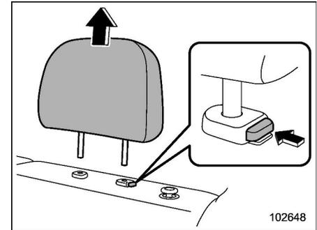
5. Remove the rear seat head restraint. For details, refer to “Head restraints” P45.
