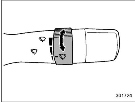
When the wiper switch is in the
