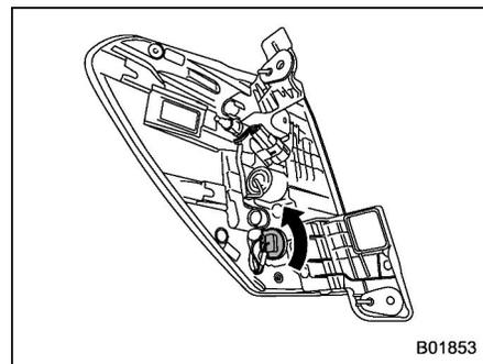
7. Remove the bulb socket from the rear combination light assembly by turning it counterclockwise.
