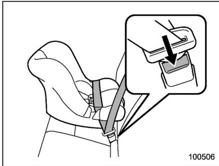
8. To remove the child restraint system, press the release button on the seatbelt buckle and allow the belt to retract completely. The belt will return to the ELR mode.
