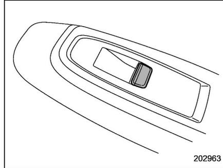
Each passenger's window can be controlled by the power window switch located on the door.
