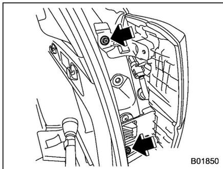
5. Using a Phillips screwdriver, remove the screws that secure the rear combination light assembly.
