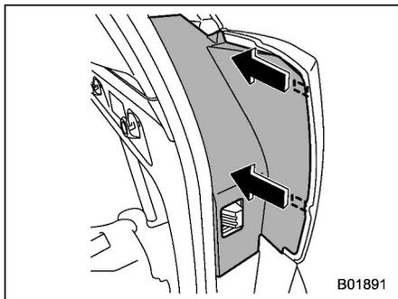
2. Push and move the cover to the forward to unlock the 2 tabs.
