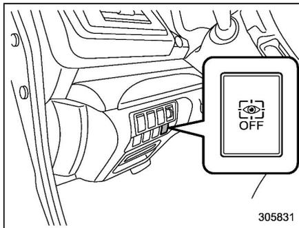
When the Driver Monitoring System OFF switch is pressed, the Driver Monitoring System turns OFF. When the Driver Monitoring System is turned OFF, the Driver Monitoring System OFF indicator on the combination meter display will illuminate. To turn the Driver Monitoring System ON, press the Driver Monitoring System OFF switch again.
