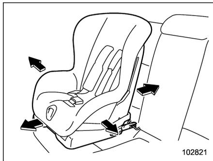
9. Before having a child sit in the child restraint system, try to move it back and forth and right and left to check if it is firmly secured. Sometimes a child restraint system can be more firmly secured by pushing it down into the seat cushion. It should not be possible to move the child restraint system more than 1 in (2.5 cm) in any direction along the seatbelt path.
