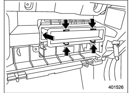
3. Replace the cabin air filter element with a new one.
