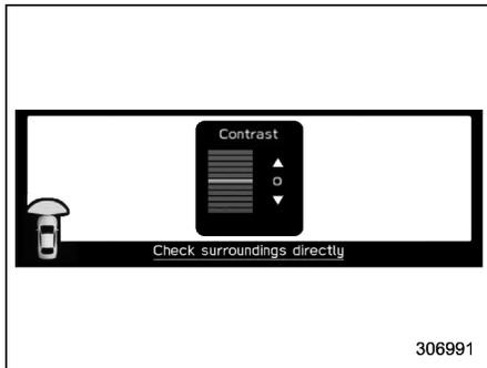
2. Select the contrast level by using the control switches.
