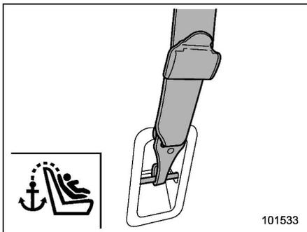
3. Attach the top tether hook to the appropriate upper anchorage.
