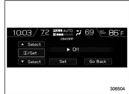
2. Select “On” or “Off” to turn the opening screen on or off by using the control switches.
