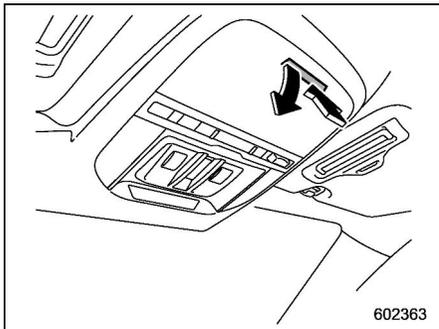
To open the console, push on the lid lightly and it will automatically open.
