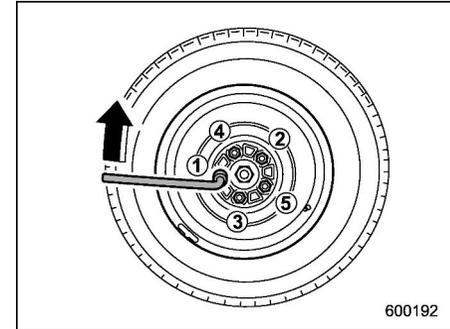
15. Use the wheel nut wrench to securely tighten the wheel nuts to the specified torque, following the tightening order in the illustration.
