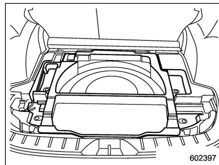
The storage compartment is located under the floor of the cargo area and can be used to store small items. Pull the strap to open the center part of the cargo floor lid, and then remove the lid.
