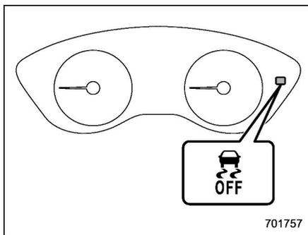
When the switch is pressed or turned during engine operation, the Vehicle Dynamics Control OFF indicator light “OFF” on the combination meter illuminates. The Vehicle Dynamics Control system will be deactivated and the vehicle will behave like a model not equipped with the Vehicle Dynamics Control system. When the switch is pressed again (type A) or turned to the “NORMAL” side (type B) to reactivate the Vehicle Dynamics Control system, the Vehicle Dynamics Control OFF indicator light turns off.
