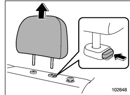
3. Remove the head restraint of the rear seating position where the child restraint system is to be installed. For details, refer to "Head restraints" P45.
