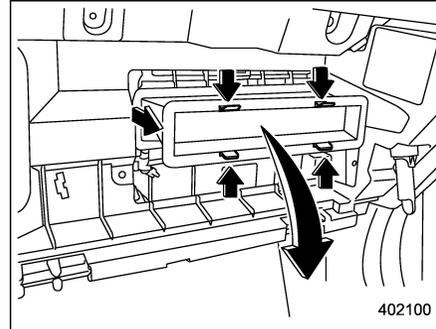
2. Remove the cabin air filter according to the following procedure in order to prevent dust on the cabin air filter from falling to the inside of its housing.
