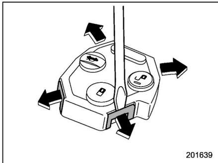
3. Open the transmitter case by releasing the hooks.
