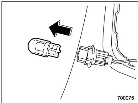
3. Pull the bulb out of the bulb socket and replace it.
