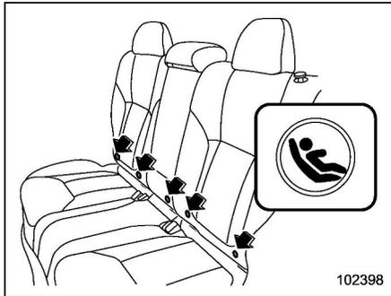
2. You will find “Ⓢ” marks at the bottoms of the rear seatback. These marks indicate the positions of the lower anchorages (bars).
