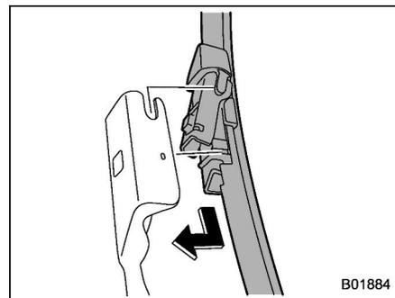
3. When installing the wiper blade assembly, align it with the wiper arm connection part and then slide it in the opposite direction of removal to install. After installing the wiper blade assembly, check that the connection part is locked completely.
