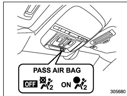
ON Front passenger’s frontal airbag ON indicator
