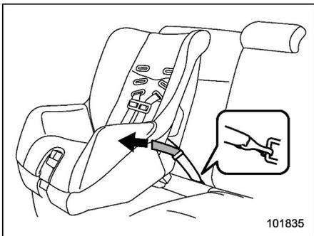
7. If your child restraint system is a flexible attachment type (which uses tether belts), push the child restraint system into the seat cushion and pull both left and right lower tether belts up to secure the child restraint system by taking up the slack in the belt.
