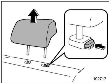
(1) Remove the head restraint from the rear seating position where the child restraint system is to be installed.
