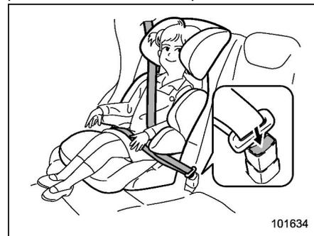
6. To remove the booster seat/cushion, press the release button on the seatbelt buckle and allow the belt to retract.
