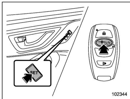
2. Hold the access key fob and press and hold the “SET” button, then press the “
