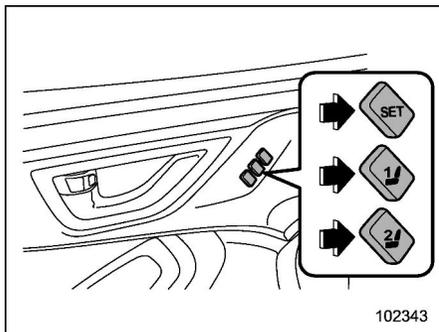
2. Register the adjusted positions by either of the following procedures.
