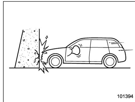
A head-on collision against a thick concrete wall at a vehicle speed of 12 to 19 mph (20 to 30 km/h) or higher activates only the driver's SRS frontal airbag or both driver's and front passenger's SRS frontal airbags. The airbag(s) will also be acti-
