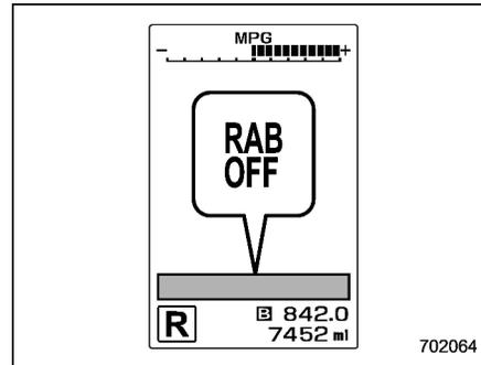
RAB OFF indicator light: illuminates when the Reverse Automatic Braking (RAB) system is turned OFF.
