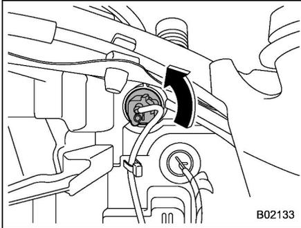
3. Disconnect the electrical connector from the bulb and remove the bulb from the headlight assembly by turning it counterclockwise.
