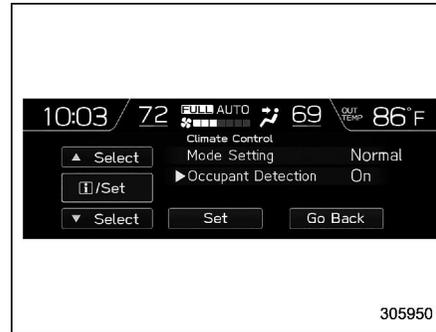
2. Select on or off to turn the occupant detection on or off by using the control switches.
