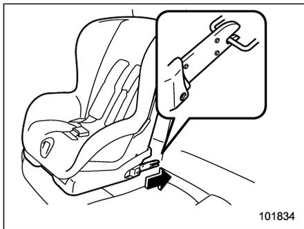
6. While following the instructions supplied by the child restraint system manufacturer, connect the lower hooks onto the lower anchorages located at “
