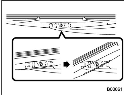
2. Turn the wiper blade assembly counterclockwise.
