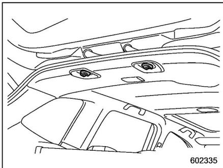
There are two hooks on the lining in the cargo area. Use them to hang or secure lightweight objects when the vehicle is stopped.
