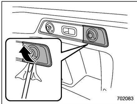
1. Remove the access cover at the right side of the cargo area trim using flat-head screwdriver.
