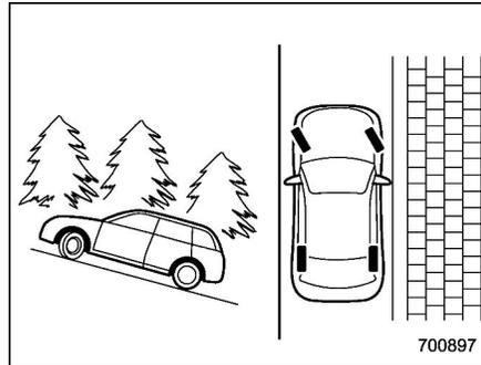
When parking on a hill, always turn the steering wheel. When the vehicle is
