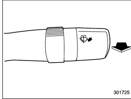
To wash the windshield, pull the wiper control lever toward you. The washer fluid sprays until you release the lever. The wipers operate while you pull the lever.
