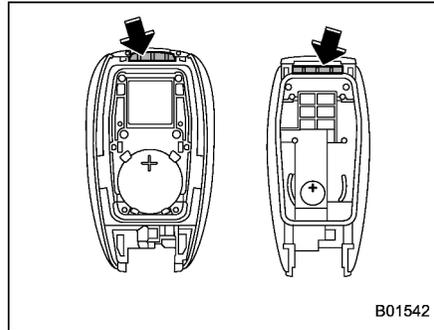
5. Attach the cover to the access key fob by fitting the projections and recesses together.
