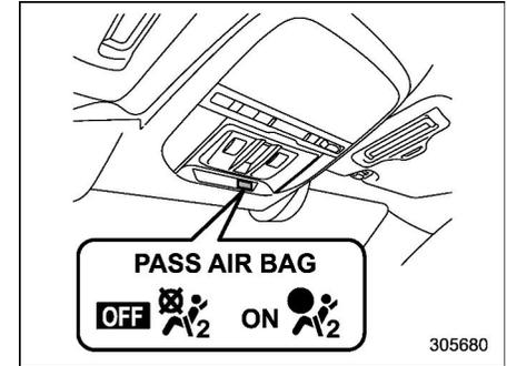
on : Front passenger's frontal airbag ON indicator
