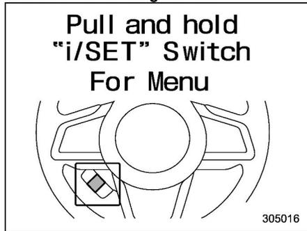
While this screen is selected, pull and hold the “i/SET” switch to enter the menu screen.
