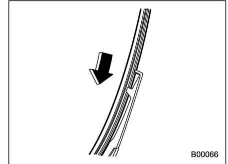
4. Align the claws of the plastic support with the grooves in the blade rubber assembly, then slide the blade rubber assembly into place.
