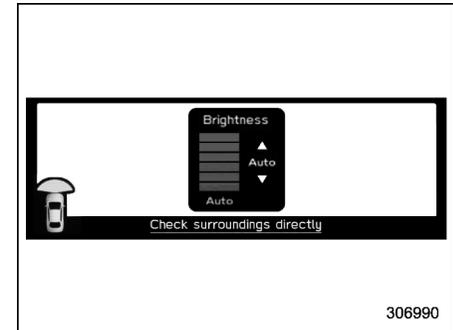
2. Select the brightness level by using the control switches.
