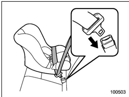
2. Run the lap and shoulder belt through or around the child restraint system following the instructions provided by its manufacturer.
