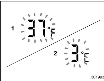
When the outside temperature drops to a certain temperature or lower, the temperature indication flashes for 5 seconds to show that the road surface may be frozen. If the display is already indicating that the outside temperature is low when the ignition switch is turned to the "ON" position, the indication does not flash.
