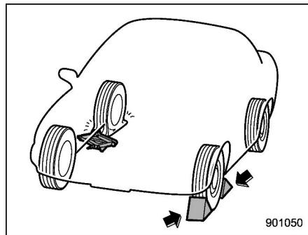
4. Put wheel blocks at the front and rear of the tire diagonally opposite the tire that you are going to replace.
