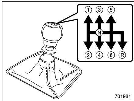
The manual transmission is a fully synchronized, 6-forward-speed and 1-reverse-speed transmission.
