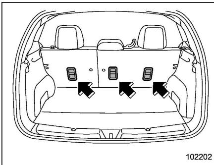
The tether anchorages (upper anchorages) are provided at the locations shown in the above illustration. For details, refer to "Top tether anchorages" 1-38.
