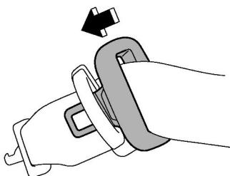
3. Allow the retractor to roll up the belt. You should hold the webbing end and guide it back into the retractor while it is rolling up. Insert the connector (tongue) into the belt holder.
