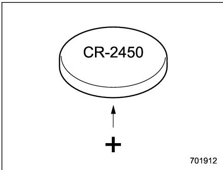
3. Remove the circuit board from the bottom half of the case and remove the battery and replace with new one. Be sure to observe the (+) sign on the old battery before removing it to ensure that the new battery is inserted properly (battery "+")
