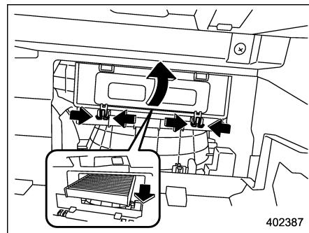
2. Remove the cabin air filter according to the following procedure in order to prevent dust on the air cleaner from falling to the inside of its housing.
