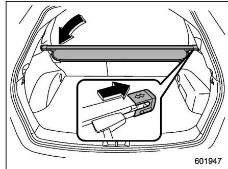
1. Insert the right end of the cover into the recessed portion with the arrow mark facing upward.
