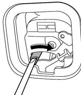
3. To open the rear gate, turn the lever to the right position using a flat-head screwdriver or a similar tool.
