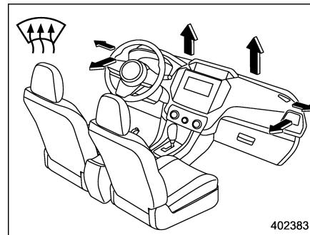
**Defrost:** Windshield defroster outlets and both side outlets of the instrument panel (Refer to "Defrosting"  $\Rightarrow$  4-10.)
