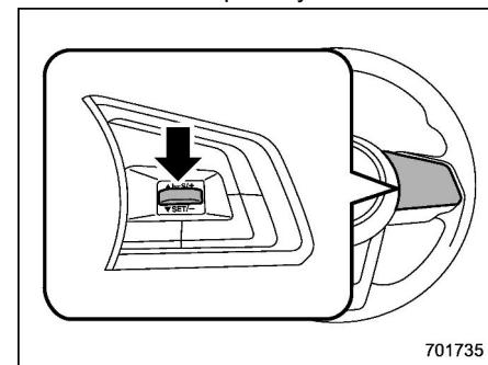
2. When the speed decreases to the desired speed, press the "RES/SET" switch to the "SET" side once. Now the desired speed is set and the vehicle will keep running at that speed without depressing the accelerator pedal.
