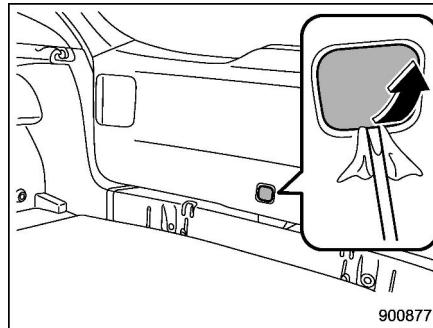
1. Remove the access cover at the bottom-center of the rear gate trim using a flat-head screwdriver wrapped with vinyl tape or a cloth.
