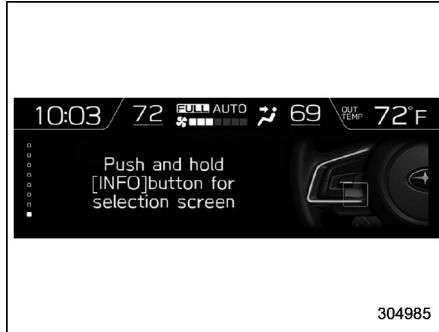
When the INFO button on the steering wheel is pressed and held on this screen, the setting screen can be displayed. For details, refer to "Setting screen" 3-57.
