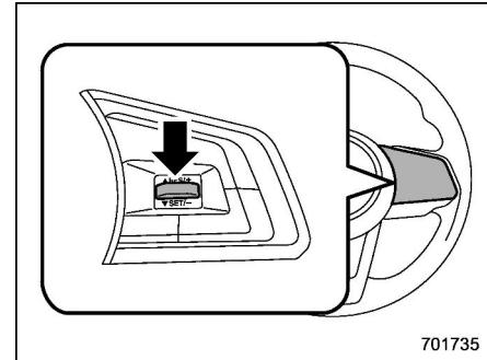
3. Press the "RES/SET" switch to the "SET" side and release it. Then release the accelerator pedal.
