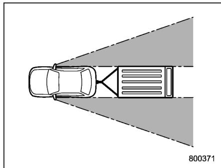
After hitching a trailer to your vehicle, check that the standard outside mirrors provide a good rearward field of view without significant blind spots. If significant blind spots occur with the vehicle's standard outside mirrors, use towing mirrors that conform with Federal, state/province and/or other applicable regulations.
