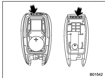
5. Attach the cover to the access key fob by fitting the projections and recesses together.
