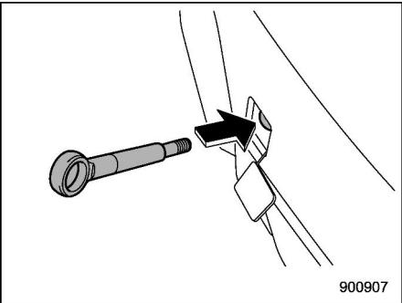
3. Screw the towing hook into the thread hole until its thread can no longer be seen.
