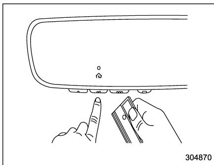
3. While the HomeLink indicator light is flashing orange, press and hold the hand-held remote button. Continue pressing the hand-held remote button until the HomeLink indicator light changes from orange to green. You may now release the hand-held remote button.
