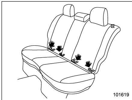
The lower anchorages (bars) are used for installing a child restraint system only on the rear seat window-side seating positions. For each window-side seating position, two lower anchorages are provided. Each lower anchorage is located where the seat cushion meets the seatback.
