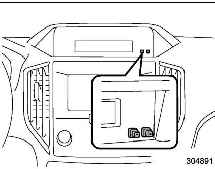
1. Press and hold the "+" button located on the side of the information display. The stopped time will then flash.
