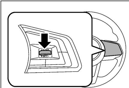
Press the "RES/SET" switch to the "SET" side and hold it until the vehicle reaches the desired speed. Then, release the switch. The vehicle speed at that moment will be memorized and treated as the new set speed.
