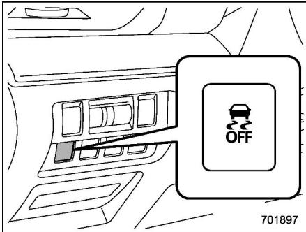
5. Press and hold the Vehicle Dynamics Control OFF switch for 30 seconds until the Vehicle Dynamics Control OFF indicator light
