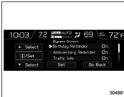
2. Select "On" or "Off" to turn the display of items on or off by using the control
