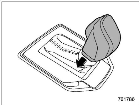
With the vehicle either moving or stationary, move the select lever from the "D" position to the "M" position to select the manual mode.
