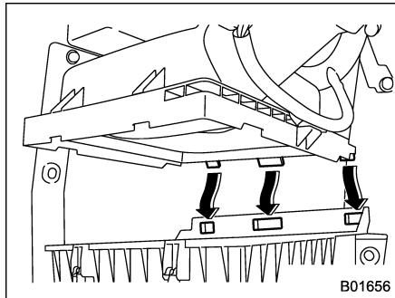
5. To install the air cleaner case (rear), insert the three projections on the air
