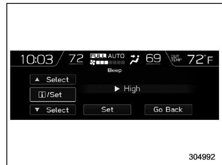
2. Set the beep volume by using the control switches.
