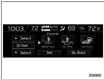
2. Set the desired items by using the control switches. For details about items, refer to "Favorite screen"  $\Rightarrow$  3-54.
