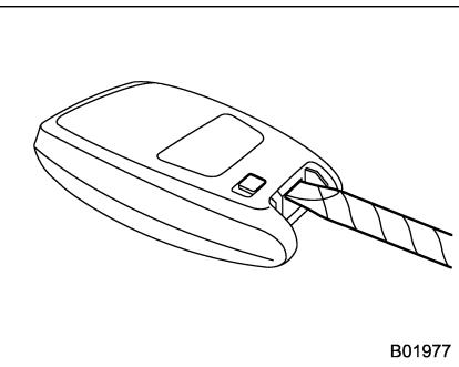
2. Wrap a flat-head screwdriver with vinyl tape or a cloth, and insert it in the gap to remove the cover.
