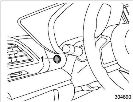
Press the TRIP RESET switch to switch between the displays for the average fuel consumption that corresponds to the A trip meter mileage and the average fuel consumption that corresponds to the B trip meter mileage.
