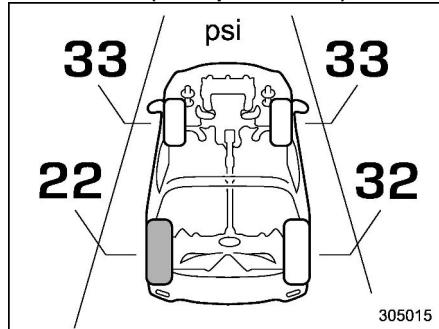
This screen displays each tire pressure. When a tire is deflated, the deflated tire and the tire pressure will be displayed on the screen in yellow.
