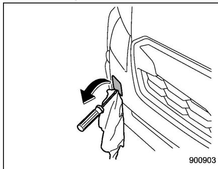
2. Cover the tip of a flat-head screwdriver
