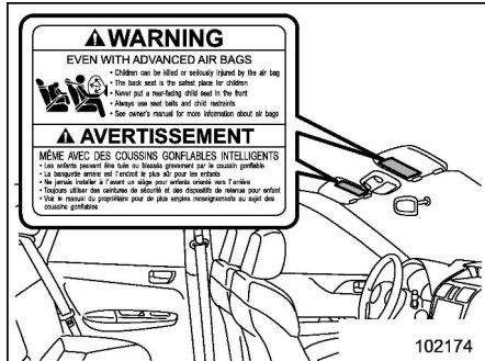
Your vehicle has warning labels on the driver's and front passenger's sun visors beginning with the phrase "EVEN WITH
