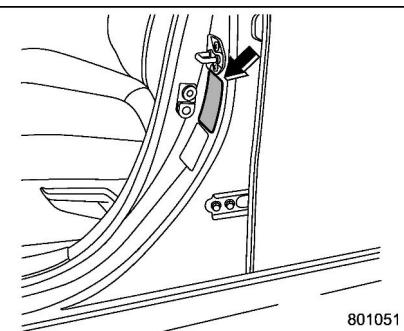
The vehicle placard is attached to the driver's side door pillar.
