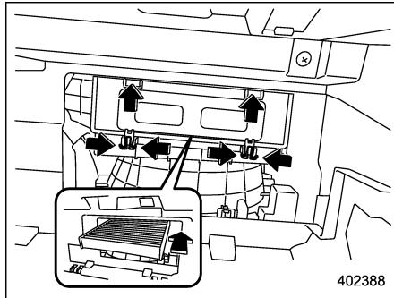
3. Replace the cabin air filter with a new one and then reinstall the cover.
