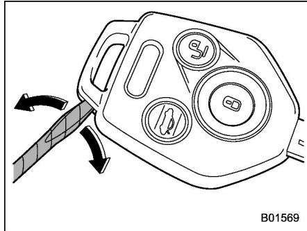
1. Wrap a flat-head screwdriver with vinyl tape or a cloth. Open the key head using a flat-head screwdriver.
