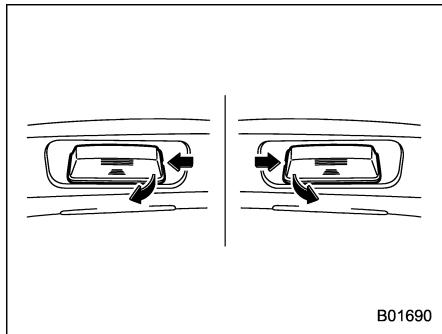
1. The license plate lights must be pushed outwards, and then pulled out to be removed.
