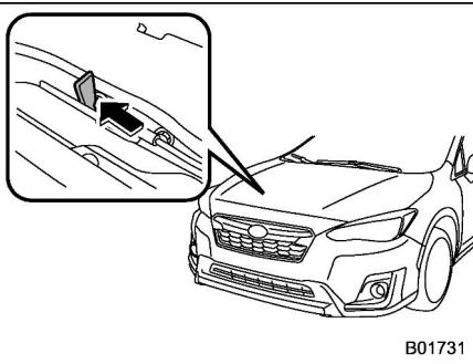
3. Release the secondary hood release by moving the lever between the front grille and the hood toward the left.
