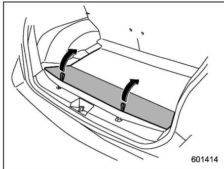
1. Raise and fold the rear end of the cargo floor board.
