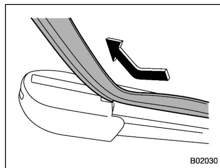
2. Pull the end of the wiper blade rubber through the slit to remove it.
