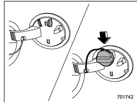
4. Set the fuel filler cap on the cap holder inside the fuel filler lid.
