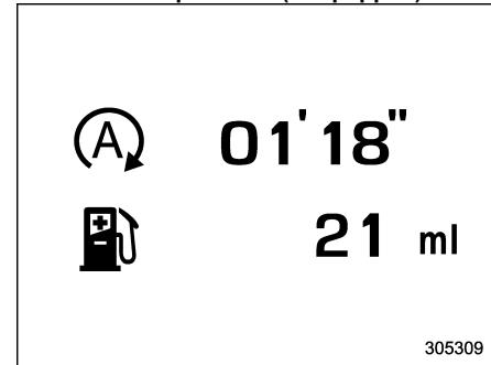
: The total amount of time that the engine was stopped by means of the Auto Start Stop system
