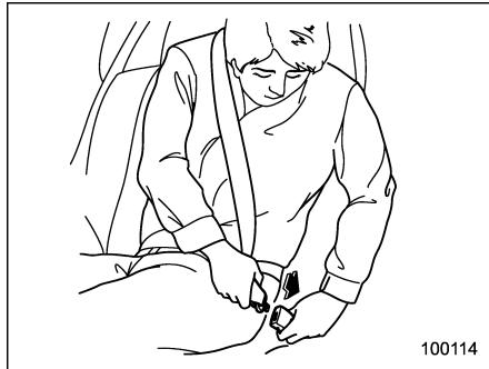
5. Insert the center seatbelt tongue plate into the center seatbelt buckle marked "CENTER" on the left-hand side until it clicks.
