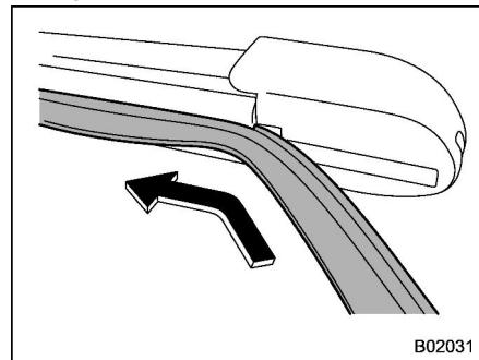
3. Insert a new wiper blade rubber into the slit. Do not insert the wiper blade rubber into the wrong slit.
