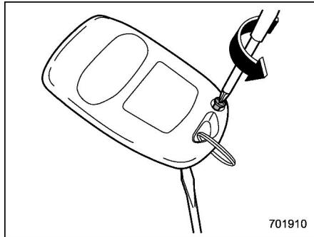
1. Remove the small Phillips screw located on the back side lower left corner of the transmitter.
