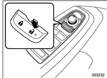
2. Hold down "■" of the power door locking switch.
