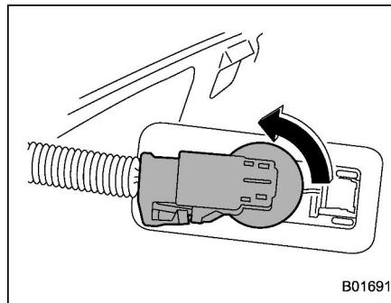
2. Turn the bulb socket counterclockwise and pull out the socket.
