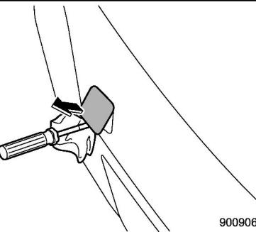
2. Cover the tip of a flat-head screwdriver with vinyl tape or cloth so that it will not scratch the bumper. Pry off the cover on the rear bumper using a screwdriver, and you will find a threaded hole for attaching the towing hook.
