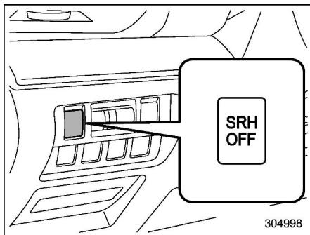
You can turn the SRH function on or off by pressing the SRH OFF switch.
