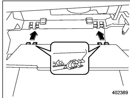
4. Reinstall the glove box, and connect the damper shaft.
