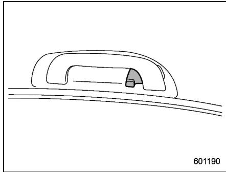
A coat hook is attached to the rear passenger's assist grip.
