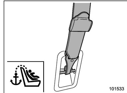
1. Attach the top tether hook to the appropriate upper anchorage.
