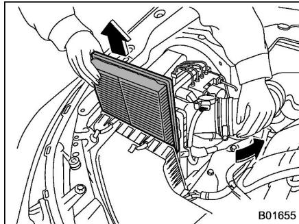
cleaner case (rear) into the slits on the air cleaner case (front).
