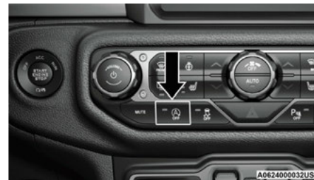
Stop/Start OFF Switch
