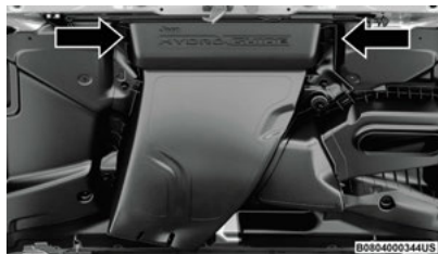
First Water Chamber Removal
