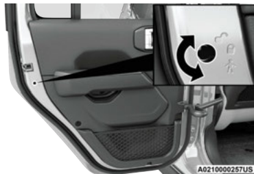
Child-Protection Door Lock Function
