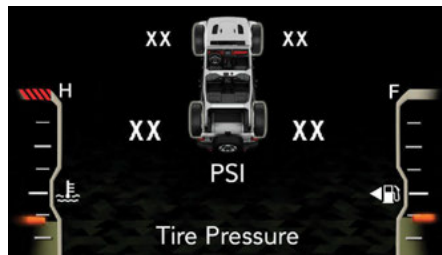
Tire Pressure Monitoring System Display
