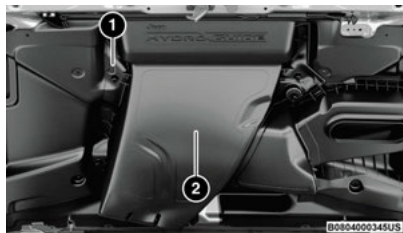
First Water Separation Chamber
