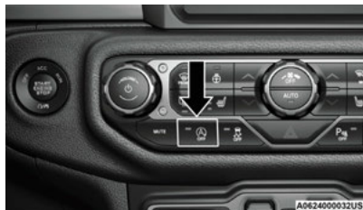
Stop/Start OFF Switch
