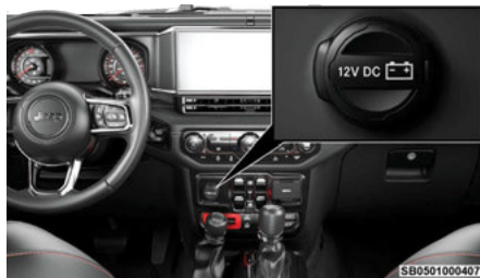
Front Power Outlet
