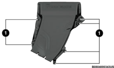
First Water Separation Chamber
