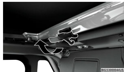
Engage Both Header Latches
