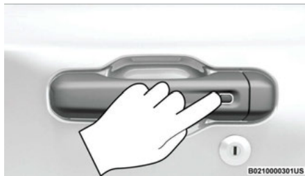
Push The Door Handle Button To Lock
