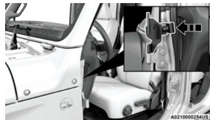
Push Bracket Onto A-pillar
