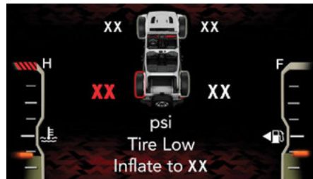
Tire Pressure Monitoring System Low Pressure Warning
