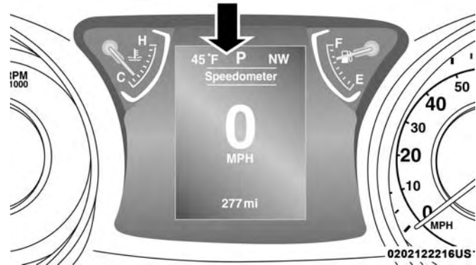
3.5 Inch Instrument Cluster Display Location
