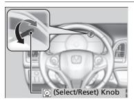
When the ignition switch is in ON III\*1, you can use the (2) (select/reset) knob to adjust instrument panel brightness.
