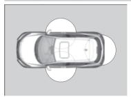
When you carry the keyless remote, you can lock/unlock the doors and the tailgate. You can lock/unlock the doors and the tailgate within a radius of about 32 inches (80 cm) of the outside door or tailgate outer handle.
