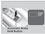
While the system is on, press the automatic brake hold button again.
