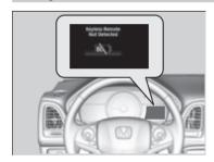
When the power mode is set to any mode other than OFF and you remove the keyless remote from the vehicle and shut the door, an alarm will sound. If the alarm continues to sound, place the keyless remote in another location.
