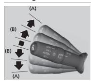
The turn signals can be used when the ignition switch is in ON  $\overline{II}$ <sup>\*1</sup>.
