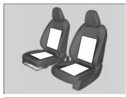
The ignition switch must be in ON  $\overline{II}^{*1}$  to use the seat heaters
