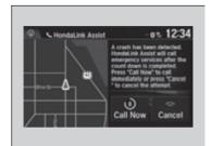
If your vehicle's airbags deploy or if the unit detects that the vehicle is severely impacted, your vehicle automatically will attempt to connect to the HondaLink® operator. If connected, information about your vehicle, its location, and its condition can be sent to the operator\*1; you also can speak to the operator when connected.
