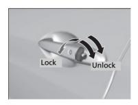
If the lock or unlock button of the remote does not work, use the key instead. Fully insert the key and turn it.
