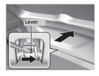
**3.** To open the tailgate, push the tailgate while sliding the lever to the right.
