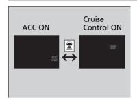
Press and hold the (Interval) button for one second. Cruise Mode Selected appears on the multi-information display for two seconds, and then the mode switches to Cruise. To switch back to ACC, press and hold the (Interval) button again for one second. ACC Mode Selected appears on the multi-information display for two seconds.
