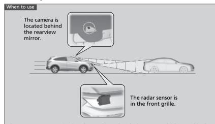
The system starts monitoring the roadway ahead when your vehicle speed is about 3 mph (5 km/h) or above and will search for a vehicle in front of you.
