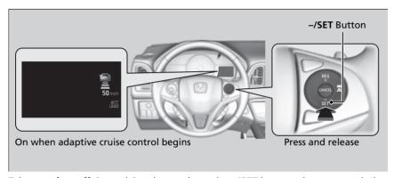
Take your foot off the pedal and press down the **-/SET** button when you reach the desired speed. The moment you release the button, the set speed is fixed, and ACC begins.
