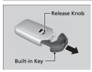
The built-in key can be used to lock/unlock the doors when the keyless remote battery becomes weak and the power door lock/unlock operation is disabled.
