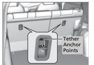
A tether anchor point is provided behind the rear outer seating positions and in the ceiling for the rear center. If you have a child seat that comes with a tether but can be installed with a seat belt, the tether may be used for additional security.
