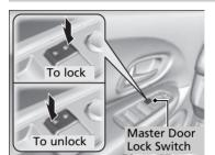
Press the master door lock switch in as shown to lock or unlock all the doors and the tailgate.
