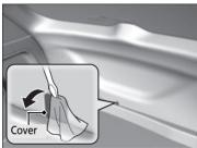
**1.** Wrap a cloth around the flat-tip screwdriver. Put it into the cover as shown in the image, and open it.
