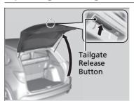
When all the doors are unlocked or you press the tailgate unlock button on the remote transmitter, the tailgate is unlocked. Press the tailgate release button and lift open the tailgate.
