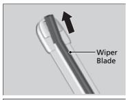
**3.** Slide the wiper blade out of the holder by pulling the tabbed end out.
