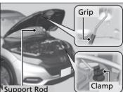
**4.** Remove the support rod from the clamp using the grip. Mount the support rod in the hood.
