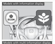
The **ECON** button turns the ECON mode on and off. The ECON mode helps you improve your fuel economy by adjusting the performance of the engine, transmission, heating and cooling system\*/climate control system\*, and cruise control\*.
