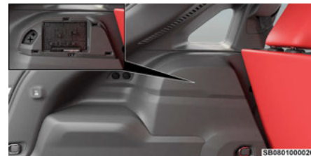
Rear Power Distribution Center Location
