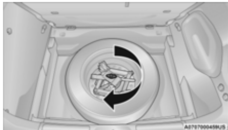
Reinstalling Jack and Tire Fastener
