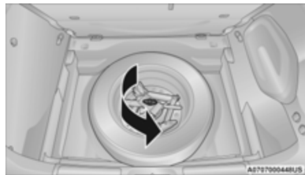
Removing Jack And Spare Tire Fastener
