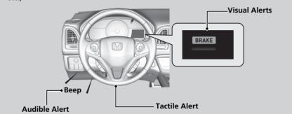
You can change the distance (**Long/Normal/Short**) between vehicles at which the system's earliest collision alert will come on through audio/information screen setting options.
