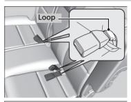
Separately lift up the left and right halves of the rear seat cushions to make room for cargo area.
