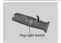
When the low beam headlights are on, turn the fog light switch on to use the fog lights.
