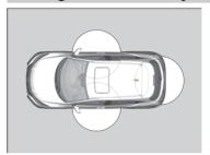
When you carry the smart entry remote, you can lock/unlock the doors and the tailgate. You can lock/unlock the doors and the tailgate within a radius of about 32 inches (80 cm) of the outside door or tailgate outer handle.
