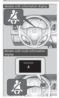
The seat belt system includes an indicator on the instrument panel to remind the driver or a front passenger or both to fasten their seat belts.
