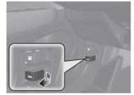
2 Locate the hood latch lever, push it to the side, and then raise the hood. Once you have raised the hood slightly, you can release the lever.
