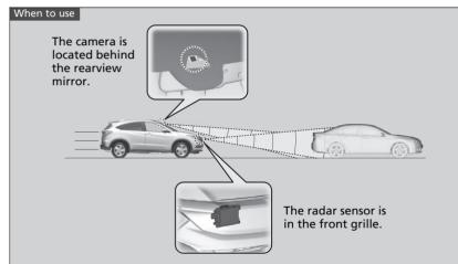
The system starts monitoring the roadway ahead when your vehicle speed is about 3 mph (5 km/h) and there is a vehicle in front of you.
