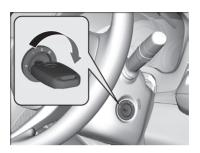
**3.** Turn the ignition switch to START **III** without depressing the accelerator pedal.
