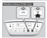
Select the ricon to turn the air conditioning system on and automatically switch the system to fresh air mode.
