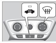
Selecting turns the air conditioning system on and automatically switches the system to fresh air mode.
