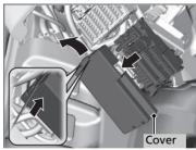
Remove the cover by putting the flat-tip screwdriver into the side slot as shown.
