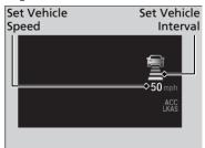
When ACC starts operating, the vehicle icon, interval bars and set speed appear on the multi-information display.
