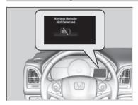
When the power mode is set to any mode other than OFF and you remove the smart entry remote from the vehicle and shut the door, an alarm will sound. If the alarm continues to sound, place the smart entry remote in another location.
