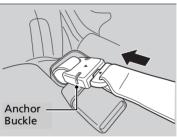
**2.** Line up the triangle marks on the small latch plate and anchor buckle. Make sure the seat belt is not twisted. Attach the belt to the anchor buckle.
