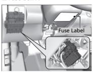
Located behind the instrument panel. Fuse locations are shown on the label under the steering column.
