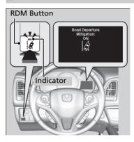
Press the RDM button to turn the system on and off.
