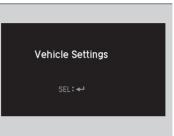
1. Press the ▲①/▼ button until Vehicle Settings appears on the display, then press the SEL/RESET button.
