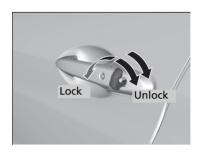
If the lock or unlock button of the remote does not work, use the key instead. Fully insert the key and turn it.
