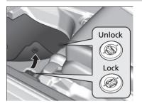
The driver's floor mat hooks over the floor anchors, which keep the mat from sliding forward. To remove a mat for cleaning, turn the anchor knobs to the unlock position. When reinstalling the mat after cleaning, turn the knobs to the lock position.
