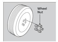
1. Remove the wheel nuts and flat tire.
