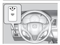
Press the heated windshield button to deice the windshield when the ignition switch is turned to ON  $\overline{II}$ <sup>\*1</sup>.
