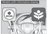
The **ECON** button turns the ECON mode on and off. The ECON mode helps you improve your fuel economy by adjusting the performance of the engine, transmission, heating and cooling system\*/climate control system\*, and cruise control\*.
