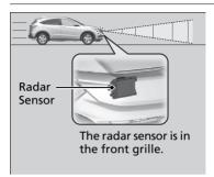
The radar sensor is in the front grille.
