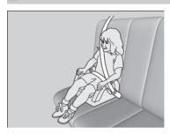
If a lap/shoulder seat belt cannot be used properly, position the child in a booster seat in a rear seat. For the child's safety, check that the child meets the booster seat manufacturer's recommendations.
