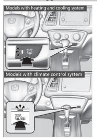
Press the rear defogger button or touch the icon to defog the rear window and mirrors\* when the ignition switch is in ON  $\boxed{II}^{*1}$ .
