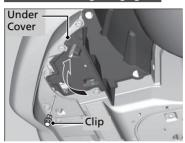
**1.** Remove the clips using a flat-tip screwdriver, and push up the under cover.
