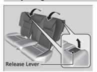
Pull the lever on the right to change the angle of the right half of the seat-back, and left for the left half.
