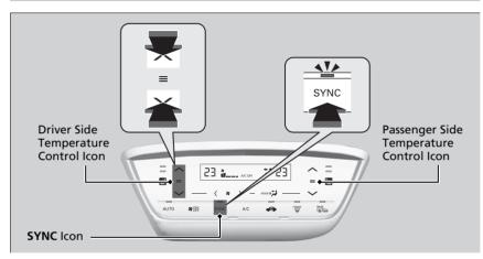
You can set the temperature synchronously for the driver side and the passenger side in synchronization mode.
