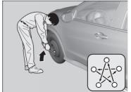
**5.** Lower the vehicle and remove the jack. Tighten the wheel nuts in the order indicated in the image. Go around, tightening the nuts, two to three times in this order.
