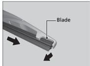
**3.** Slide the wiper blade out of the end with the indent.
