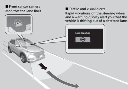
When you operate the turn signals to change lanes, the system is suspended, and resumes after the signals are off.
