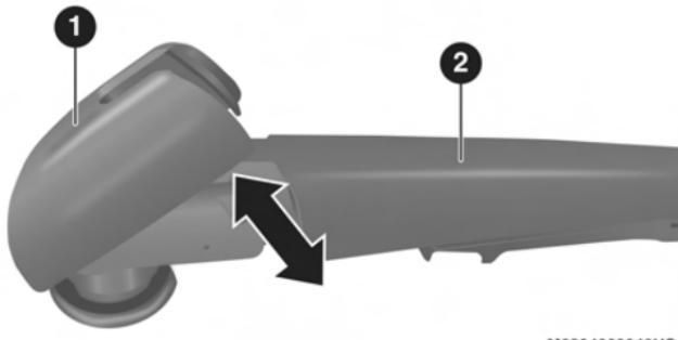
**Wiper Pivot Cap In Unlocked Position**
