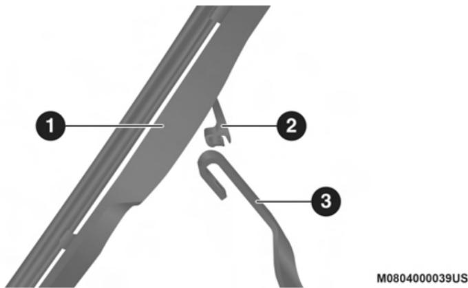
**Wiper Blade Removed From Wiper Arm**
