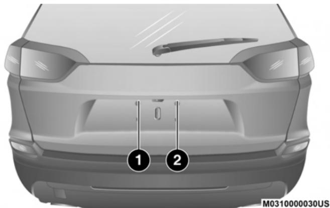
**Liftgate Passive Entry / Release Handle Location**
