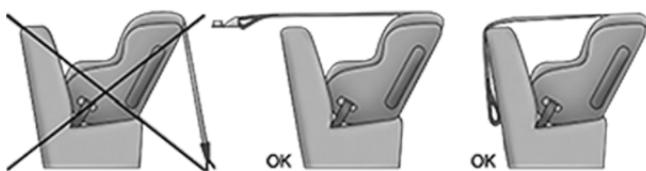
1. Look behind the seating position where you plan to install the child restraint to find the tether anchorage. You may need to move the seat forward to provide better access to the tether anchorage. If there is no top tether anchorage for that seating position, move the child restraint to another position in the vehicle if one is available.
