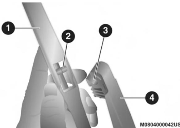
**Wiper Blade Removed From Wiper Arm**
