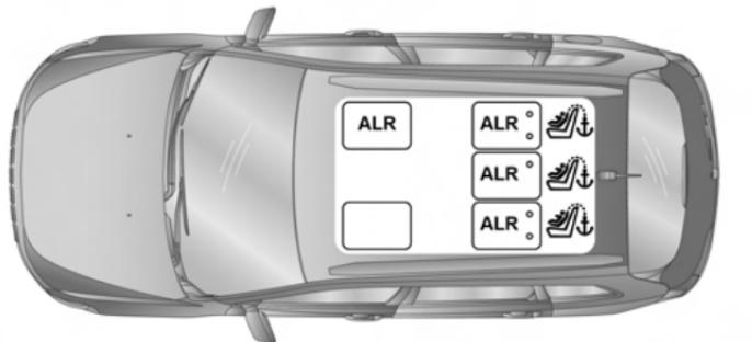
**ALR — Switchable Automatic Locking Retractor (Sliding Seat)**
