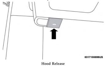
2. Move to the outside of the vehicle and pull the safety latch release lever forward (toward you). The safety latch release lever is located behind the front edge of the hood, slightly off-center to the right.
