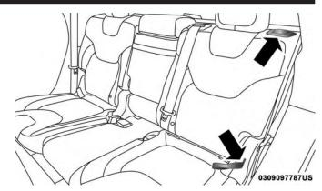
Rear Seatback Release Lever And Pull Strap
