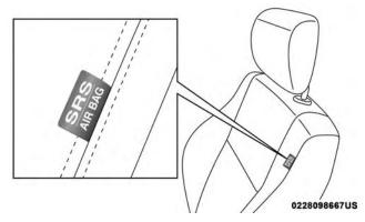
Front Supplemental Seat-Mounted Side Air Bag Label When the SAB deploys, it opens the seam on the outboard side of the seatback's trim cover (front seats) and the seam on the outboard side of the seat cushion's trim cover (outboard rear seats — if equipped with rear SABs). The
