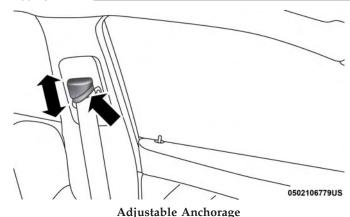
As a guide, if you are shorter than average, you will prefer the shoulder belt anchorage in a lower position, and if you are taller than average, you will prefer the shoulder belt anchorage in a higher position. After you release the anchorage button, try to move it up or down to make sure that it is locked in position.
