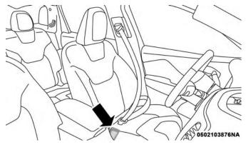
Inserting Latch Plate Into Buckle
