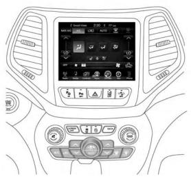
Uconnect 3C/3C NAV With 8.4-inch Display With Automatic Temperature Controls
