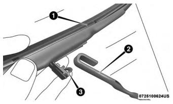
Wiper Blade Removed From Wiper Arm
