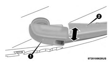
Wiper Pivot Cap In Unlocked Position
