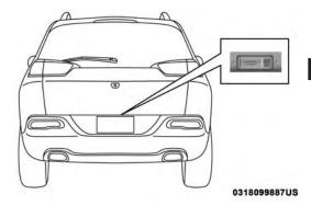
Electronic Liftgate Release/Liftgate Passive Entry Location
