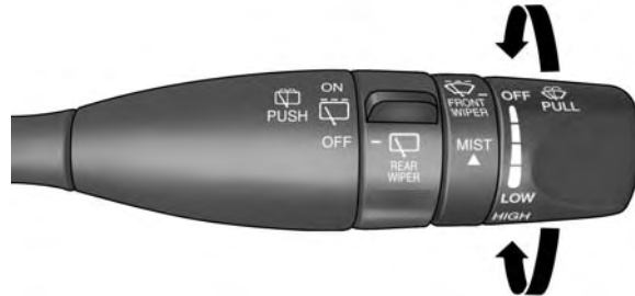
Windshield Wiper Operation
