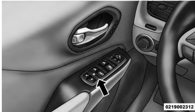
Window Lockout Switch
