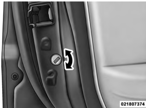
Child-Protection Door Lock Function
