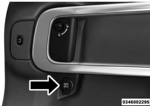
Rear Power Outlet
