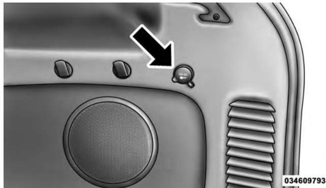
Rear Power Outlet
