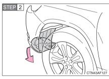
Remove the fender liner.
