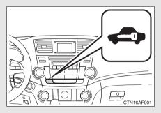
Close the doors and hood, and lock all the doors using the entry function (vehicles with smart key system) or wireless remote control. The system will be set automatically after 30 seconds.
