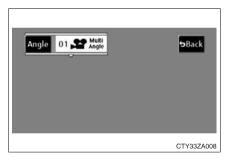
Press or select Angle to display the screen to change the angle.
