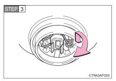
Release the bulb retaining spring.
