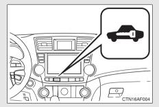
Vehicles without smart key system: The indicator light flashes after the key has been removed from the engine switch to indicate that the system is operating.
