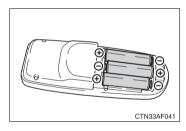
Remove the depleted batteries and install new 3 AA batteries.
