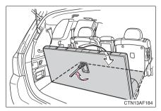
Pull the strap on the third seatback fold-down lever toward you to fold down the seatback.
