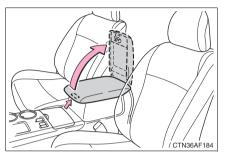
Pull up the knob to release the lock. Lift the lid.
