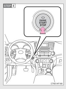
Press the "ENGINE START STOP" switch.
