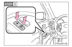
Shift the shift lever to P or N, and press and hold the driver's door lock switch ( or or approximately 5 seconds and then release it.
