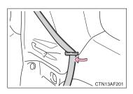
Pass the outer seat belts through the seat belt hangers to prevent the shoulder belts from being damaged.
