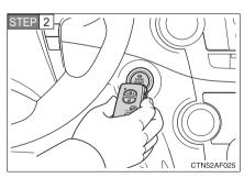
Touch the Toyota emblem side of the electronic to the kev "ENGINE START STOP" switch.
