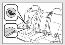
Second seat: Child restraint LATCH anchors
