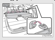
Hang the hooks on the hook brackets on the second seat seatback.
