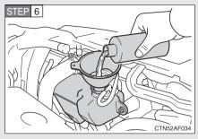
Add engine coolant if necessary.
