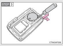
Remove the depleted battery.
