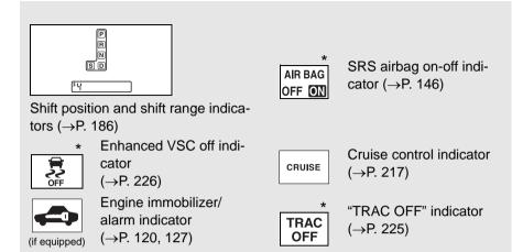
\*: These lights turn on when the engine switch is turned to the "ON" position (vehicles without smart key system) or the "ENGINE START STOP" switch is turned to IGNITION ON mode (vehicles with smart key system) to indicate that a system check is being performed. They will turn off after the engine is started, or after a few seconds. There may be a malfunction in a system if a light does not come on, or if the lights do not turn off. Have the vehicle inspected by your Toyota dealer for details.
