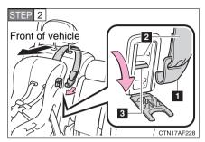
Outside seat: Open the anchor bracket cover, latch the hook onto the anchor bracket and tighten the top tether strap.
