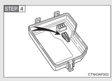
Remove the fuse with the pullout tool.
