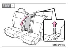
Fold down the second center seatback while pulling the seatback lock release strap.
