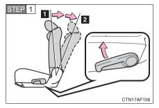
Fold the seatback while pulling the lever. Return the seatback and secure it at the 1st lock position (most upright position). Adjust the seatback to the 3rd lock position.  $(\rightarrow P.~86)$
