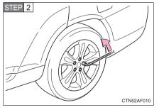
Slightly loosen the wheel nuts (one turn).
