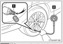
STEP 1 Remove the tire valve cap.
