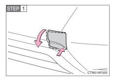
Remove the eyelet cover while pushing it.
