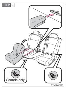
Latch the buckles onto the LATCH anchors.
