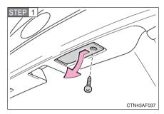
Remove the screw and remove the unit.
