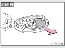
Remove the discharged transmitter battery.
