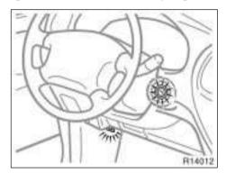
For easy access to the ignition switch, the ignition switch light comes on when the driver's door is opened. The step light also comes on when the driver's door is opened.
