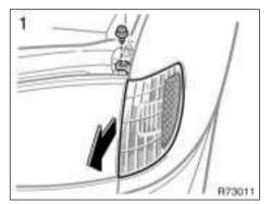
Use a Phillips-head screwdriver. Remove and install the clip as shown in the following illustrations.
