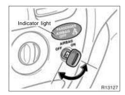
The passenger airbag system is equipped with a manual on-off switch and indicator light. Turning the passenger airbag manual on-off switch clockwise to the "ON" position makes the passenger airbag system operational. Turning the passenger airbag manual on-off switch counterclockwise to the "OFF" position disables the passenger airbag system. The indicator light on the passenger airbag manual on-off switch will come on when the passenger airbag system has been disabled.
