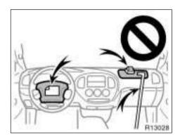
• Do not put objects or your pets on or in front of the dashboard or steering wheel pad that houses the airbag system. They might restrict inflation or cause death or serious injury as they are projected rearward by the force of the deploying airbags. Likewise, the driver and front passenger should not hold objects in their arms or on their knees.
