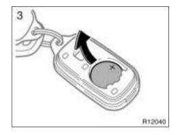
3. Remove the discharged transmitter battery.
