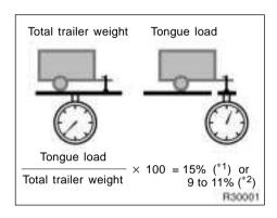
The trailer cargo load should be distributed so that the tongue load is 15% for weight distributing hitch (\*1) or 9 to 11% for weight carrying hitch (\*2) of the total trailer weight, not exceeding the maximum load of the following.
