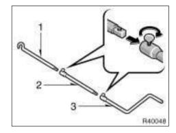
Access cab models—Put a jack handle, jack handle extension and jack handle end together as shown in the illustration.
