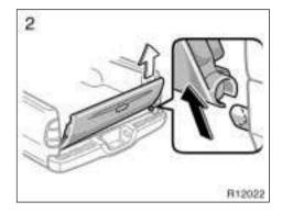
2. Tilt the tailgate to about 30° from vertical and pull up the right side of the tailgate to unhook the right side.
