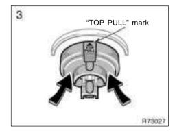
Install the rubber cover with the "TOP PULL" mark upward, and fit it securely on the boss. Then plug in the connector.
