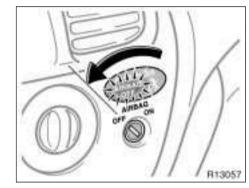
When you put a rear-facing child restraint system on the front seat, turn the passenger airbag manual on-off switch counterclockwise to the "OFF" position. (For details, see "SRS driver airbag and front passenger airbag" in this section.)
