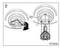
2. Release the bulb retaining spring and remove the bulb. Install a new bulb and the bulb retaining spring.
