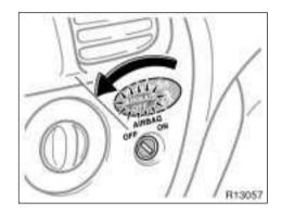
When you install a rear-facing child restraint system which belongs to a passenger risk group on the right front seat, turn the passenger airbag manual on-off switch counterclockwise to the "OFF" position. (For details, see "SRS driver airbag and front passenger airbag" in this section.)
