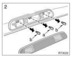
a: High mounted stoplight b: Cargo lamps
