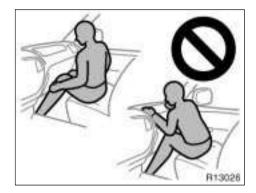
• Do not sit on the edge of the seat or lean over the dashboard when the vehicle is in use, since the airbags inflate with considerable speed and force. Otherwise, you may be killed or seriously injured. Sit up straight and well back in the seat, and always use your seat belt properly.
