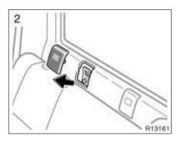
Lightly push down on the top surface of the anchor bracket cover, then pull it forward to remove.
