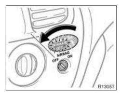
When you put a rear-facing child restraint system on the front seat, turn the passenger airbag manual on-off switch counterclockwise to the "OFF" position. (For details, see "SRS driver airbag and front passenger airbag" in this section.)
