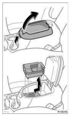
The rear console box is equipped with a compact disc and cassette tape holder.
