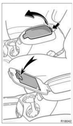
The rear console box is equipped with a note pad holder. This is designed to hold small paper such as note pads.
