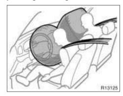
The SRS (Supplemental Restraint System) airbags are designed to provide further protection for the driver and right front passenger in addition to the primary safety protection provided by the seat belts.
