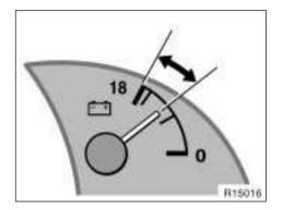
The voltmeter tells whether the battery is charged or discharged. Check it while the engine is running—the needle should always indicate as shown above.
