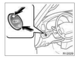
The rear window can be operated with the switch on the instrument panel.
