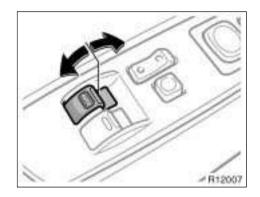
The windows can be operated with the switch on either front door.
