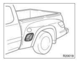
The side step is for easier step-up loading.
