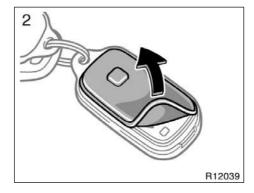
2. Remove the rubber gasket and set it aside.
