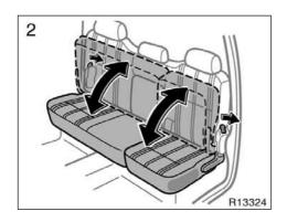
2. Raise the bottom cushion while pushing the lock release lever.
