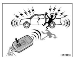
Pushing the "PANIC" switch blows the horn intermittently and flashes the headlights and tail lights.
