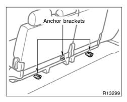
Use one anchor bracket on the back of rear seats and two anchor brackets on the floor as shown above to attach the top strap.
