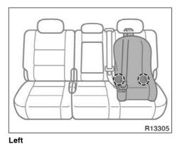
Lower anchorages for the child restraint systems complying with the FMVSS225 or CMVSS210.2 specifications are installed in the center and left positions of the rear seats.
