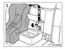
Route the top strap through the slot on top of the seat, pass the strap through the seat, then latch the hook onto the anchor bracket.
