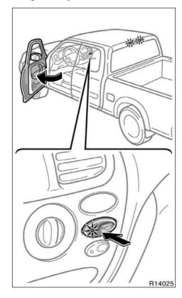
The cargo lamp is designed to light up the rear deck of your vehicle.
