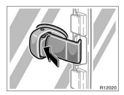
To open the back window, push the lever and slide the window.
