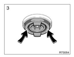
Install the rubber cover as shown, and fit it securely on the boss. Then plug in the connector.
