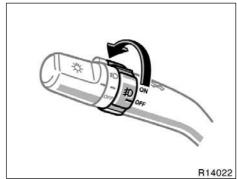
To turn on the front fog lights, twist the band of the headlight/turn signal lever. They will come on only when the headlights are on low beam.
