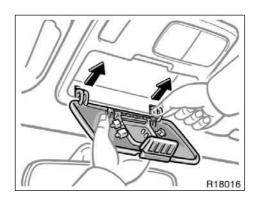
Standard and access cab models only— The auxiliary box (stored in the glove box) and garage door opener box are interchangeable.
