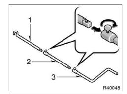
Access and double cab models—Put a jack handle, jack handle extension and jack handle end together as shown in the illustration.
