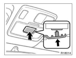
When the garage door opener transmitter is properly installed, you can operate the transmitter by pushing the center panel of the cover.
