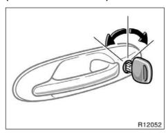
When all the doors are unlocked simultaneously using a key, the interior light, ignition switch light, step light come on for about 15 seconds and cargo lamp for about 20 seconds before fading out. (For details, see "Center interior and personal lights", "Ignition switch and step lights" and "Cargo lamp" in Section 1–5.)
