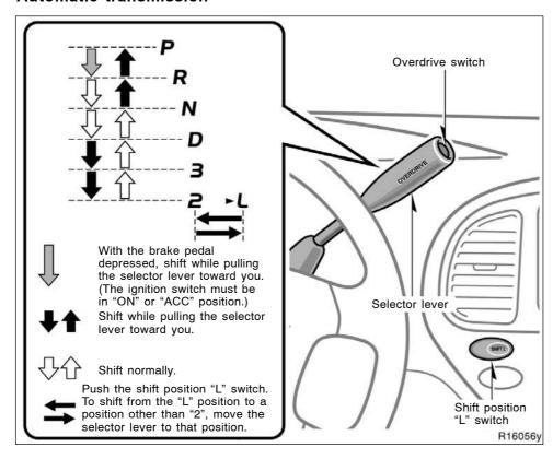
Your automatic transmission has a shift lock system to minimize the possibility of incorrect operation. This means you can only shift out of "P" position when the brake pedal is depressed (with the ignition switch in "ON" or "ACC" position and the selector lever pulled toward you).
