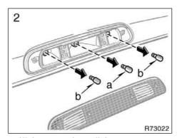
a: High mounted stoplight b: Cargo lamps
