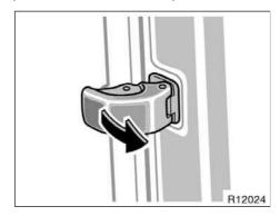
To open the rear side window, pull the latch handle toward you and swing it fully out.
