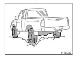
The "AUTO LSD" system aids traction by using the traction control system to control engine performance and braking when one of the rear wheels begins to spin.
