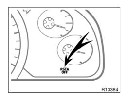
The seat belt pretensioners will not operate in a vehicle rollover if the "RSCA OFF" indicator light is on. For details, see "Roll sensing of curtain shield airbags off switch" in this Section.
