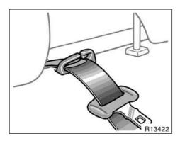
Make sure the shoulder belt pass through the guide when returning the seatback.
