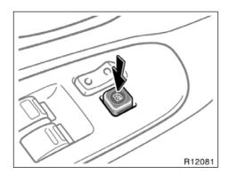
Access cab models only—If you push in the window lock switch on the driver's door, the back window cannot be operated.
