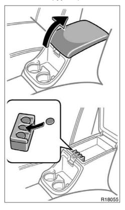
The rear console box is equipped with a coin holder.
