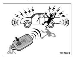
Pushing the "PANIC" switch blows the horn intermittently, flashes the tail lights, and turns on the interior light.
