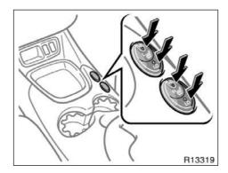
To turn on the seat heater, push the switch ("L" switch for the left front seat and "R" switch for the right seat).
