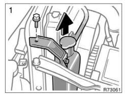
LEFT SIDE PARKING LIGHT—Loosen the bolt and remove the engine coolant reservoir.
