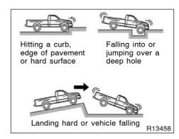
The SRS airbags may also deploy if a serious impact occurs to the underside of your vehicle. Some examples are shown in the illustration.
