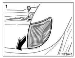
Use a Phillips-head screwdriver. Remove and install the clip as shown in the following illustrations.
