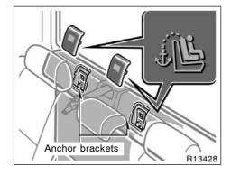
Use the anchor bracket on the back panel to attach the top strap.
