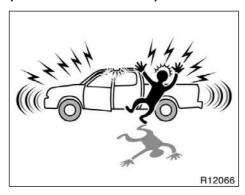
To deter vehicle theft, the system is designed to sound an alarm if any of the doors or hood is forcibly unlocked or opened or the battery terminal is disconnected and then reconnected when the vehicle is locked.
