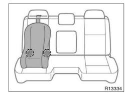
Lower anchorages for the child restraint systems complying with the FMVSS225 or CMVSS210.2 specifications are installed in the front seat.
