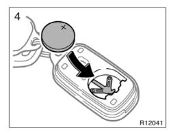
4. Put in a new transmitter battery with positive (+) side up.
