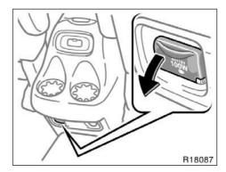
This power outlet (115 VAC) is designed for use as a power supply for electric appliances in the vehicle.
