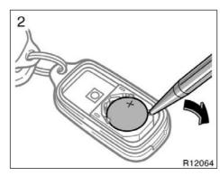
2. Remove the discharged transmitter battery.
