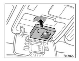
Place the transmitter with Velcro square facing inside of box into the box. Make sure the transmitter button is located above button pins.
