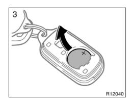
3. Remove the discharged transmitter battery.
