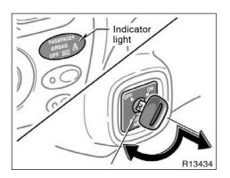
The passenger airbag system is equipped with a manual on-off switch and indicator light. Turning the passenger airbag manual on-off switch clockwise to the "ON" position makes the passenger airbag system operational. To disable the passenger airbag system, turn the manual on-off switch counterclockwise to the "OFF" position and remove the key. The indicator light on the passenger airbag manual on-off switch will come on when the passenger airbag system has been disabled.
