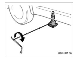
After making sure that no one is in the vehicle, raise it high enough so that the temporary spare tire can be installed.
