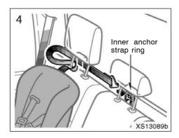
Latch the hook onto the inner anchor strap ring and tighten the top strap.
