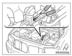
Connecting point for 5.7 L V8 (3UR-FE) engine
