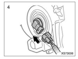
4. Install the connector to the bulb.
