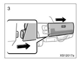
Tilt the tailgate up to about 15° open and slide the tailgate a little to the right to unhook the left side.
