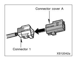
4. Attach the connector cover A (gray) to the connector 1 (white).
