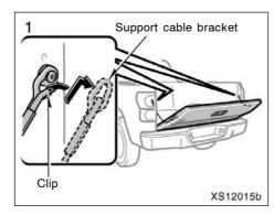
Open the tailgate to the angle where you can release the brackets on the support cables from the lugs on both sides.
