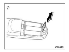
2. Remove the insulating sheet.
