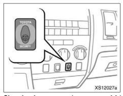
Glass breakage sensor (on some models)
