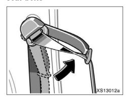
USING FRONT SEAT BELT HANGERS (Regular cab models)
