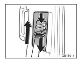
Seat belts with an adjustable shoulder anchor (Double cab and Crew Max models)—
