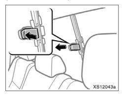
To open the rear window, push the lever and slide the window.
