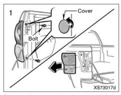
Remove the covers (seal type) and bolts.
