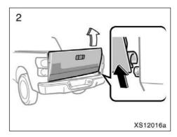
Tilt the tailgate to about 45° from vertical and pull up the right side of the tailgate to unhook the right side.
