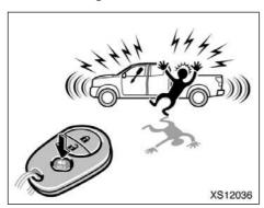
Holding the " (alarm) switch blows the horn intermittently and flashes the headlights, tail lights, turn signal lights, interior light and personal lights.
