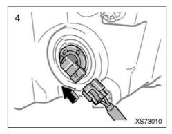
**4. Install the connector to the bulb.**If the battery has been moved, reinstall the battery and check that the battery is installed securely by wiggling it.
