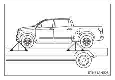
If you use chains or cables to tie down your vehicle, the angles indicated by triangles must be  $45^{\circ}$ .
