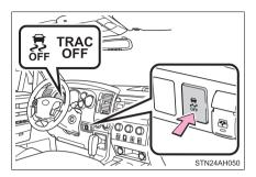
Stop the vehicle completely, and press the VSC OFF switch for more than 3 seconds.
