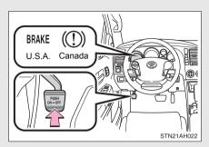
the Sets parking brake\*. (Depressing the pedal again releases the parking brake.)
