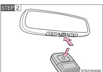
Point the remote control transmitter for the device 1 to 3 in. (25 to 75 mm) from the HomeLink® control buttons.
