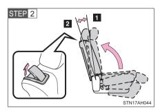
Fold down the seatback and back to the 1st lock position (most upright position) until it locks into place. Adjust the seatback to the 8th lock position.  $(\rightarrow P. 63)$
