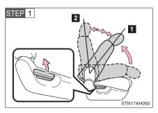
Fold down the seatback and back to the 1st lock position (most upright position) until it locks into place. Adjust the seatback to the 13th lock position.  $(\rightarrow P. 61)$
