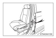
For the GAWR, see the Certification Label. For the maximum load of the tire, see the load limit at maximum cold tire inflation pressure mentioned on the sidewall of the tire. ( $\rightarrow$  P. 672)
