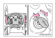
When starting the engine, the engine switch may seem stuck in the LOCK position. To free it, turn the key while turning the steering wheel slightly in either direction.
