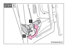
Loosen and remove the jack.
