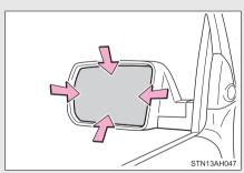
Adjust the mirror up, down, in or out by pushing the mirror surface.
