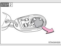
Remove the discharged transmitter battery.
