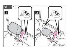
Remove the head restraint.
