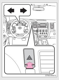
Press the switch to flash all the turn signal lights. To turn them off, press the switch once again.
