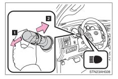
With the headlights on, push the lever forward to turn on the high beams.
