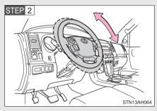
Adjust to the ideal position by moving the steering wheel vertically.
