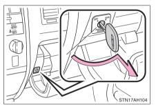
Turn the passenger airbag off switch counterclockwise to the OFF position and remove the key.
