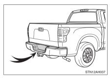
For rear end protection and easier step-up loading.
