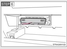
Pull the filter out of the filter outlet.
