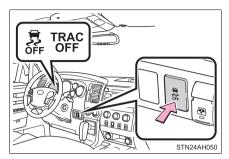
Stop the vehicle completely, and press the VSC OFF switch for more than 3 seconds, when the system is in the AUTO LSD mode
