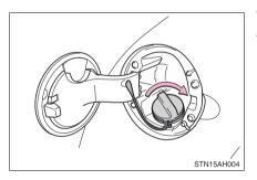
When installing the fuel tank cap, turn it until you hear a click.
