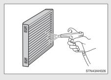
If the filter is dirty, clean by blowing compressed air through the filter from the downward side.
