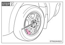
Slightly loosen the wheel nuts (one turn).
