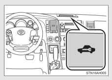
Close the doors and hood, and lock all the doors. The system will be set automatically after 30 seconds.
