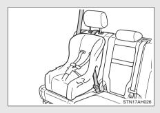
Seat belts equipped with a child restraint locking mechanism (ALR/ELR belts except driver's seat belt) (→P. 79)
