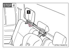
Latch the hook onto the inner anchor strap ring and tighten the top tether strap.
