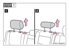
Remove the head restraint.
