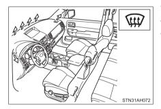
When the dial is set to \( \text{\text{\$\psi}} \), air flows to the windshield and side windows.
