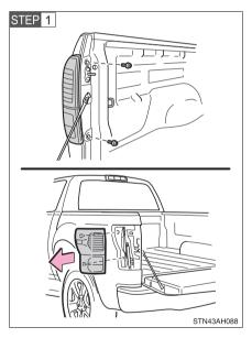
Remove the bolts and rear combination assembly.
