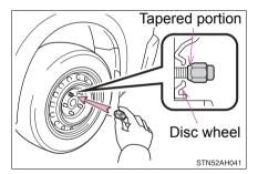
Tighten the nuts until the tapered portion comes into loose contact with the bolt seat in the disc wheel.
