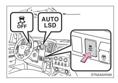
Stop the vehicle completely, and press the VSC OFF switch for more than 3 seconds, when the system is in the TRAC OFF mode.
