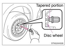
Tighten the nuts until the tapered portion comes into loose contact with the bolt seat in the disc wheel.
