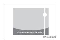
If a bright light, such as sunlight reflected off the vehicle body, is picked up by the camera, a smear effect\* characteristic to the camera may occur.
