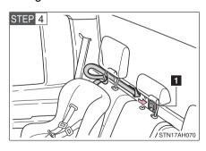
Latch the hook onto the inner anchor strap ring and tighten the top tether strap.
