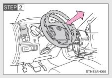
Adjust to the ideal position by moving the steering wheel horizontally.
