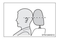
Make sure that the head restraints are adjusted so that the center of the head restraint is closest to the top of your ears.
