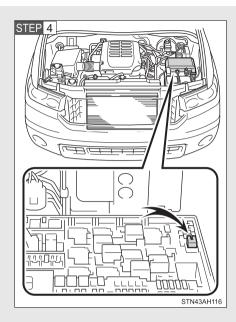
Remove the fuse with the pullout tool.
