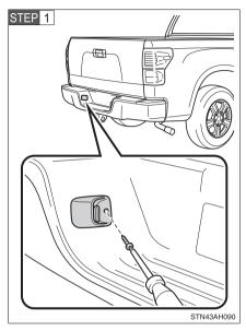
Remove the screw and light unit.
