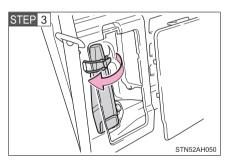
Unhook the strap and remove the tool bag.
