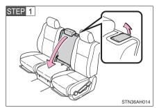
Pull the lever up and fold down the seatback.
