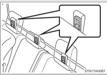
▶ Double Cab models Anchor brackets are provided for all rear passenger seats.
