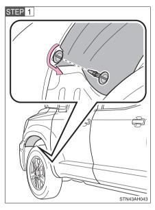
Remove the fender liner clip.
