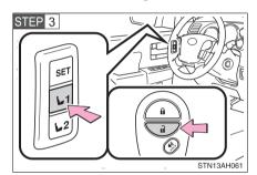
Push the "1" or "2" button and the button on the wireless remote control at the same time for about 1 second until you hear a beep.
