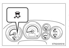
If the rear wheels spin, the slip indicator flashes to indicate that the AUTO LSD system has controlled the spinning of the rear wheels.
