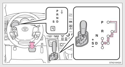
While the engine switch is on, depress the brake pedal and move the shift lever.
