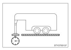
The load placed on the 5th wheel mount or the gooseneck ball.  $(\rightarrow P. 275)$
