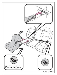
LATCH anchors and tighten the lower straps.
