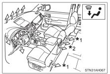
When the dial is set to , air flows to the feet and the windshield defogger operates.
