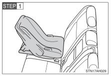
Place the child seat on the rear seat facing the rear of the vehicle.
