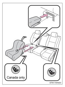
STEP 2 Latch the buckles onto the LATCH anchors.
