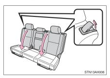
Pull the lever to unlock the seatback and fold the seatback down until it locks.
