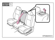
Pull the lever up and fold down the seatback.
