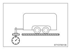
The load placed on the trailer hitch ball.  $(\rightarrow P. 275)$
