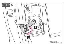
Loosen and remove the jack.
