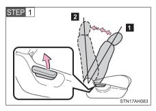
Fold the seatback while pulling the lever. Return the seatback and secure it at the 1st lock position (most upright position). Adjust the seatback to the 13th lock position. (→P. 61)
