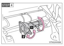
Unhook the strap. Loosen and remove the jack.
