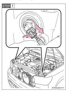
Unplug the connector while depressing the lock release.
