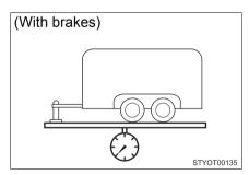
The maximum allowable gross trailer weight. The gross trailer weight is the sum of the trailer weight and the weight of the cargo in the trailer.
