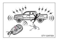
When NoLD is pushed for longer than about one second, an alarm will sound for about 60 seconds and the vehicle lights will flash to deter any person from trying to break into or damage your vehicle.
