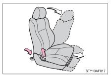
Lift the seatback angle adjusting lever or press the pedal behind the seatback. The seat will slide forward.
