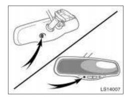
To ensure correct functioning of antiglare mirror sensors located on both sides of the mirror, do not touch or cover the sensors with your finger or a piece of cloth, etc.
