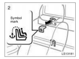
Lightly push down on the top surface of the routing device cover with the symbol mark shown in the illustration, then pull it forward to remove.
