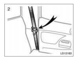
Make sure the shoulder belt passes through the hanger when folding the rear seat.
