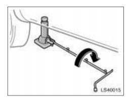
7. After making sure that no one is in the vehicle, raise it high enough so that the spare tire can be installed.
