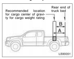
The figures given in the illustration indicate the recommended center of gravity zone.
