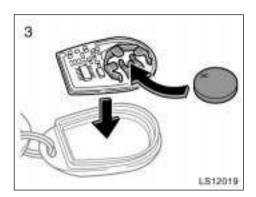
3. Put in a new transmitter battery with positive (+) side up. Install the circuit board into the transmitter case.
