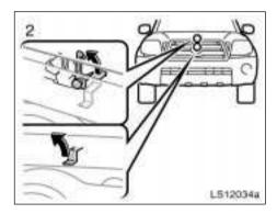
2. Pull up the auxiliary catch lever inside the engine compartment, and lift the hood. (by inserting your finger through either the opening between the hood and grille or through the grille.)
