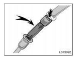
To connect the extender to the seat belt, insert the tab into the seat belt buckle so that the "PRESS" signs on the buckle release buttons of the extender and the seat belt are both facing outward as shown.
