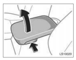
To use the rear console box, raise the console box lid while pushing the lock release button.
