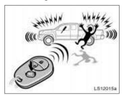
Pushing the "==" (alarm) switch blows the horn intermittently and flashes the headlights, tail lights, turn signal lights, and interior light.
