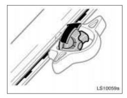
4. Tighten the thumb wheel in a clockwise motion until the clutch mechanism ratchets.
