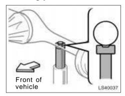
6. After making sure that no one is in the vehicle, as the jack touches the vehicle and begins to fit, double-check that it is properly positioned.
