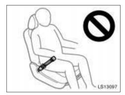
• If the seat belt extender has been connected to the driver's seat belt buckle without the driver actually wearing the seat belt, the SRS driver's airbag system will judge that the driver is wearing it. In this case, the driver's airbag may not activate correctly, causing death or serious injury in the event of collision. Be sure to wear the seat belt with the seat belt extender.
