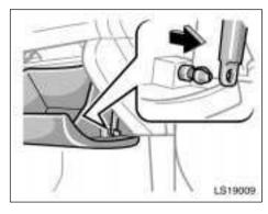
1. Open the glove box, and slide off the damper as shown.
