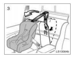
Pull the seatback release lever and swing the seatback forward slightly.Route the top strap through the routing device as shown in the il-
