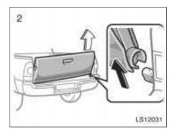
2. Tilt the tailgate to about 30° from vertical and pull up the right side of the tailgate to unhook the right side.
