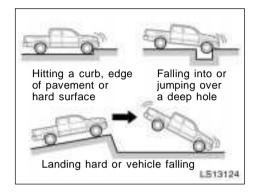
The SRS side and curtain shield airbags may deploy if a serious impact occurs to the underside of your vehicle. Some examples are shown in the illustration.
