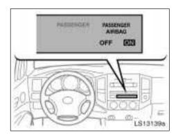
The front passenger occupant classification indicator light indicates the actuation of the front passenger airbag and front passenger seat belt pretensioner.
