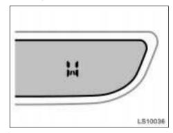
The compass indicates the direction that the vehicle is heading. In the above case, it shows that the vehicle is heading west.
