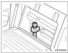
The flashlight holder is designed to hold the flashlight securely.
