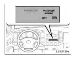
The front passenger occupant classification indicator light indicates the actuation of the front passenger airbag, side airbag on the front passenger seat and front passenger seat belt pretensioner.
