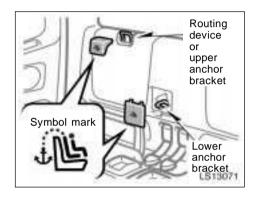
Use the routing device and the anchor bracket to attach the top strap.
