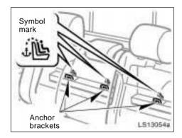
Use the anchor bracket on the back panel to attach the top strap.
