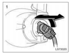
1. Turn the bulb base counterclockwise and remove it.
