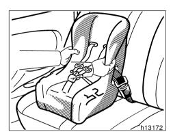
Push and pull the child restraint system in different directions to be sure it is secure. Follow all the installation instructions provided by its manufac-
