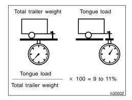
• The trailer cargo load should be distributed so that the tongue load is 9 to 11% of the total trailer weight. not exceeding the maximum load of the following. Without towing package 158 kg (350 lb.)
