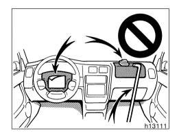
• Do not put anything or any part of your body on or in front of the dashboard or steering wheel pad that houses the airbag system. They might restrict inflation or cause death or serious injury as they are projected rearward by the force of the deploying airbags. Likewise, the driver and front passenger should not hold objects in their arms or on their knees.
