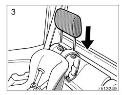
3. Fix the child restraint system with the seat belt and tighten the top strap.
