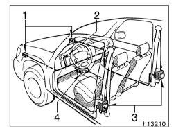
The seat belt pretensioner system consists mainly of the following components and their locations are shown in the illustration.
