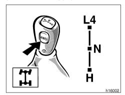
Use the front drive control lever and "4WD" button to select the following transfer modes.
