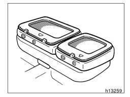
You can use the rear seatback as a temporary table when the vehicle is stopped. See "Seatback table" in Section 1-10 for instructions.
