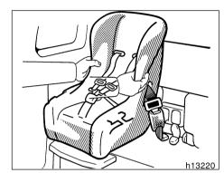
Push and pull the child restraint system in different directions to be sure it is secure. Follow all the installation
