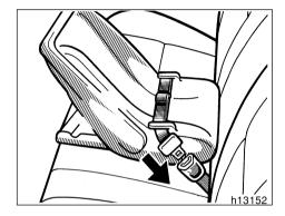
Run the center lap belt through or around the infant seat following the instructions provided by its manufacturer and insert the tab into the buckle taking care not to twist the lap belt.
