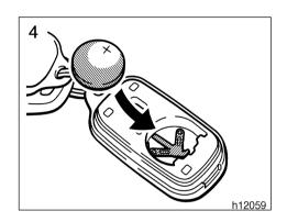
4. Put a new transmitter battery with positive (+) side up.
