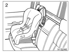
Fix the child restraint system with the seat belt and tighten the top strap.
