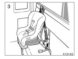
Latch the hook onto the rear lower anchor bracket and tighten the top strap.
