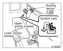
Use the routing device and the anchor bracket to attach the top strap.
