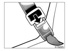
To remove the child restraint system, press the buckle release button and allow the belt to retract.
