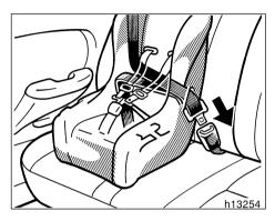
Run the lap and shoulder belt through or around the convertible seat following the instructions provided by its manufacturer and insert the tab into the buckle taking care not to twist the belt. Keep the lap portion of the belt tight.
