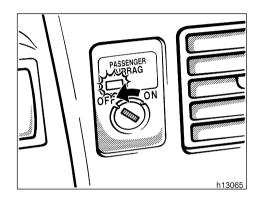
When you install a rear-facing child restraint system on the front passenger seat, turn the passenger airbag manual on-off switch counterclockwise to the "OFF" position. (For details, see "SRS driver airbag and front passenger airbag" in this Section.)
