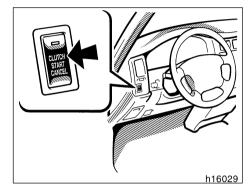
To crank the engine without depressing the clutch pedal, push the switch with the ignition on.
