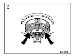
Install the rubber cover with the "TOP PULL" mark upward and fit it securely on the boss. Then plug in the connector.
