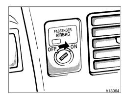
The passenger airbag system is equipped with a manual on-off switch and indicator light. Turning the passenger airbag manual on-off switch clockwise to the "ON" position makes the front passenger airbag system operational. Turning the passenger airbag manual on-off switch counterclockwise to the "OFF" position disables the front passenger airbag system. The indicator light on the passenger airbag manual on-off switch will come on when the front passenger airbag system has been disabled.
