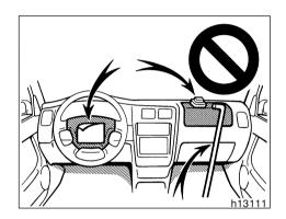
• Do not put anything or any part of your body on or in front of the dashboard or steering wheel pad that houses the airbag system. They might restrict inflation or cause death or serious injury as they are projected rearward by the force of the deploying airbags. Likewise, the driver and front passenger should not hold objects in their arms or on their knees.
