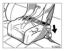
Run the center lap belt through or around the convertible seat following the instructions provided by its manufacturer and insert the tab into the buckle taking care not to twist the lap belt.
