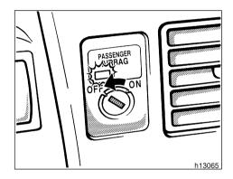
When you install a rear-facing child restraint system which belongs to a passenger risk group on the right front seat, turn the passenger airbag manual on-off switch counterclockwise to the "OFF" position. (For details, see "SRS driver and front passenger airbags" in this Section.)
