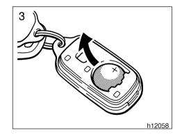
3. Remove the discharged transmitter battery.
