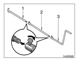
Xtra- cab and double cab models— Put a jack handle, jack handle extension and jack handle end together as shown in the illustration.
