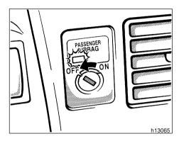
When you install a rear-facing child restraint system on the front passenger seat, turn the passenger airbag manual on-off switch counterclockwise to the "OFF" position. (For details, see "SRS driver airbag and front passenger airbag (vehicles with passenger airbag manual on-off switch)" in this Section.)
