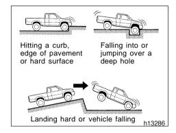
The SRS airbags may also deploy if a serious impact occurs to the underside of your vehicle. Some examples are shown in the illustration.
