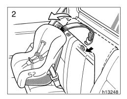
Pull the seatback release lever and swing the seatback forward slightly, then latch the hook onto the anchor bracket.
