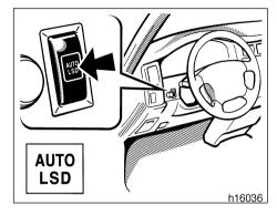
To activate the system, push the "AUTO LSD" switch under the following condition. At this time, the "AUTO LSD" indicator light will come on.
