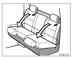
Pull the seatback lock release belt forward and fold down the seat back.
