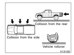
The SRS airbags are generally not designed to inflate if the vehicle is involved in a side or rear collision, if it rolls over, or if it is involved in a low-speed frontal collision. But, whenever a collision of any type causes sufficient forward deceleration of the vehicle, deployment of the SRS airbags may occur.
