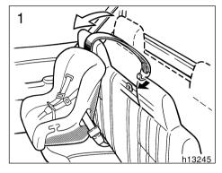
TO USE THE ANCHOR BRACKET: Regular cab with bench seat—
