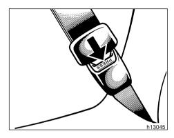
3. To remove the convertible seat, press the buckle release button.
