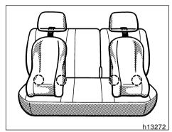
Lower anchorages for the child restraint systems complying with the FMVSS225 or CMVSS210.2 specifications are installed in the outside positions of the rear seat.
