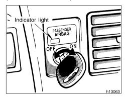
This on-off switch is designed to disable the front passenger airbag in order to allow usage, if necessary, of a member of a passenger risk group identified in TABLE 1 is occupying the right front passenger seating position. (For details, see "SRS driver airbag and front passenger airbag" in this Section.)
