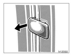
To unlock the rear window, pull the latch handle toward you.
