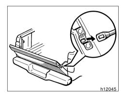
To lower the tailgate fully, release the support brackets from the lugs as shown above.
