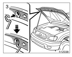
3. Hold the hood open by inserting the support rod into the slot.
