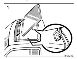
Insert the flat hinges of the moon roof panel into the cutouts on the body. Then slowly lower it to hang the hook into the auxiliary catch while holding the roof with your hands.
