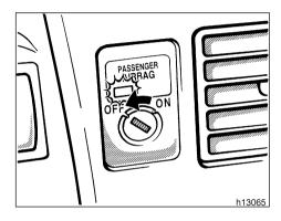
When you install a rear-facing child restraint system on the front passenger seat, turn the passenger airbag manual on-off switch counterclockwise to the "OFF" position. (For details, see "SRS driver and front passenger airbags (vehicles with passenger airbag manual on-off switch)" in this section.)
