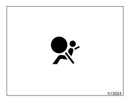
This indicator comes on when the ignition key is turned to the "ON" position. It goes off after about 6 seconds. This means the SRS airbags are operating properly.
