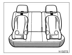
The lower anchorages for the child restraint system interfaced with the FMVSS225 specification are installed in the outside positions of the rear seat.
