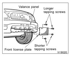
Install the front license plate using the following procedure:
