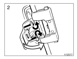
Press in the retaining spring arms and insert them into the holes. Then push the handle up with the palm of your hand and lock the roof.
