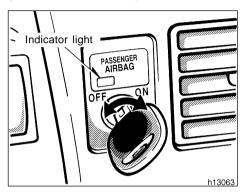
This on-off switch is designed to disable the front passenger airbag in order to allow usage, if necessary, of a member of a passenger risk group identified in TABLE 1 is occupying the right front passenger seating position. (For details, see "SRS driver and front passenger airbags" in this section.)
