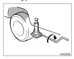
After making sure that no one is in the vehicle, raise it high enough so that the spare tire can be installed.
