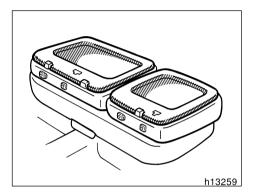
You can use the rear seatback as a temporary table only when the vehicle is stopped.
