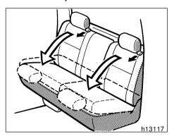
Pull the seatback lock release belt forward and fold down the seat back.
