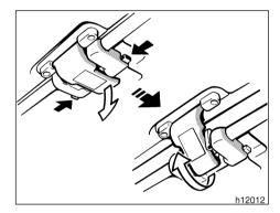
To tilt up the moon roof, first pull down on the handle while pushing in one of the lock buttons. Then push up the moon roof until it locks.
