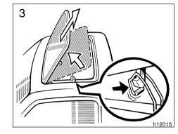
3. Push back the auxiliary catch to release it from the hook. Then lift the moon roof panel and pull it out.
