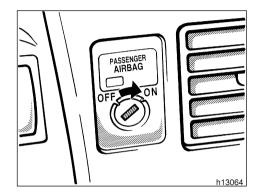
The passenger airbag system is equipped with a manual on-off switch and indicator light. Turning the passenger airbag manual on-off switch clockwise to the "ON" position makes the front passenger airbag system operational. Turning the passenger airbag manual on-off switch counterclockwise to the "OFF" position disables the front passenger airbag system. The indicator light on the passenger airbag manual on-off switch will come on when the front passenger airbag system has been disabled.
