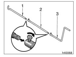
Xtra-cab and double cab models—Put a jack handle, jack handle extension and jack handle end together as shown in the illustration.
