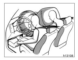
The SRS (Supplemental Restraint System) airbags are designed to provide further protection for occupants in the following seats in addition to the primary safety protection provided by the seat belts.
