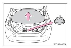
2 Set the jack attachment on the floor jack and position the jack.
