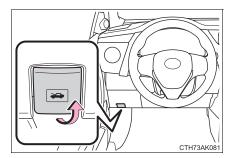
2 Pull up the auxiliary catch lever and lift the hood.
