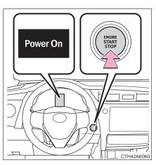
If the engine is stopped with the shift lever in a position other than P, the engine switch will not be turned off but instead be turned to ACCESSORY mode. Perform the following procedure to turn the switch off:
