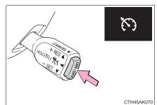
2 Accelerate or decelerate, with accelerator pedal operation, to the desired vehicle speed (at or above approximately 25 mph [40 km/h]) and push the lever down to set the speed.
