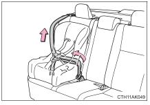
5 If the child restraint has a top tether strap, the top tether strap should be latched onto the top tether strap anchor.  $(\rightarrow P. 63)$
