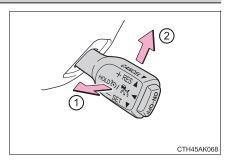
However, cruise control does not resume when the vehicle speed is approximately 25 mph (40 km/h) or less.
