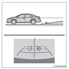
When the ground behind the vehicle slopes down sharply
