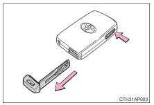
After using the mechanical key, store it in the electronic key. Carry the mechanical key together with the electronic key. If the electronic key battery is depleted or the entry function does not operate properly, you will need the mechanical key. ( $\rightarrow$ P. 523)
