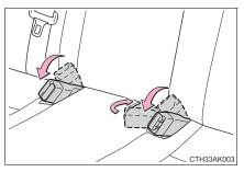
2 Pull the seatback lock release knob and fold the seatback down.
