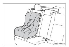
3 Open the anchor bracket cover, latch the hook onto the anchor bracket and tighten the top tether strap.
