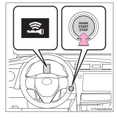
The engine can be started from any engine switch mode.
