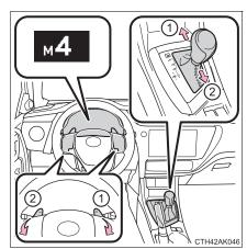
However, even when in the M position, the gear steps will be automatically changed if the engine speed is too high, or too low.
