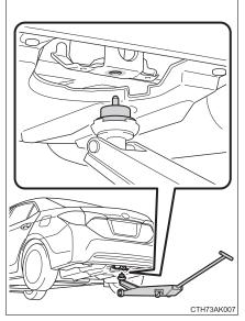
3 Before raising the vehicle, make sure that the floor jack is positioned so that the protrusion on the jack attachment fits securely into the hole of the jack point.
