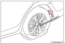
Turn the tire jack portion "A" by hand until the notch of the jack is in contact with the jack point.
