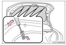
2 Partly remove the trunk panel cover and turn the bulb base counterclockwise.
