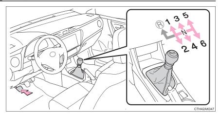
Fully depress the clutch pedal before operating the shift lever, and then release it slowly.
