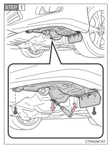
Remove the fender liner bolts and clip.
