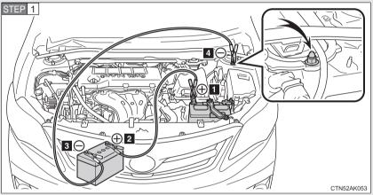
Connecting the jumper cables
