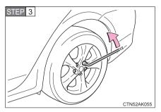
Slightly loosen the wheel nuts (one turn).
