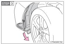
Partly remove the fender liner.
