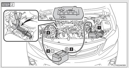
Connecting the jumper cables
