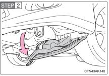
Partly remove the fender liner.
