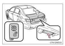
Press the button to unlock the trunk.
