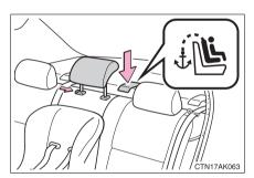
Lock the head restraint in place at the lowest position.
