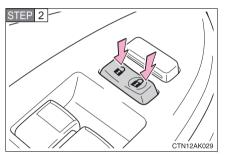
Shift the shift lever to P or N, and press and hold the driver's door lock switch ( or or approximately 5 seconds and then release.
