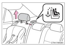
Remove the head restraint.
