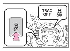
Push and hold the button while the vehicle is stopped to turn off TRAC and VSC.
