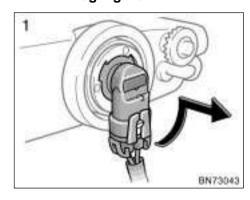
1. Turn the bulb base counterclockwise and remove it.
