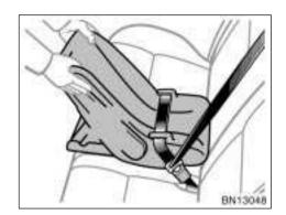
Push and pull the child restraint system in different directions to be sure it is secure. Follow all the installation instructions provided by its manufacturer.
