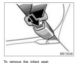
Press the buckle release button and allow the belt to retract completely. The belt will move freely again and be ready to work for an adult or older child passenger.
