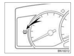
The tire pressure warning light comes on when the ignition key is turned to the "ON" position and goes off after a few seconds. This means the tire pressure warning system is operating properly. If the tire inflation pressure becomes low, the light comes on again. In this case, adjusting the tire inflation pressure will turn off the light after a few minutes. If the light comes on after blinking for 1 minutes, the tire pressure warning system is not working properly.
