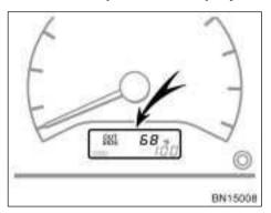
The displayed temperature ranges from  $-30^{\circ}\text{C}$  ( $-22^{\circ}\text{F}$ ) up to  $50^{\circ}\text{C}$  ( $122^{\circ}\text{F}$ ).
