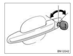
LOCKING AND UNLOCKING WITH KEY Insert the key into the keyhole and turn it.
