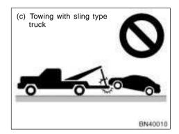
(c) Towing with sling type truck
