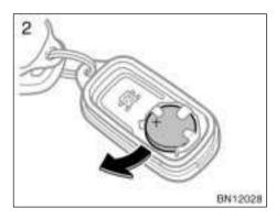
2. Remove the discharged transmitter battery.
