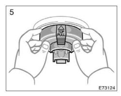
5. Install the rubber cover with the "TOP" mark upward, and snuggle on the boss. Insert the connector.
