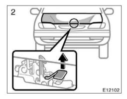
In front of the vehicle, pull up on the auxiliary catch lever and lift the hood.
