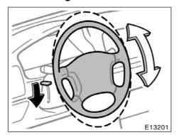
To change the steering wheel angle, hold the steering wheel, pull down the lock release lever, tilt the steering wheel to the desired angle and return the lever to its original position.
