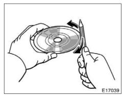
A new disc may have rough edges on its inner and outer perimeter. Remove the rough edges by pressing the side of a ball-point pen or pencil against the inner and outer perimeter of the disc as shown.
