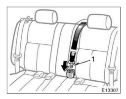
Before returning the seatback to the upright position, make sure to correctly connect the center seat belt for ready use.
