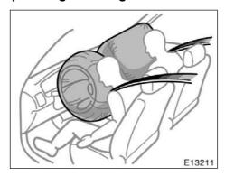
The SRS (Supplemental Restraint System) airbags are designed to provide further protection for the driver and front passenger when added to the primary protection provided by the seat belts.
