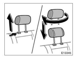
2. Unlock and remove the head restraint, then reinstall it facing backward.
