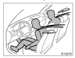
The driver and front passenger's seat belts are equipped with a pretensioner which is designed to be activated together with the front airbags in response to a severe frontal impact.
