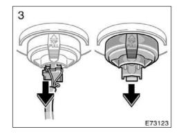
3. Unplug the connector. Remove the rubber cover.
