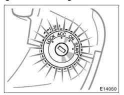
For easy access to the ignition switch, the ignition switch light comes on when any of the doors are opened.
