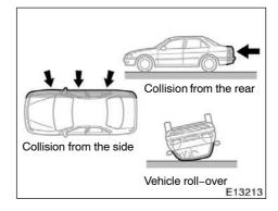
The SRS airbags are not designed to inflate if the vehicle is subjected to a side or rear impact, if it rolls over, or if it is involved in a low-speed frontal collision.
