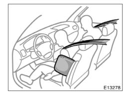
The SRS (Supplemental Restraint System) side airbags are designed to provide further protection for the driver and front passenger when added to the primary protection provided by the seat belts.
