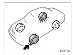
Block the wheel diagonally opposite the flat tire to keep the vehicle from rolling when it is jacked up.
