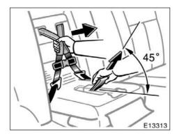
3. While pulling the seat belt release strap (black), pull both shoulder belts together.
