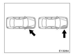
The SRS side airbag system may not inflate if the vehicle is subjected to a collision from the side at an angle, or a collision to the side of the vehicle body other than the passenger compartment shown in the illustration, which impact is not severe enough for the passenger compartment.
