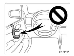
• Do not attach a cup holder or any other device on or around the door. When the side airbag inflates, the cup holder or any other device will be thrown with great force or the side airbag may not activate correctly, resulting in death or serious injury. Likewise, the driver and front passenger should not hold things in their arms or on their knees.
