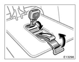
12. To store the built-in child restraint, fasten the shoulder belt clip and return the seat belt buckle using the fastener tapes. Fold up the seat belt adjustment strap (gray tab) in the seat so that the edge of the strap does not come out the raised child restraint cushion. Raise the child restraint cushion and reinstall the head restraint correctly by inserting the posts into the holes.
