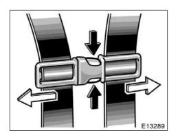
Compress the shoulder belt clip to separate the right and left shoulder belts.
