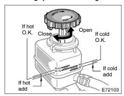
Check the fluid level through the reservoir. If necessary, add automatic transmission fluid DEXRON® II or III.
