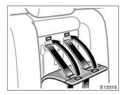
Press the removable pad against the fastener tapes and install the pad to the seatback. Make sure the belts go through the slots in the pad.
