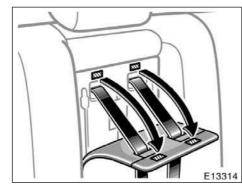
Pull down the seatback part of the removable pad. Make sure the child's shoulders are at or below the maximum shoulder height indicator label.
