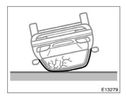
The SRS side airbags are not designed to inflate if the vehicle is rolled over.
