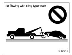
(c) Towing with sling type truck
