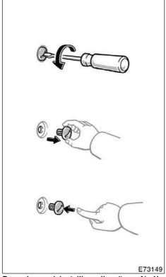
Removing and installing clips (type A): Use a flat-bladed screwdriver or equivalent.
