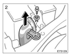
2. LEFT-HAND HEADLIGHT: Remove the clip and take out the air cleaner duct.
