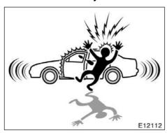
To deter the vehicle theft, the system is designed to give an alarm and keep the engine from being started if any of the doors, trunk or hood is forcibly unlocked or the battery terminal is disconnected and then reconnected when the vehicle is locked.
