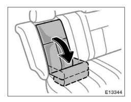
Separate the fastener tapes under the right rear seatback and fold the separated part of the seatback down while lowering it.
