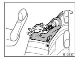
(B) CONVERTIBLE SEAT INSTALLATION A convertible seat is used in forward-facing and rear-facing position depending on the child's age and size. When installing, follow the manufacturer's instructions about the applicable child's age and size as well as directions for installing a child restraint system.
