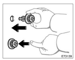
Installing clips (type B)
