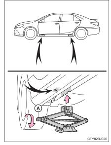
5 Raise the vehicle until the tire is slightly raised off the ground.
