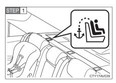
Secure the child restraint using the seat belt or LATCH anchors.
