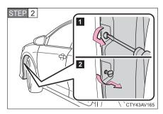
Remove the fender liner clip.
