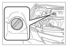
If the oil level is below or near the low level mark, add engine oil of the same type as that already in the engine.
