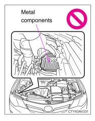
Vehicles with discharge headlights: While the low beam headlights are turned on, and for a short time after they have been turned off, metal components at the rear of the headlight assembly will be extremely hot. To prevent burns, do not touch these metal components until you are certain they have cooled down.
