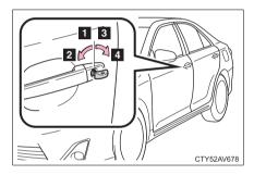
Using the mechanical key ( $\rightarrow$ P. 29) in order to perform the following operations (driver's door only):
