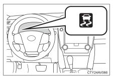
If the vehicle is in danger of slipping or if any of the drive wheels spins, the slip indicator light flashes to indicate that the TRAC/VSC systems are operating.
