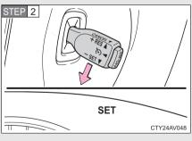
Accelerate or decelerate the vehicle to the desired speed, and push the lever down to set the speed.
