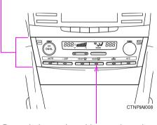
Rear window and outside rear view mirror defogger switch P. 199
