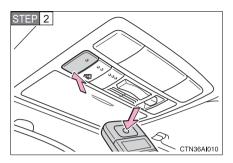
Press and hold down one of the buttons on HomeLink® and the button on the transmitter. When the indicator light on HomeLink® changes from a slow to a rapid flash after 20 seconds, you can release both buttons.
