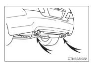
When your vehicle becomes stuck and cannot move, the emergency hooks are used for another vehicle to pull your vehicle out in an emergency.
