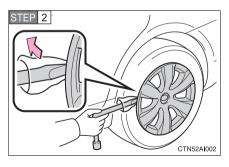
Vehicles with a steel wheel, remove the wheel ornament using the wrench.
