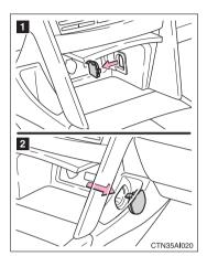
The auxiliary box of the front console is provided with a hole that allows cables to be passed into the cabin from the power outlet and AUX adapter inside.
