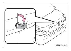
Turn the mechanical key clockwise to open.
