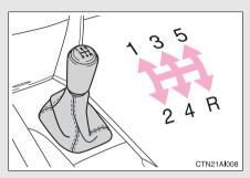
Fully depress the clutch pedal before operating the shift lever, and then release the clutch pedal slowly.
