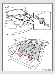
Pull the seatback lever in the trunk for the seatback you wish to fold down.
