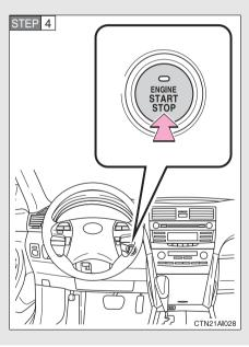
Press the "ENGINE START STOP" switch.
