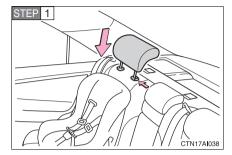
Secure the child restraint using the seat belt lower anchors, and lock the head restraint in place at the lowest position.
