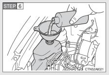
Add engine coolant if necessary.
