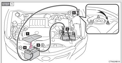
Connecting the jumper cables
