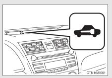
Vehicles with smart key system: The indicator light flashes after the "ENGINE START STOP" switch has been turned OFF to indicate that the system is operating.
