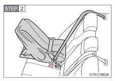
Run the seat belt through the child seat and insert the plate into the buckle. Make sure that the belt is not twisted.
