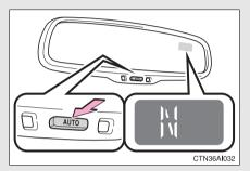
To turn the compass on or off, press and hold "AUTO" for 3 seconds.
