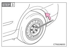
Slightly loosen the wheel nuts (one turn).
