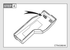
Remove the fuse with the pullout tool.
