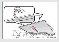
Pull the tab of the shade and hook it on using the anchors. To lower the shade, pull the tab slightly to unhook the shade, and lower it slowly.
