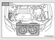
After the engine has cooled down sufficiently, check the engine coolant level and inspect the radiator core (radiator) for any leaks.
