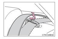
Use the seat belt after passing it through the guide if the seat belt comes free from the guide.
