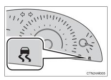
If the vehicle is in danger of slipping or the front wheels spin, the indicator flashes to indicate that VSC/TRAC have been engaged.
