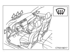
Pressing to turn the air conditioning on clears the windshield and side windows faster.
