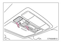
Press and hold down the 2 outside buttons for 20 seconds until the indicator light flashes.
