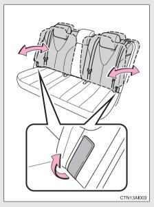
Pull up the seatback angle adjustment lever until the lock is completely released.
