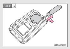
Remove the depleted battery.
