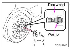
Turn the nuts until the washers come into contact with the disc wheel.
