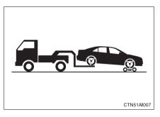
Automatic transmission: Use a towing dolly under the front wheels.
