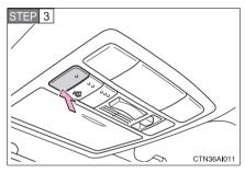
Test the operation of HomeLink<sup>®</sup> by pressing the newly programmed button.
