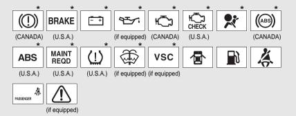
\*: These lights turn on when the "ENGINE START STOP" switch is turned to IGNITION ON mode (vehicles with smart key system) or the engine switch is turned to "ON" position (vehicles without smart key system) to indicate that a system check is being performed. They will turn off after the engine is started, or after a few seconds. There may be a malfunction in a system if a light does not come on, or if the lights do not turn off. Have the vehicle inspected by your Toyota dealer for details.
