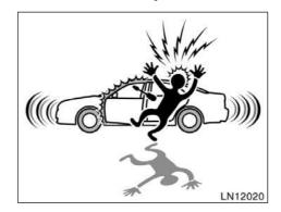
To deter vehicle theft, the system is designed to sound an alarm if any of the doors, trunk or hood is forcibly unlocked or the battery terminal is disconnected and then reconnected when the vehicle is locked.
