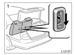
This system prevents someone (with the sub key) from gaining access to the trunk by folding down a rear seat or using the trunk lid lock release lever.
