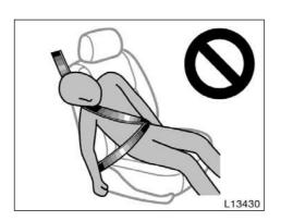
• Do not get your head closer to the area where the side airbag and curtain shield airbag inflate, since these airbags inflate with considerable speed and force. Otherwise, you may be killed or seriously injured. Special care should be taken especially when you have a small child in the vehicle.
