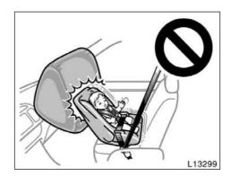
Never install a rear-facing child restraint system on the front passenger seat because the force of the rapid inflation of the front passenger airbag can cause death or serious injury to the child.
