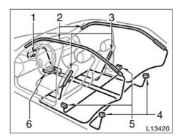
The SRS side airbag and curtain shield airbag system mainly consists of the following components, and their locations are shown in the illustration.
