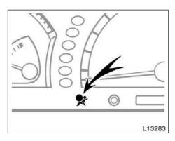
This front seat belt pretensioner system has a service reminder indicator to inform the driver of operating problems. If any of the following conditions occurs, this indicates a malfunction of the airbags or pretensioners. Contact your Toyota dealer as soon as possible to service the vehicle.
