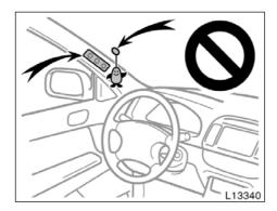
• Do not attach a microphone or any other device or object around the part where the curtain shield airbag activates such as on the windshield glass, side door glass, front and rear pillars, roof side and assist grips. When the curtain shield airbag inflates, the microphone or other device or object will be thrown with great force or the curtain shield airbag may not activate correctly, resulting in death or serious injury.
