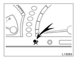
This SRS side airbag and curtain shield airbag system has a service reminder indicator to inform the driver of operating problems. If either of the following conditions occurs, this indicates a malfunction of the airbags. Contact your Toyota dealer as soon as possible to service the vehicle.
