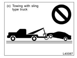
(c) Towing with sling type truck
