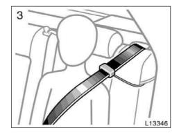
Buckle, position and release the seat belt. (For wearing the seat belt, see "—Front and rear seat belts" on page 46 in this section.) Make sure the shoulder belt crosses the shoulder.
