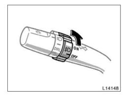
To turn on the front fog lights, twist the band of the headlight and turn signal switch lever. They will come on only when the headlights are on low beam.
