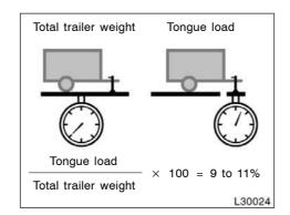
● The trailer cargo load should be distributed so that the tongue load is 9 to 11% of the total trailer weight, not exceeding the maximum of 90 kg (200 lb.). Never load the trailer with more weight in the back than in the front. About 60% of the trailer load should be in the front half of the trailer and the remaining 40% in the rear.
