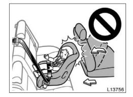
• A forward-facing child restraint system should be allowed to be installed on the front passenger seat only when it is unavoidable. Always move the seat as far back as possible, because the force of the deploying front passenger airbag could cause death or serious injury to the child.
