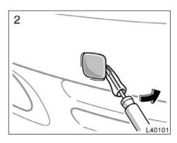
Remove the front towing eyelet cover on the front bumper, using a flatbladed screwdriver which is wrapped with a cloth.
