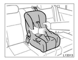
Push and pull the child restraint system in different directions to be sure it is secure. Follow all the installation instructions provided by its manufacturer.
