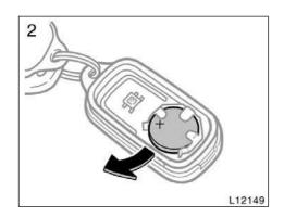
2. Remove the discharged transmitter battery.
