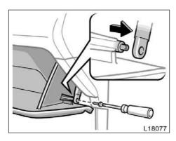
Open the glove box. Remove the screw with a Phillips-head screwdriver and slide the hook as shown.
