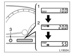
This meter displays the odometer and two trip meters when the ignition switch is on.
