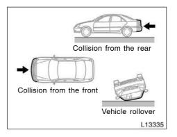
The SRS side airbags and curtain shield airbags are not designed to inflate if the vehicle is involved in a front or rear collision, if it rolls over, or if it is involved in a low-speed side collision.
