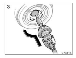
Plug in a new bulb into the connector and install it into the mounting hole.
