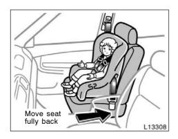
On vehicles with side airbags and curtain shield airbags, do not allow the child to lean against the door or around the door even if the child is seated in the child restraint system. It is dangerous if the side airbag and curtain shield airbag inflate, and the impact could cause death or serious injury to the child.
