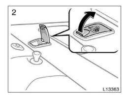
2. Open the lid of the anchor bracket to open.
