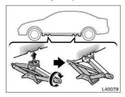
Position the jack at the correct jack point as shown. Rotate the load rest 90° from storage position to lifting position.
