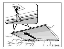
To raise the rear sun shade, pull the tab of the shade and hook it on the anchors. To lower the shade, pull the tab slightly to unhook the shade, and lower it slowly.
