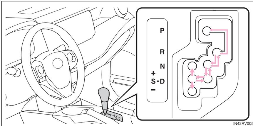
← While the power switch is in ON mode, move the shift lever with the brake pedal depressed.
