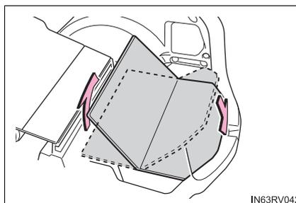
4 Lay the opposite side of the deck board over the edge of the separator.
