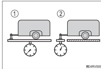
The gross trailer weight, gross axle weight and tongue weight can be measured with platform scales found at a highway weighing station, building supply company, trucking company, junk yard, etc.
