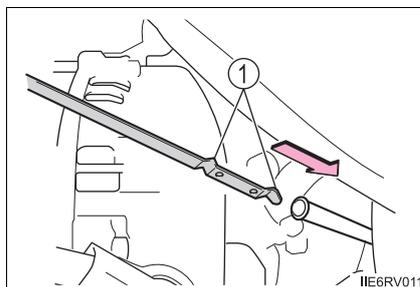
5 Holding a rag under the end, pull the dipstick out and check the oil level.
