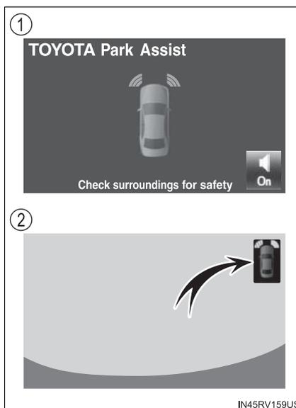
**Sensor detection display, obstacle distance**
