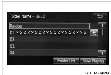
Turn the “TUNE•SCROLL” knob to move the cursor box to select a desired item from the list, and press the knob to play it. The track that is being played is highlighted.
