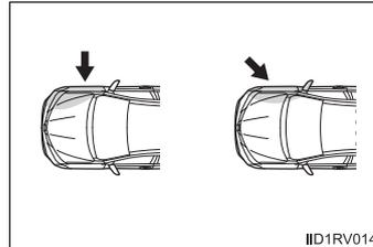
The SRS side airbags do not generally inflate if the vehicle is involved in a rear collision, if it rolls over, or if it is involved in a low-speed side or low-speed frontal collision.
