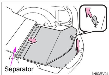
3 Lift the opposite side of the deck board up and return the nearest side to its original position.
