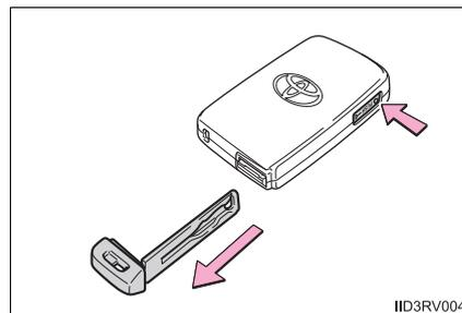
After using the mechanical key, store it in the electronic key. Carry the mechanical key together with the electronic key. If the electronic key battery is depleted or the entry function does not operate properly, you will need the mechanical key. (→P. 590)
