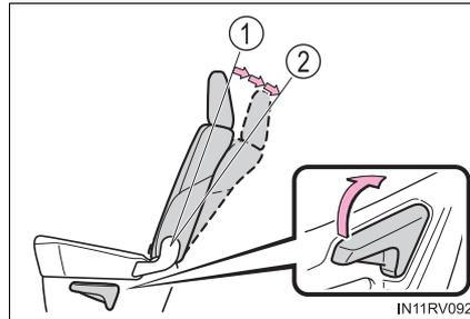
If your child restraint system interferes with a head restraint and cannot be installed properly, install the child restraint system after removing the head restraint. (→P. 151)
