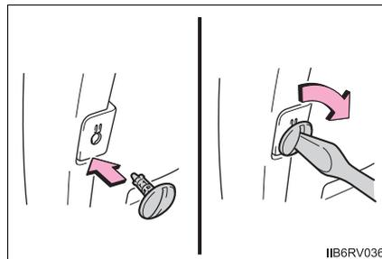
**9** Reinstall the fender liner and install the screws.
