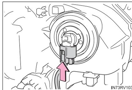
■ **Front turn signal lights/parking lights (halogen headlights) or front turn signal lights (LED headlights)**
