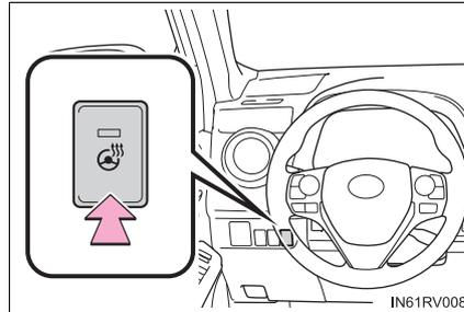
The heated steering wheel can be used when the power switch is in ON mode.
