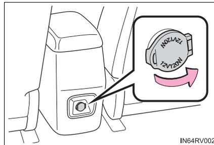
The power outlets can be used when the power switch is in ACCESSORY or ON mode.
