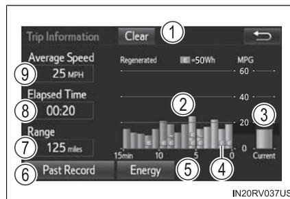
Average fuel consumption for the past 15 minutes is divided by color into past averages and averages attained since the power switch was last turned to ON mode. Use the displayed average fuel consumption as a reference.
