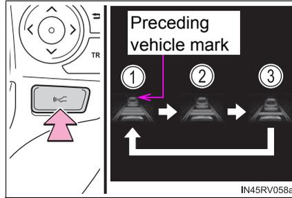
**Vehicle-to-vehicle distance settings (vehicle-to-vehicle distance control mode)**
