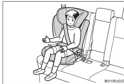
Check that the shoulder belt is correctly positioned over the child's shoulder and that the lap belt is as low as possible. (→P. 30)
